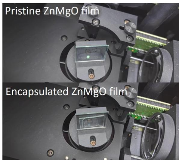
Figure. S3 photos of pristine and encapsulated ZnMgO films excited by 330 nm Xe lamp
