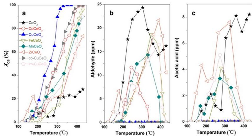
**Figure S5** CB conversion and primary reaction byproduct distribution over synthesized catalysts.
