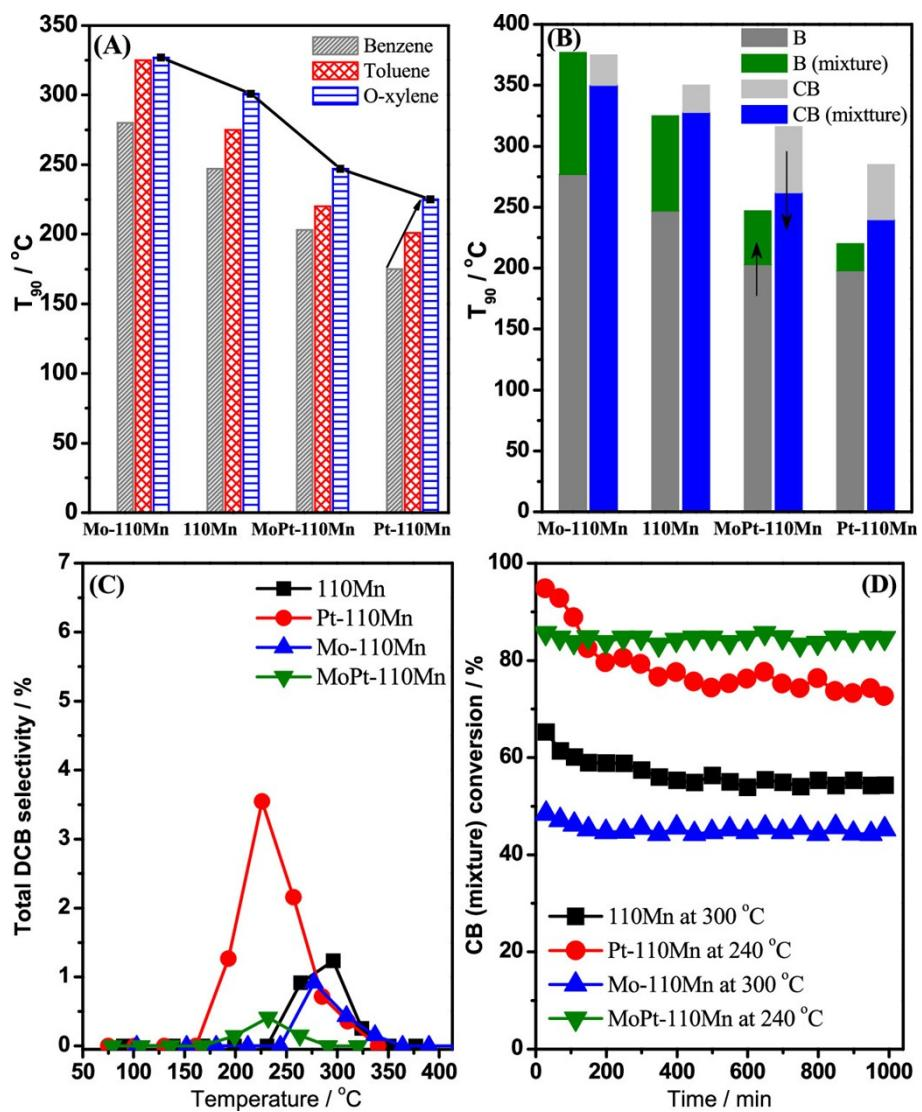
**Figure S3** Catalytic performance of prepared Mn-based catalysts for catalytic oxidation of BTX (A) and the mixed CB and benzene (B), DCB selectivity (C), and durability (D) for catalytic oxidation of the mixed CB and benzene.<sup>37</sup> Copyright 2021 American Chemical Society
