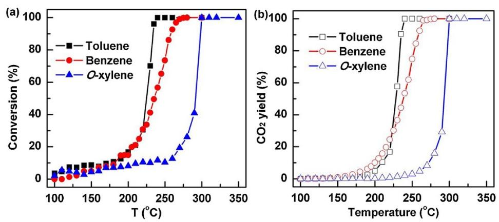
**Figure S1.** The activity test in catalytic oxidation of VOCs at: Conversion of different aromatic VOCs and CO<sub>2</sub> yield over 3Mn1Ce. (WHSV of 60000 mL g<sup>-1</sup> h<sup>-1</sup>) <sup>35</sup> Copyright 2018 American Chemical Society
