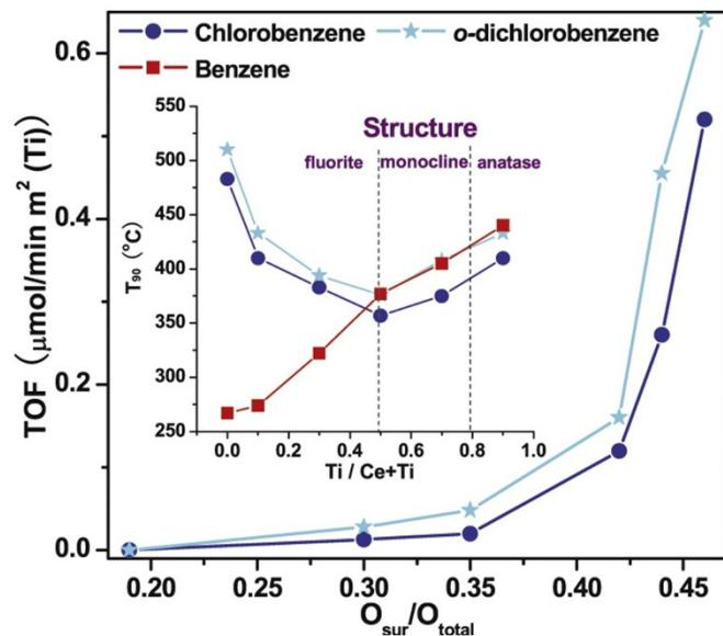
**Figure S6** Effect of structure on CBCs removal performance on Ce-Ti mixed oxide catalysts.<sup>40</sup>
