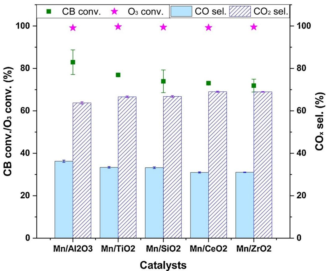
**Figure S2** Catalytic performance of CB ozonation over MnO<sub>x</sub> with different supports.<sup>36</sup>
