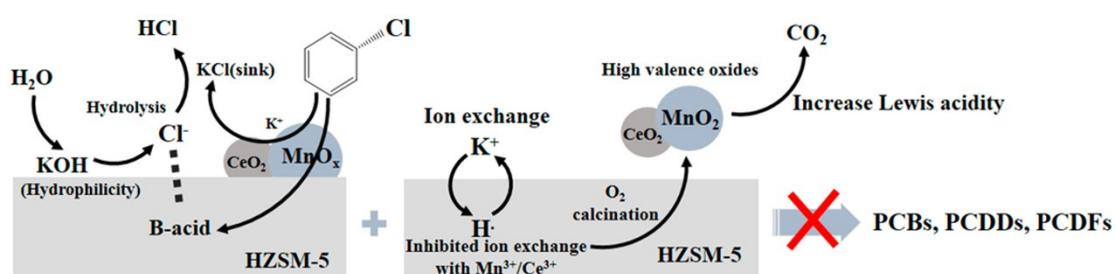
**Figure S4** Possible reaction mechanism of CB oxidation on  $\text{Mn}_x\text{Ce}_{1-x}\text{O}_2/\text{HZSM-5}$ .<sup>38</sup> Copyright 2018 American Chemical Society
