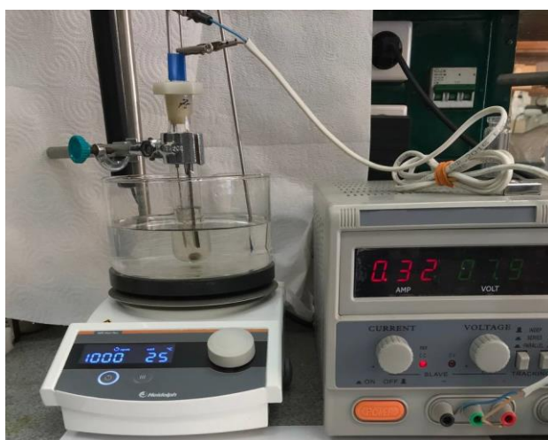
Figure S2. Undivided electrochemical cell equipped with glassy carbon anode (4.5 cm 2 ) and platinum plate cathode (4.5 cm 2 ) and connected to a DC regulated power supply with the reaction mixture during electrolysis under constant current conditions.
