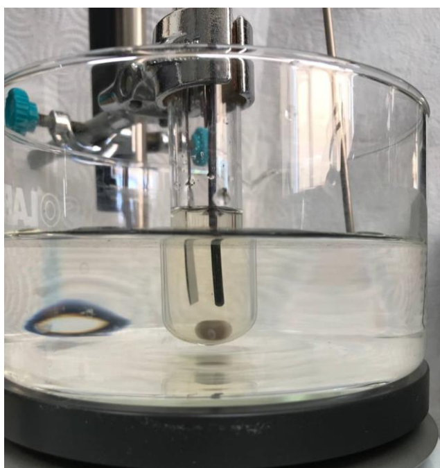
Figure S3. Undivided electrochemical cell equipped with glassy carbon anode (4.5 cm 2 ) and platinum plate cathode (4.5 cm 2 ) with the reaction mixture at the beginning of the reaction.
