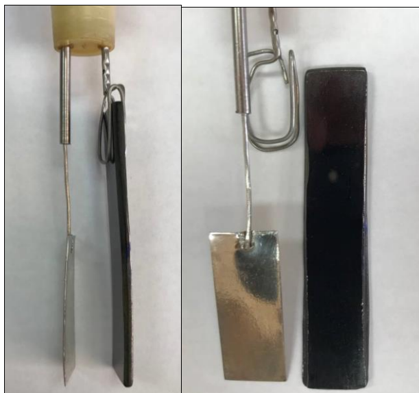
Figure S1. Glassy carbon anode (4.5 cm 2 ) and platinum plate cathode (4.5 cm 2 )
