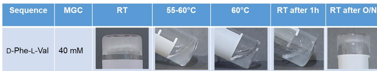
Fig. S20. Thermoreversibility test for D-Phe-L-Val hydrogel
