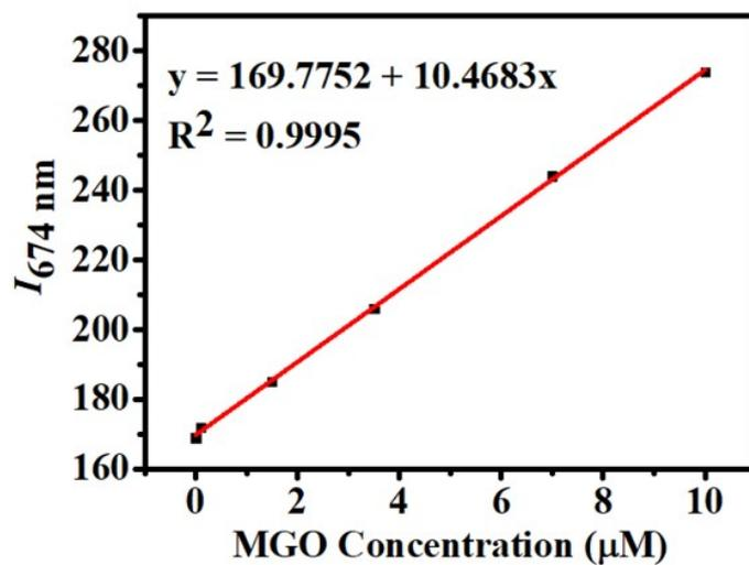
**Fig. S9.** Linear relationship between the fluorescence intensity at 674 nm and MGO concentration from 0.0 to 10.0 μM.
