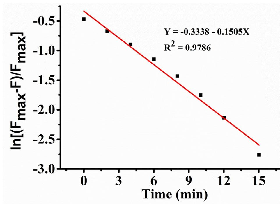
**Fig. S10.** Pseudo first-order kinetic plots of SWJT-2 (10.0  $\mu\text{M}$ ) with the addition of MGO. ( $\lambda_{\text{ex}} = 450 \text{ nm}$ )
