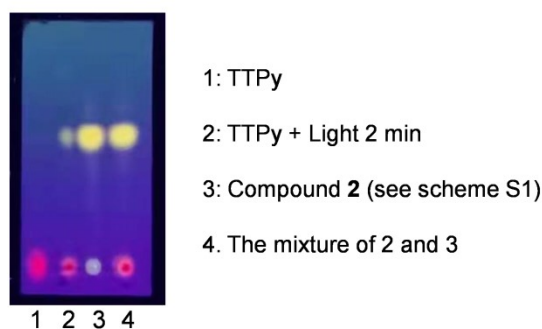
Fig. S14. Thin layer chromatography (TLC) analysis of the photochemical product of TTPy. TTPy in 0.1% SDS solution was irradiated by a LED light (490 nm, 5W) for 2 min. The eluent is ethyl acetate/petroleum ether 1:5.
