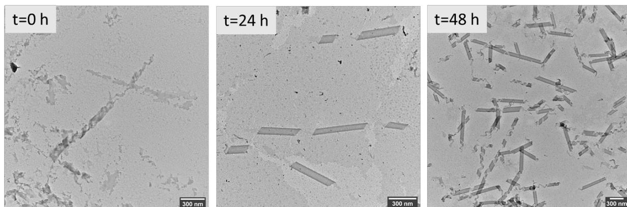
**Figure S16:** TEM images of **1** during the assembly process. Samples were aged for 72 h at 20 mM in PBS (pH 7.4). Aliquots were removed for imaging at various time points after dissolution in PBS. Samples were diluted to 1 mM prior to imaging.
