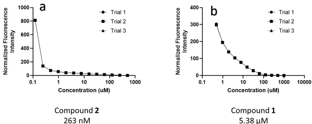
**Figure S14:** CAC plots for the determination of the CAC for compound 2 (a) and 1 (b) using CPT fluorescence. Samples of both 1 and 2 were aged at 10 mM in PBS (pH 7.4) for 72 h before dilution to concentrations for analysis. The CAC of compound 1 was found to be  $5.38 \pm 0.01 \mu\text{M}$ . The CAC of compound 2 was found to be 263 nM.
