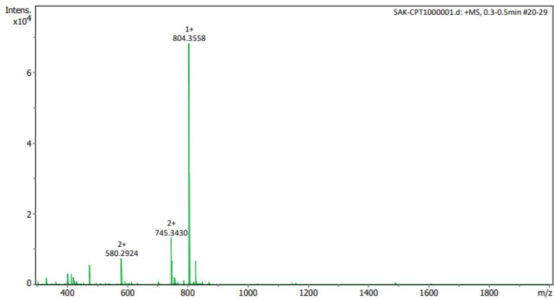
**Figure S8:** ESI High-resolution mass spectrum of **2**, obtained in positive mode with 80/20 MeCN/water.
