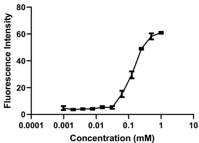
**Figure S15:** CMC plot for compound 1 using Nile red (50  $\mu\text{L}$  of 20  $\mu\text{M}$  Nile Red in acetone was added to each sample) as a fluorescent probe. Compound 1 was aged at 10 mM in PBS (pH 7.4) for 72 h before dilution to concentrations for analysis. The CMC of compound 1 was found to be  $38 \pm 3 \mu\text{M}$ .
