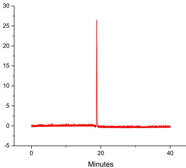
**Figure S2.** Analytical HPLC trace (1 mL/min, ramped from 15-80% CH<sub>3</sub>CN in water, spiked with 0.1% TFA) of **2** after purification via preparatory HPLC.
