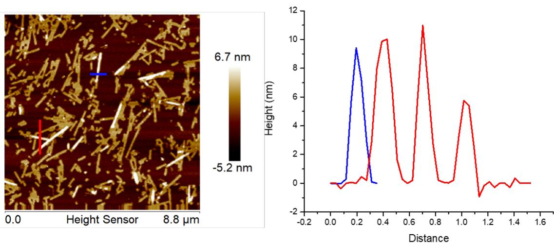
**Figure S18:** AFM image of compound **1** Samples were aged for 72 h at 20 mM in PBS (pH 7.4), then diluted to 1.0 mM and deposited onto freshly cleaved mica for 5 min, rinsed with water for 10 s, then dried with nitrogen gas. Images were analyzed with Bruker’s software. Cross-sectional information was gathered using Bruker’s software and plotted with origin.
