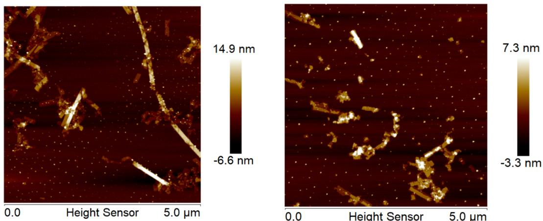
**Figure S21:** AFM images of drug release from compound **1**. Samples were aged for 72 h at 10 mM in PBS (pH 7.4), then diluted to 1.0 mM and heated to 37°C for 48 h. Samples (1.0 mM) were deposited onto freshly cleaved mica for 5 min, rinsed with water for 10 s, then dried with nitrogen gas. Images were analyzed with Bruker's software.
