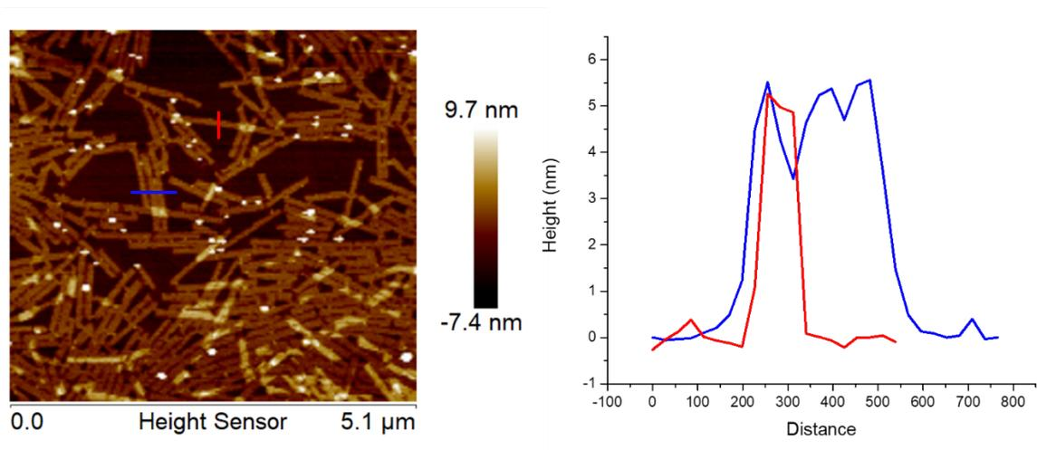
**Figure S19:** AFM image of compound **2**. Samples were aged for 72 h at 10 mM in PBS (pH 7.4), then diluted to 1.0 mM and deposited onto freshly cleaved mica for 5 min, rinsed with water for 10 s, then dried with nitrogen gas. Images were analyzed with Bruker software. Cross-sectional information was gathered using Bruker’s software and plotted with origin.
