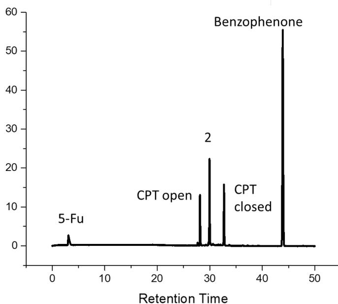
**Figure S23:** HPLC trace of **1**, assembled in PBS (pH 7.4) for 72 h at 10 mM, then diluted to 0.1 mM and heated to 37°C for 96 h to induce partial release of 5-FU and CPT. Trace plotted was measured at 254 nm, and all peaks were verified by co-injection of the individual components.
