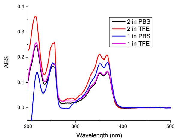
**Figure S11:** UV-Vis absorption spectra of peptides **1** and **2** in PBS and TFE. Each sample was aged in TFE or PBS at 10 mM for 72 h, then were diluted to 0.1 mM to record the spectra.
