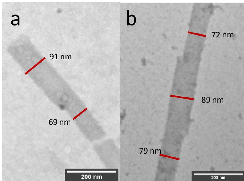
**Figure S20:** TEM images of **1**, assembled in PBS (pH 7.4) for 72 h at 10 mM, then diluted to 0.1 mM and heated to 37°C for (a) 24 h and (b) 72 h to induce drug release. Image shows regions of the nanotube with smaller diameters, consistent with hydrolytic release of 5-FU and the formation of smaller nanotubes from **2**.
