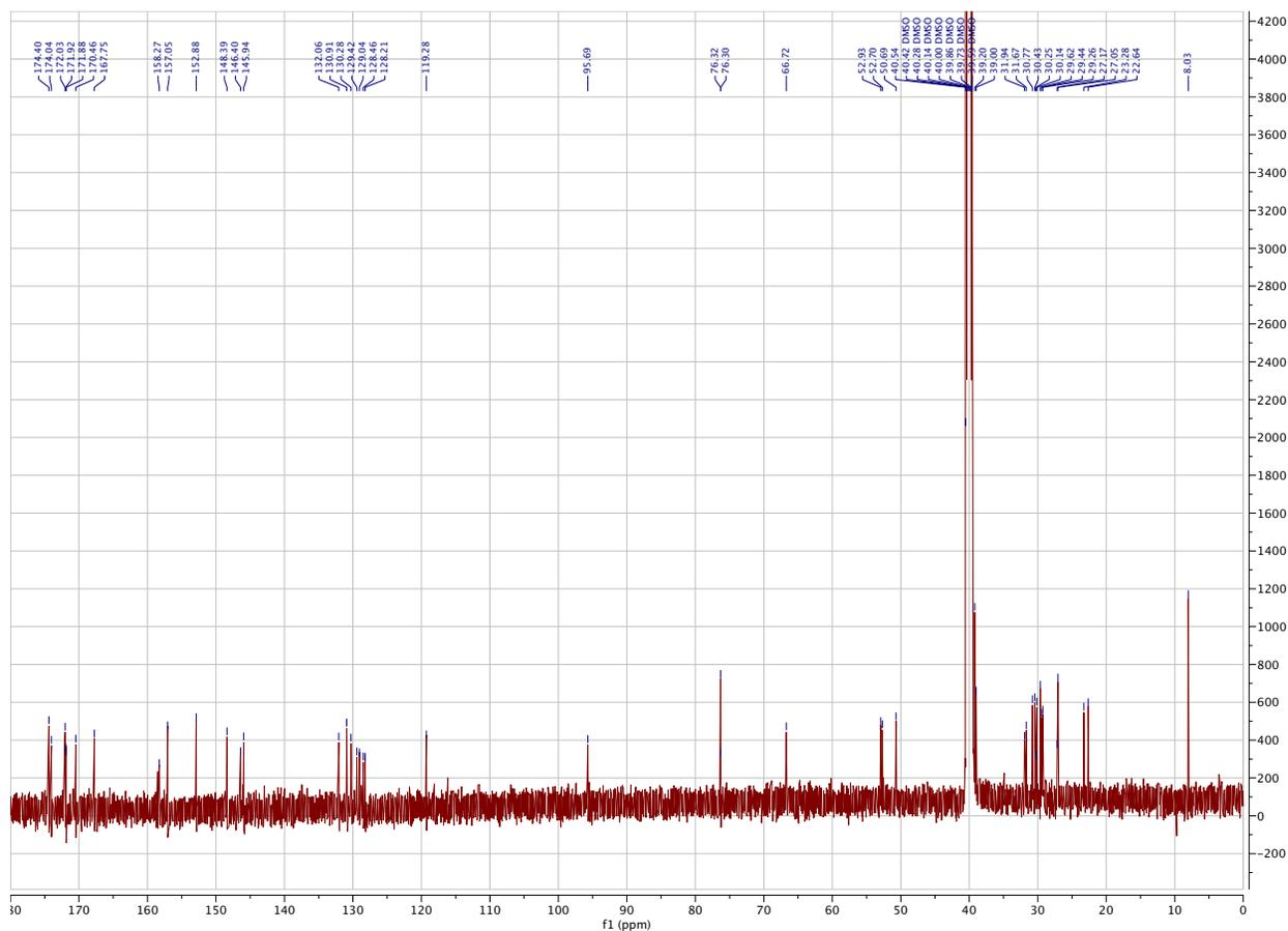
**Figure S7:**  $^{13}\text{C}$ -NMR spectra of **2** in  $\text{DMSO-d}_6$ . Significant aggregation at the concentration needed for  $^{13}\text{C}$  NMR produced additional peaks in the spectrum.
