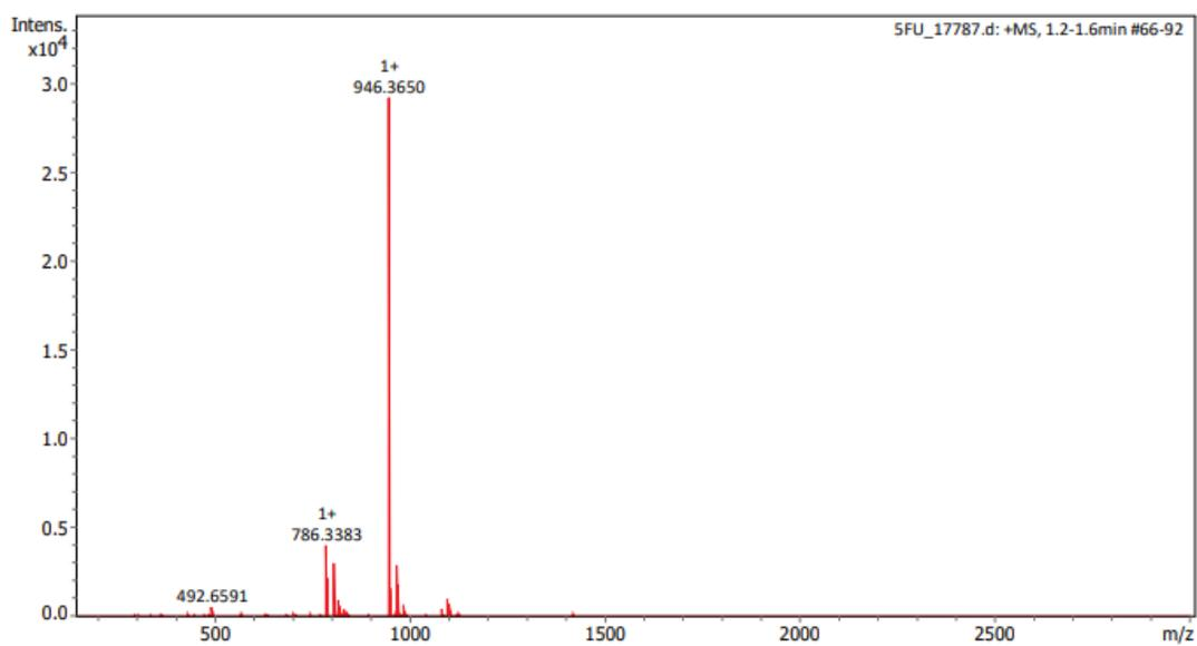
**Figure S5:** ESI High-resolution mass spectrum of **1**, obtained in positive mode with 80/20 MeCN/water.
