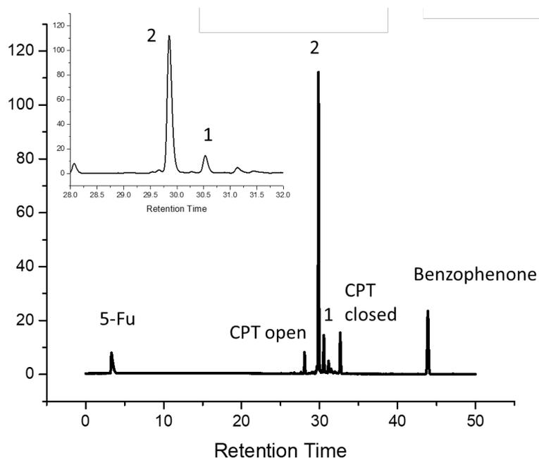
**Figure S22:** HPLC trace of **1**, assembled in PBS (pH 7.4) for 72 h at 10 mM, then diluted to 1 mM and heated to 37°C for 48 h to induce partial release of 5Fu. Trace plotted was measured at 254 nm, and all peaks were verified by co-injection of the individual components.
