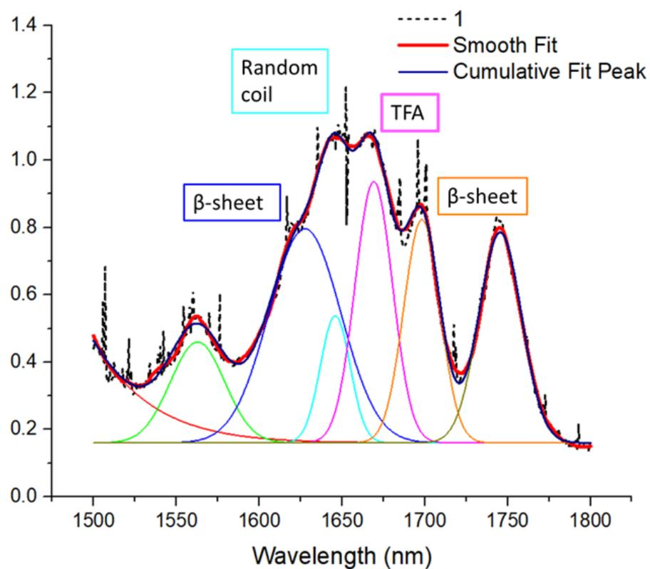
**Figure S12:** Deconvoluted FT-IR spectrum of **1** in (PBS, D<sub>2</sub>O). Sample was prepared by assembling at 20 mM in PBS for 72 h followed by two cycles of lyophilization and resuspension in D<sub>2</sub>O. The deconvoluted spectrum indicates the presence of  $\beta$  sheet and random coil (~86%  $\beta$  character and 14% random coil).
