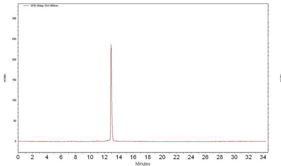
**Figure S1.** Analytical HPLC trace (1 mL/min, ramped from 10-70% CH<sub>3</sub>CN in water with 0.1 %TFA) of **1** after purification via preparatory HPLC.
