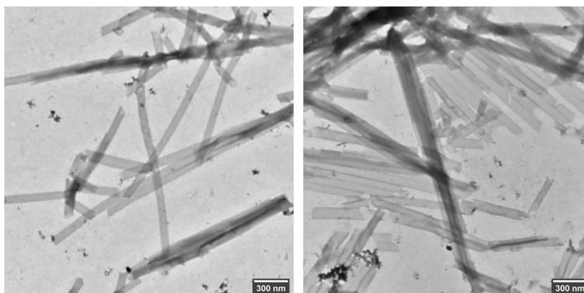
**Figure S17:** TEM images of **2** after assembling in PBS at 10 mM for 72 h. Samples were diluted to 1 mM prior to imaging.
