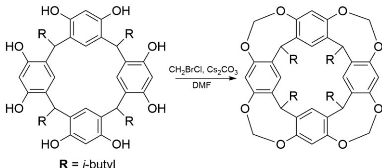
Resorcin[4]arene **O-RA** was obtained accordingly literature procedure.<sup>4</sup>
