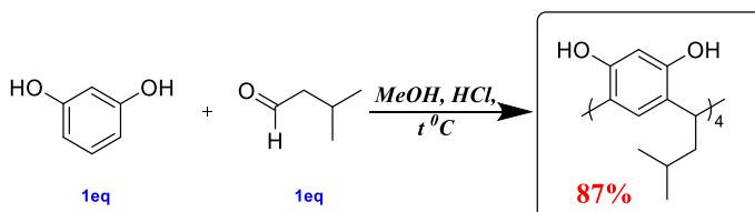
Resorcin[4]arene **H-RA** was obtained by acid-catalyzed condensation of resorcinol with isovaleraldehyde in a simple one-pot reaction by the literature procedure.<sup>1</sup>
