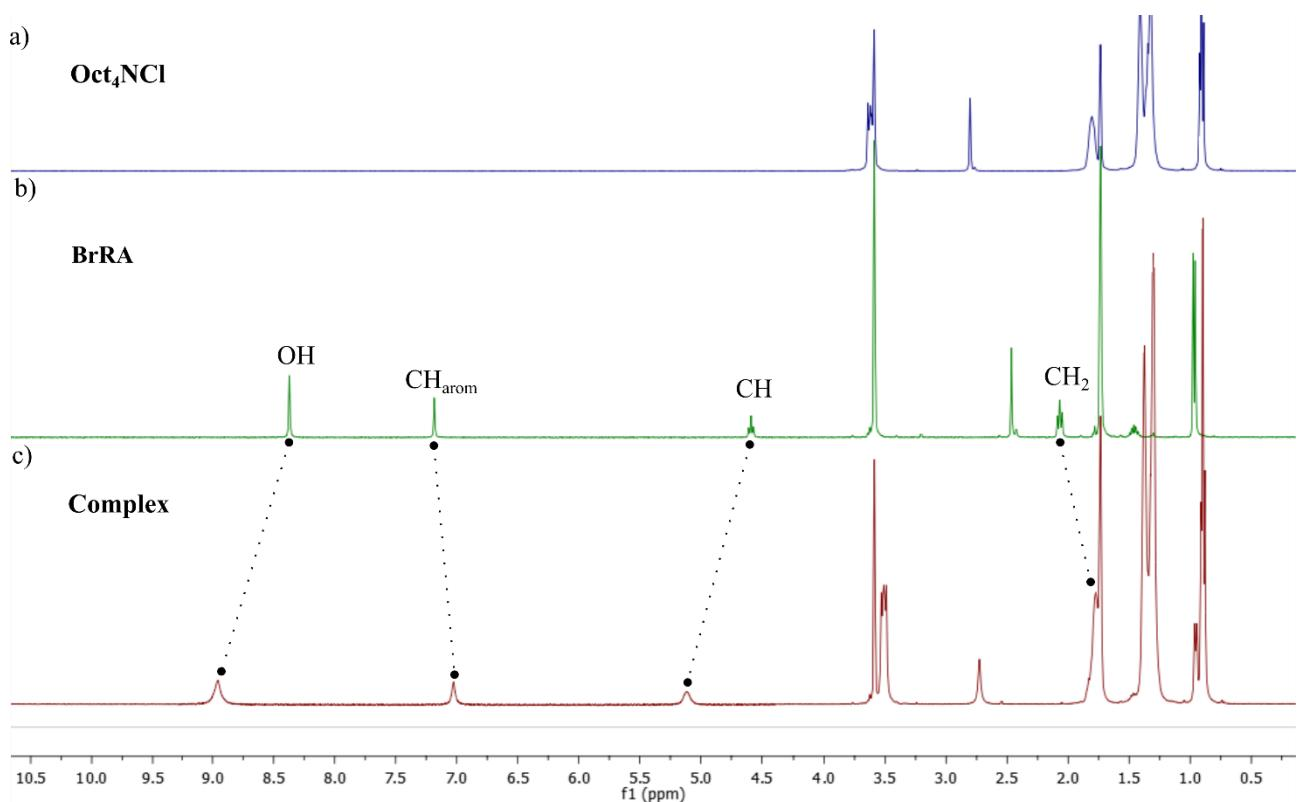
**Figure S4.** <sup>1</sup>H NMR spectra of (a) Oct<sub>4</sub>NCl; (b) Br-RA; (c) complex of Br-RA and Oct<sub>4</sub>NCl (400 MHz, 303 K, THF-d8).
