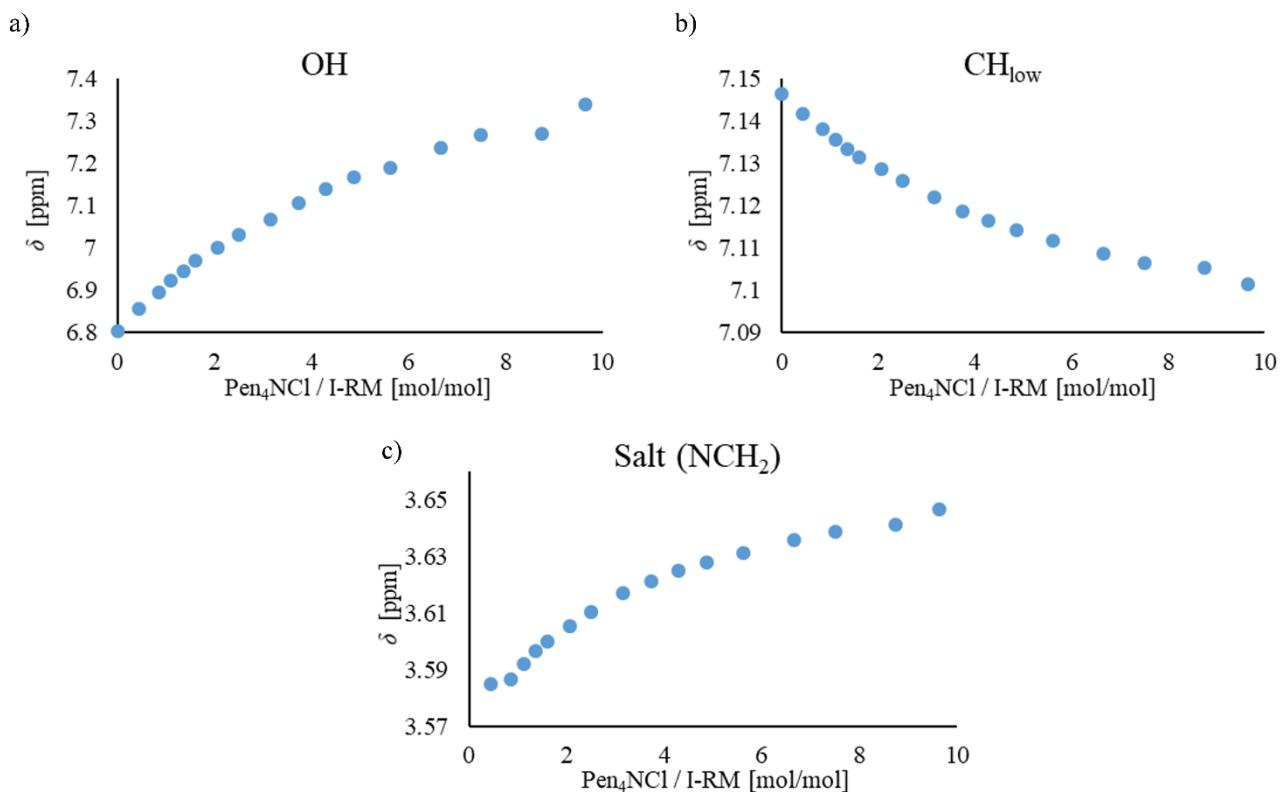
**Figure S3.** <sup>1</sup>H NMR titration curves for titration of I-RM with Pen<sub>4</sub>NCl. <sup>1</sup>H NMR chemical shifts change for: (a) OH; (b) CH<sub>low</sub>; (c) NCH<sub>2</sub> from salt (400 MHz, 303 K, THF-d8).
