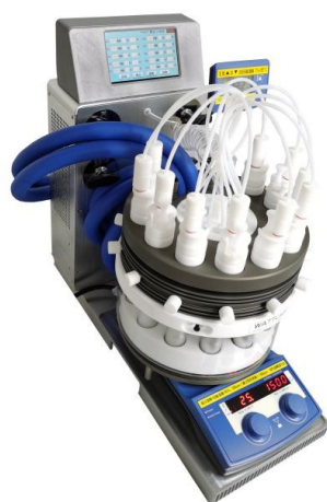
Figure. S1 The WP-TEC-1020HSL photochemical reaction system with the blue light LED
