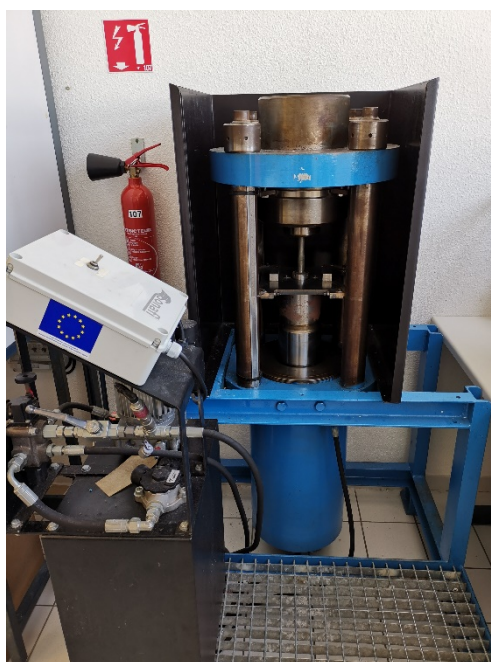
Figure 2. Piston-cylinder type apparatus Ollivaud/Lebas, France.
