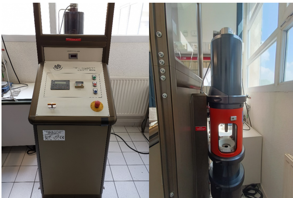
Figure 1. Pictures of piston-cylinder type apparatus U16 (Unipress, Warsaw, Poland): front (left) and side (right)
