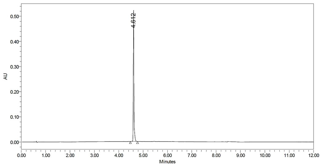
**Figure S6:** Purity Check by HPLC data for  $[\text{Cu}(\text{PyS3})_2]$
