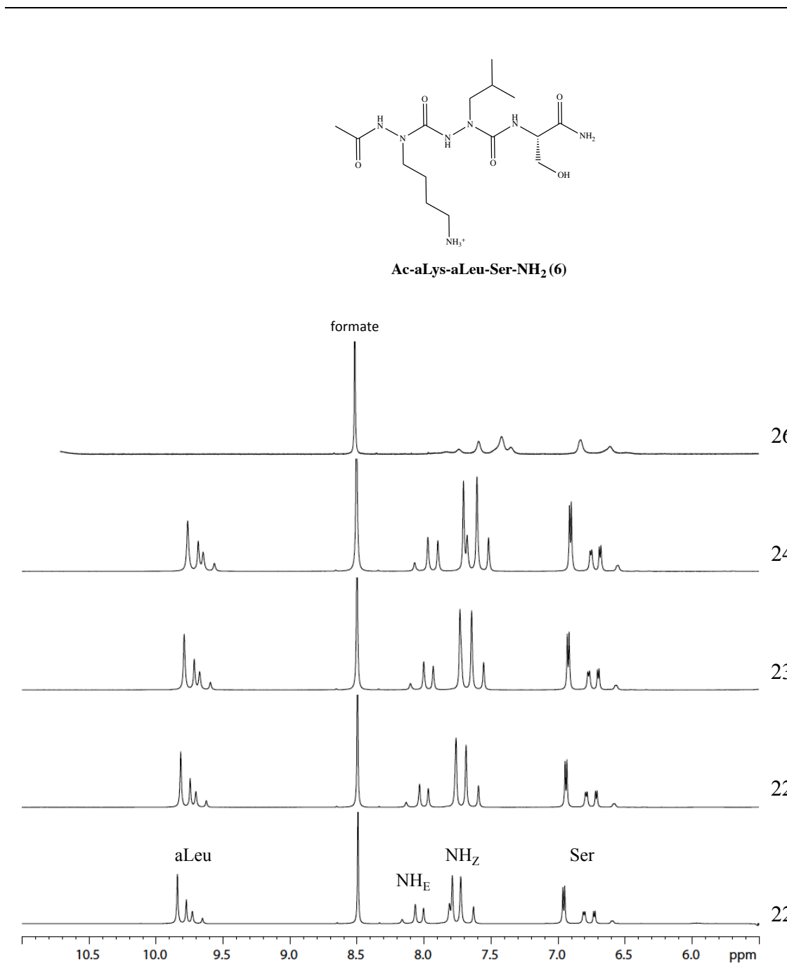
Figure S24: Variation of the amide NH proton chemical shifts of 6 in methanol (25.6 mM) in the temperature range 222 K–262 K (600.4 MHz)
