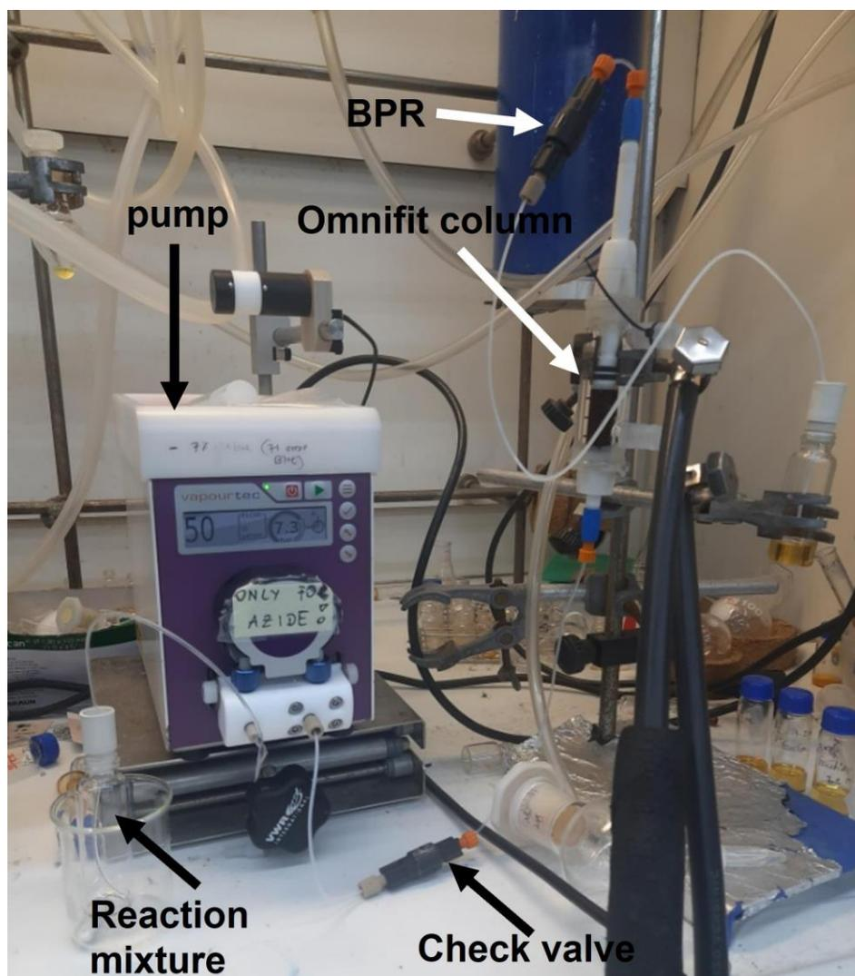
**Figure S3.** Continuous flow setup for conjugate addition using supported catalyst
