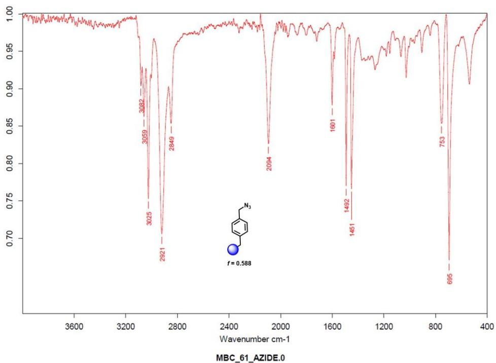
**Figure S1.** IR spectra of azidomethylpolystyrene (Azide peak at 2094 cm<sup>-1</sup>).
