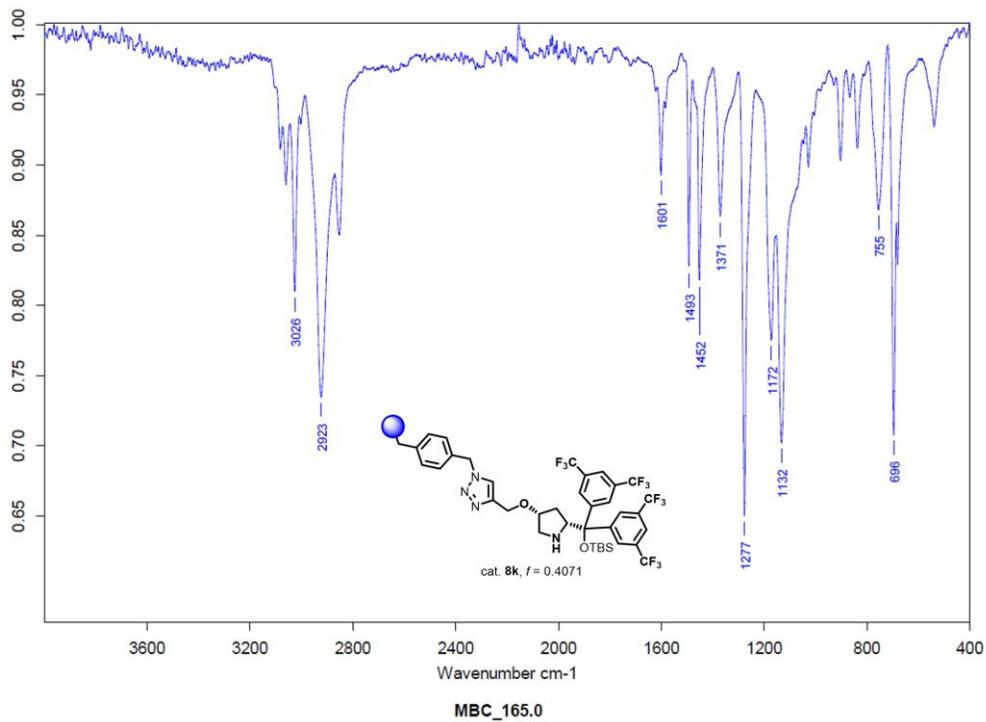
**Figure S2.** IR spectra of catalyst **8k** shows absence of azide peak at 2094 cm<sup>-1</sup>
