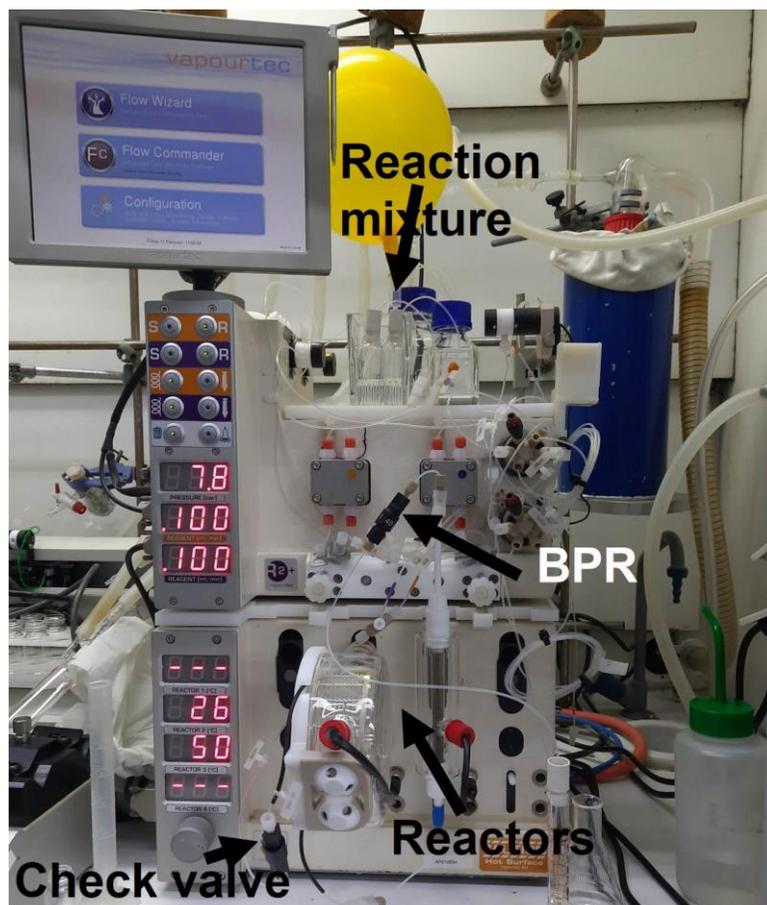
Figure S6. Reaction setup for synthesis of lactone using continuous flow
