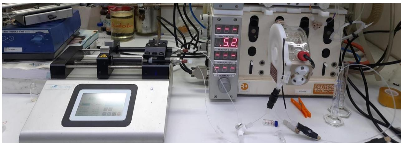
**Figure S4. Reaction setup for the continuous-flow synthesis of indoloquinolizidines 1**
