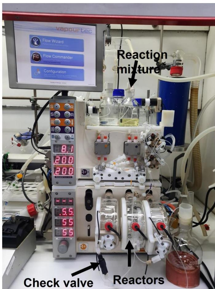
**Figure S5. Reaction setup for the scale-up of the continuous-flow synthesis of indoloquinolizidines 1**
