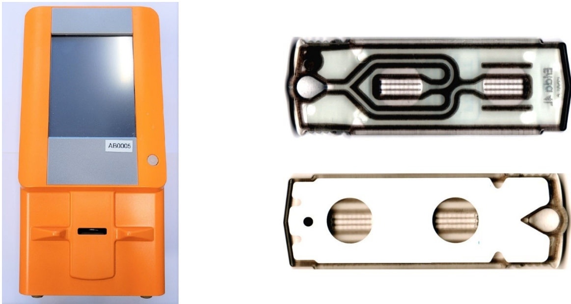
Figure S23. Optical reader system (400 nm) and polymer cartridge (top and bottom view)
