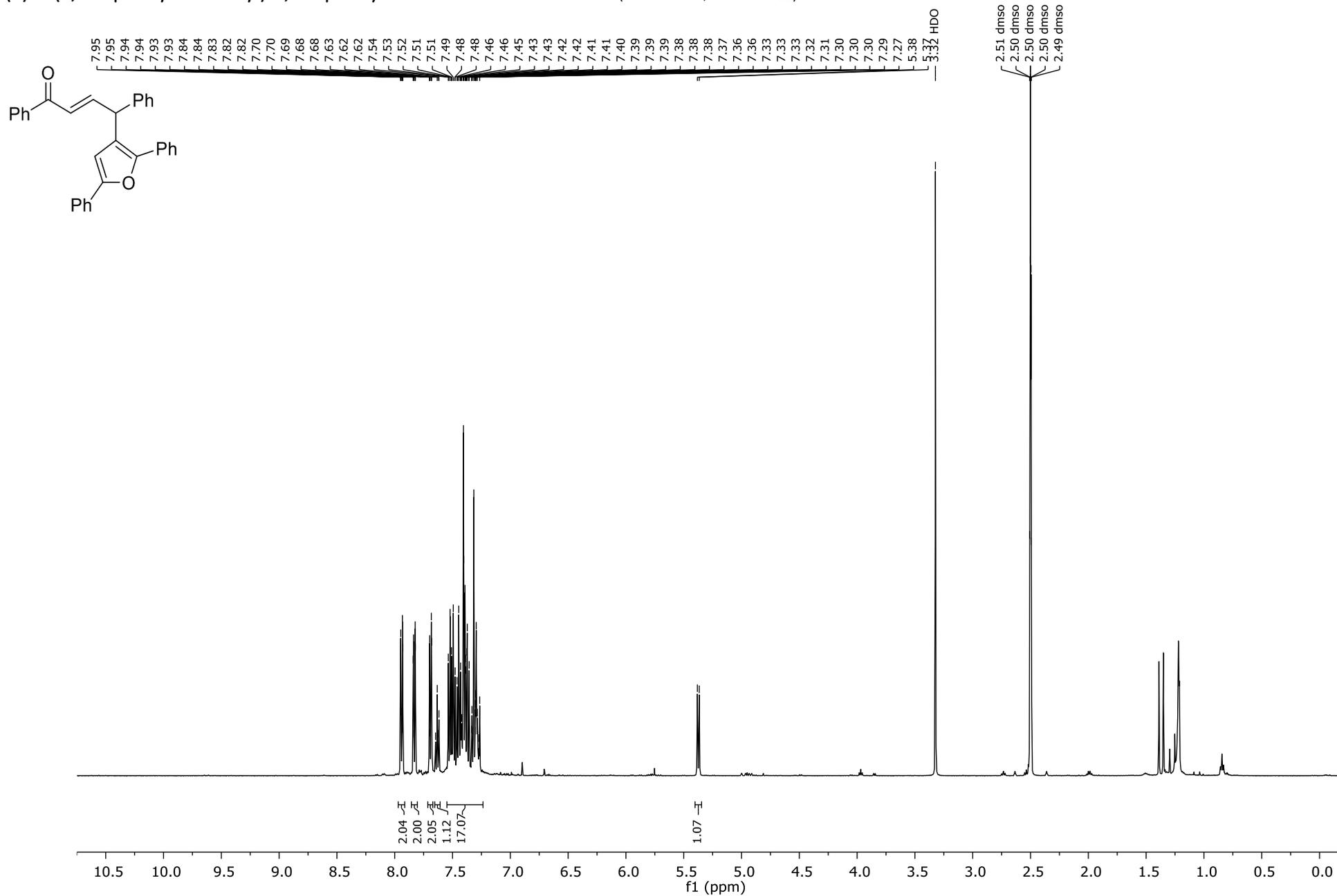
(E)-4-(2,5-Diphenylfuran-3-yl)-1,4-diphenylbut-2-en-1-one <sup>1</sup>H NMR (126 MHz, DMSO-*d*<sub>6</sub>)
