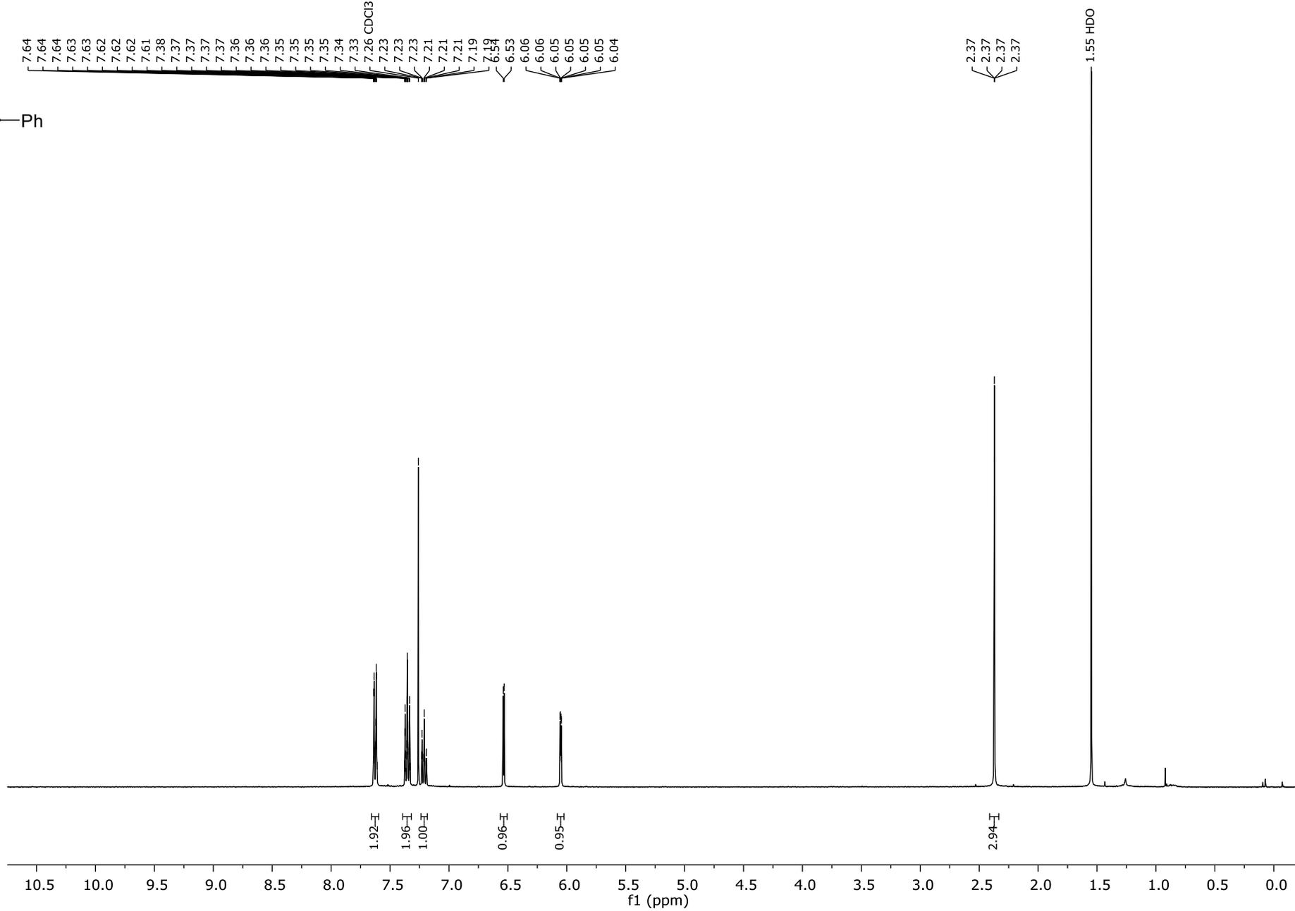
2-Phenylfuran 17 <sup>1</sup>H NMR (400 MHz, CDCl<sub>3</sub>)
