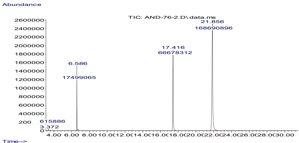
**Figure S121.** Chromatogram of the reaction mixture after reaction of 2-methylbenzene-1,3-diamine **7** with 4 equiv. EDA in the presence of 0.05 mol. % **1 $\beta$** .
