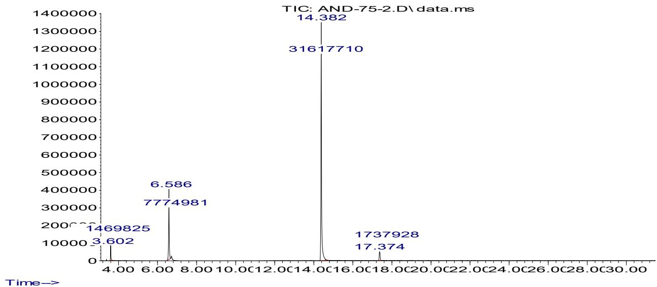
**Figure S117.** Chromatogram of the reaction mixture after reaction of 2-methylbenzene-1,3-diamine 7 with 4 equiv. EDA in the presence of 0.15 mol. % **1a**.
