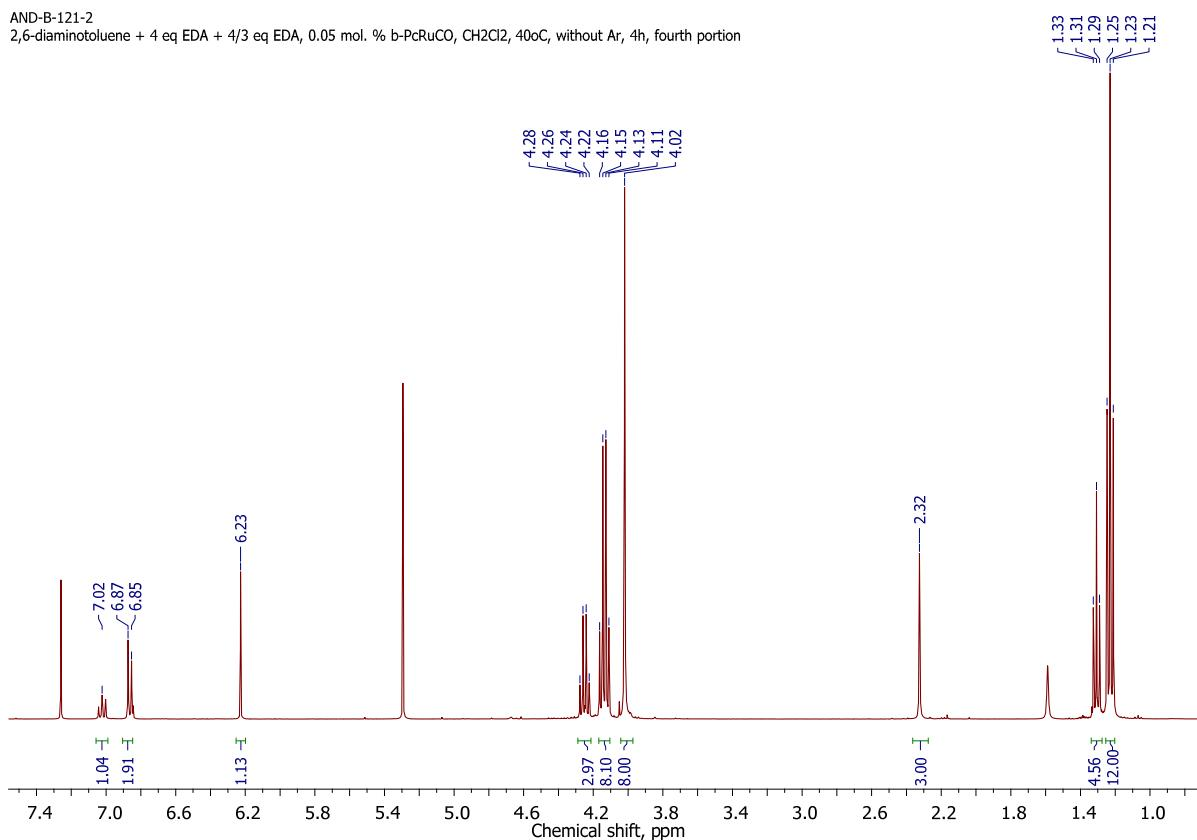
**Figure S120.** <sup>1</sup>H NMR spectrum of the reaction mixture after reaction of 2-methylbenzene-1,3-diamine **7** with 4 equiv. EDA in the presence of 0.05 mol. % **1 $\beta$** .
