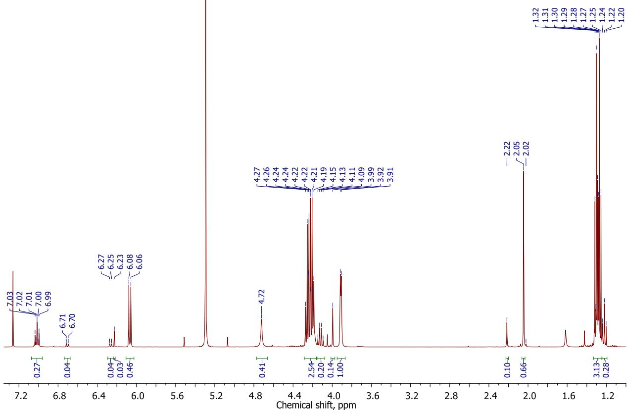
**Figure S116.** <sup>1</sup>H NMR spectrum of the reaction mixture after reaction of 4 equiv. EDA with 2-methylbenzene-1,3-diamine 7 in the presence of 0.15 mol. % **1a**.
