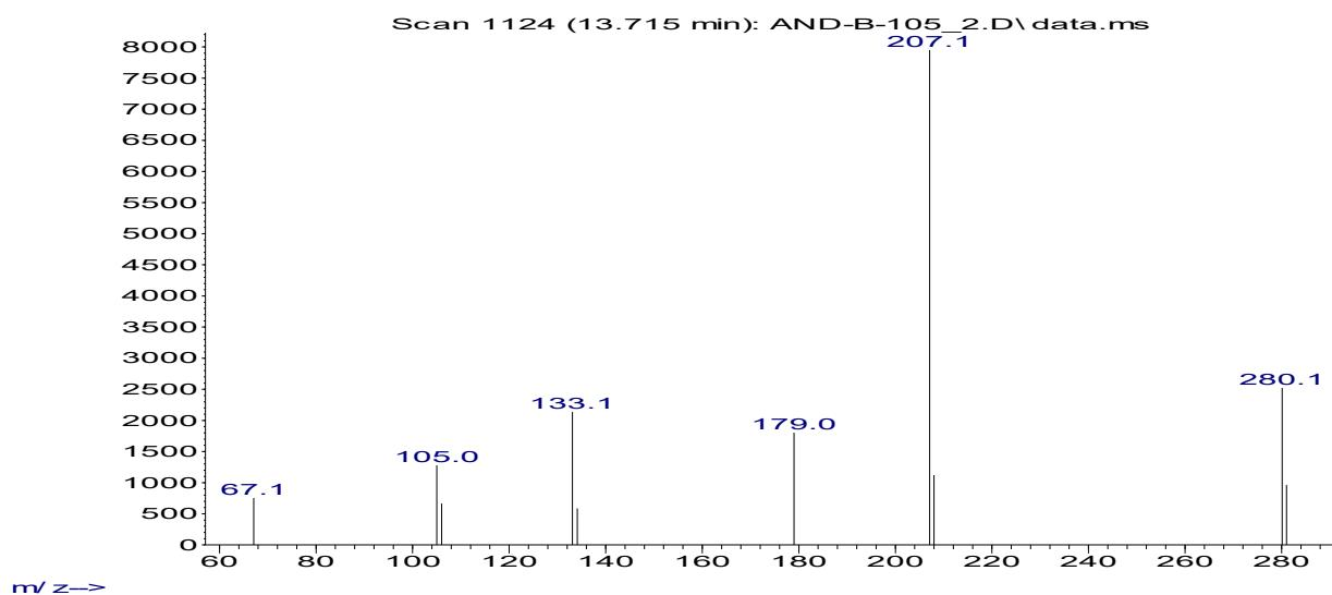
**Figure S93.** Mass spectrum (EI) of diethyl 2,2'-(1,4-phenylenebis(azanediyl))diacetate **5ss**.
