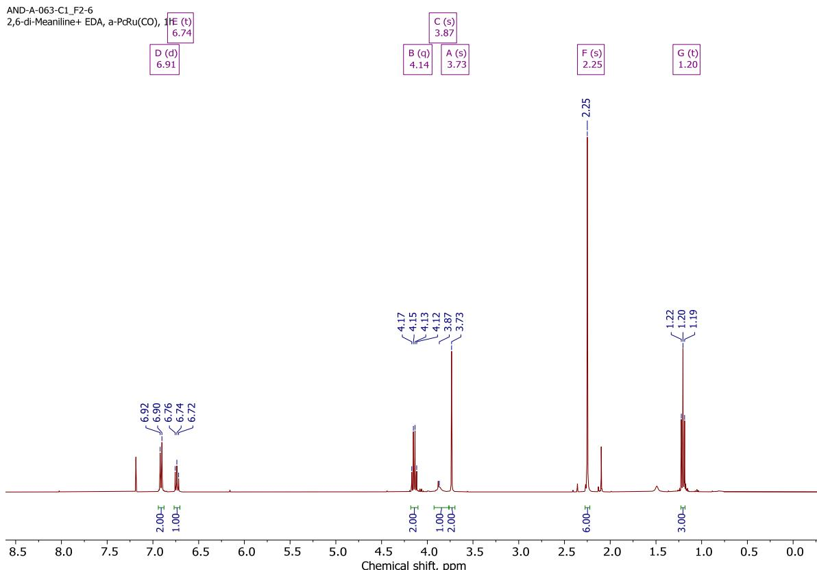
**Figure S59.** <sup>1</sup>H NMR spectrum of ethyl (2,6-dimethylphenyl)glycinate **3g**.
