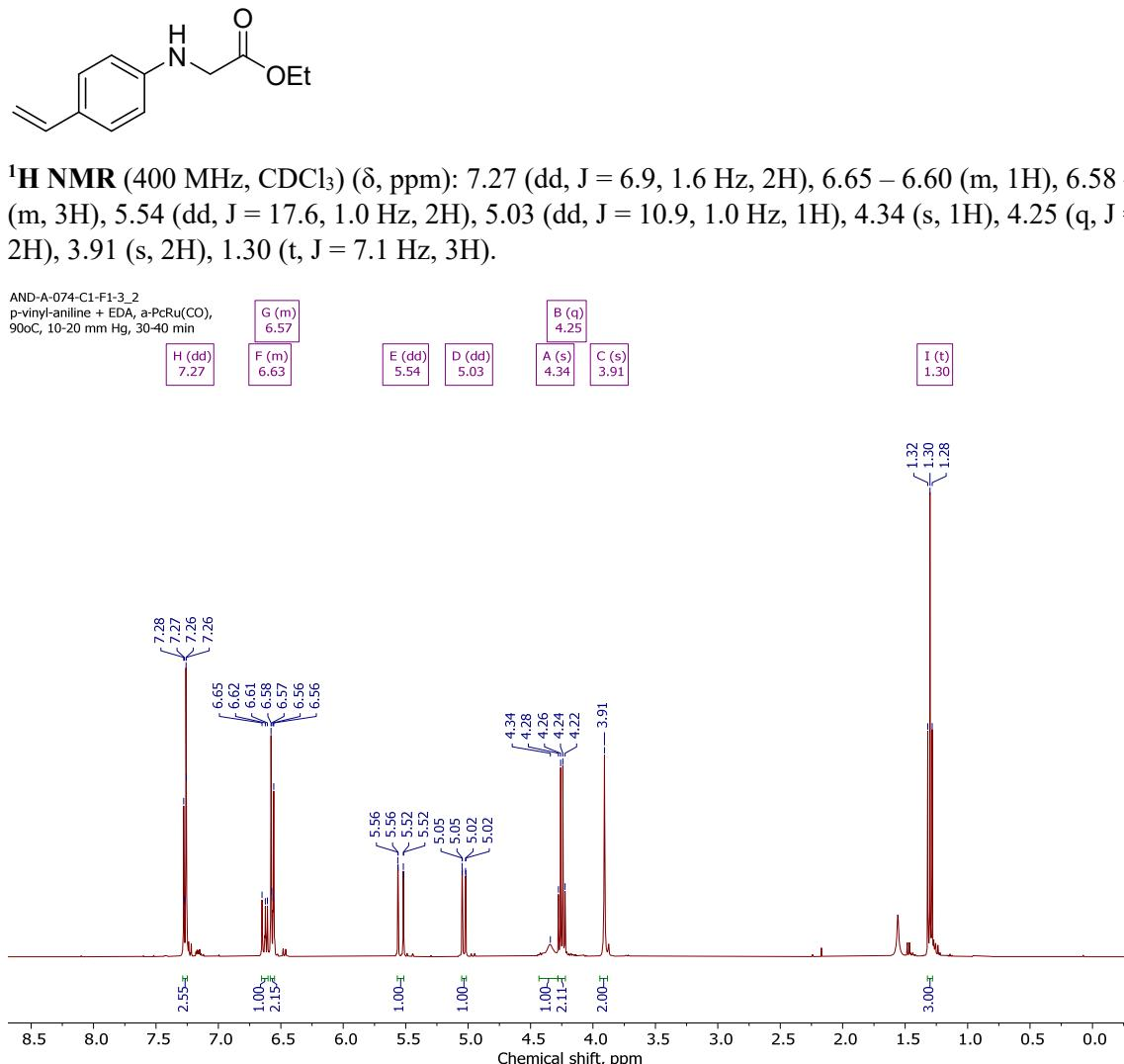
**Figure S82.**  $^1\text{H}$  NMR spectrum of ethyl (4-vinylphenyl)glycinate **3j**.
