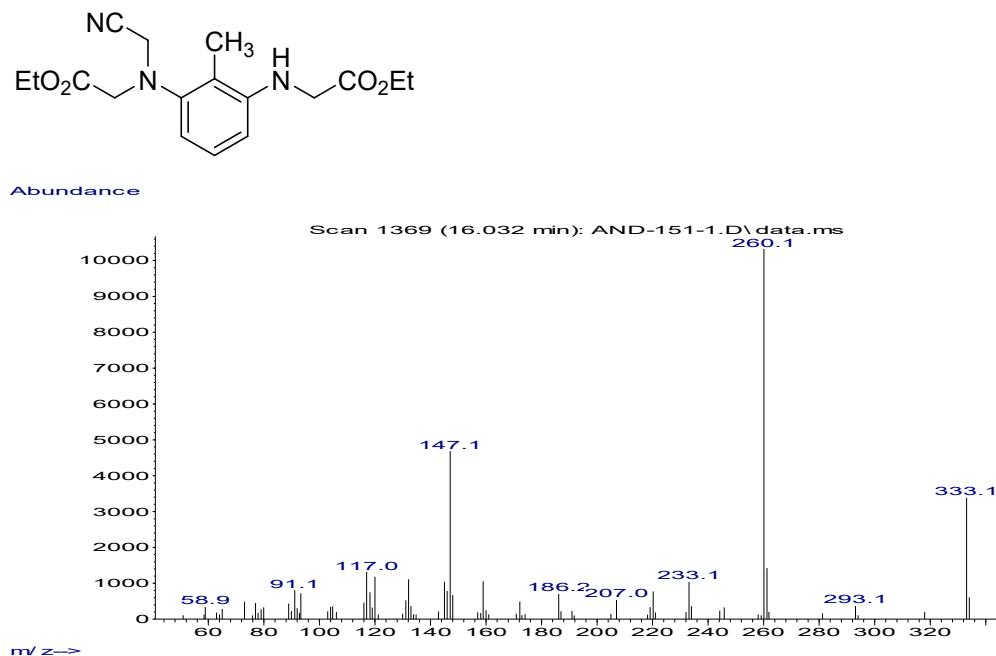
**Figure S138.** Mass spectrum (EI) of ethyl (3-((cyanomethyl)(2-ethoxy-2-oxoethyl)amino)-2-methylphenyl)glycinate.
