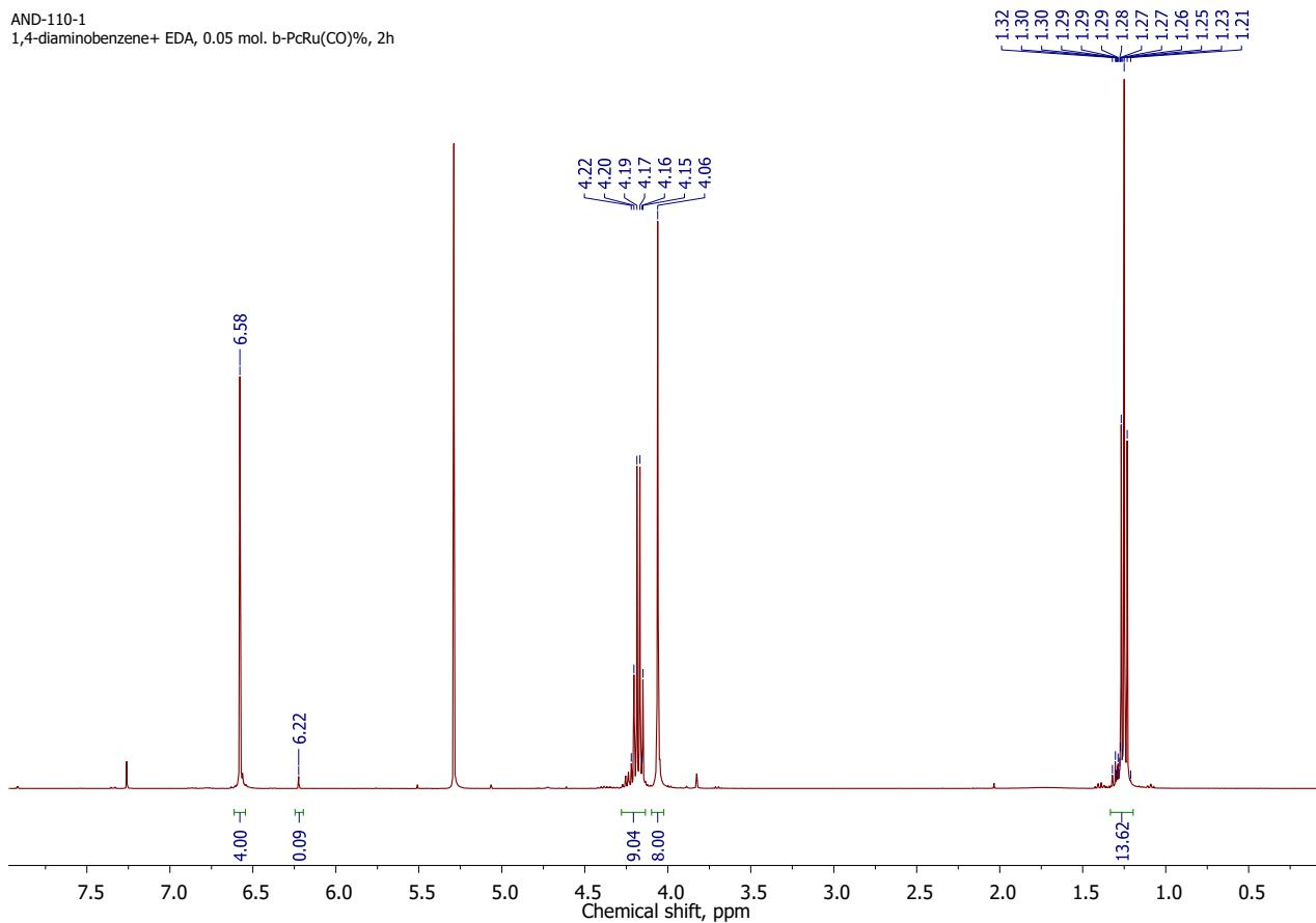
**Figure S98.**  $^1\text{H}$  NMR spectrum of the reaction mixture after reaction of 1,4-diaminobenzene **5** with EDA in the presence of 0.05 mol. % **1 $\beta$** .
