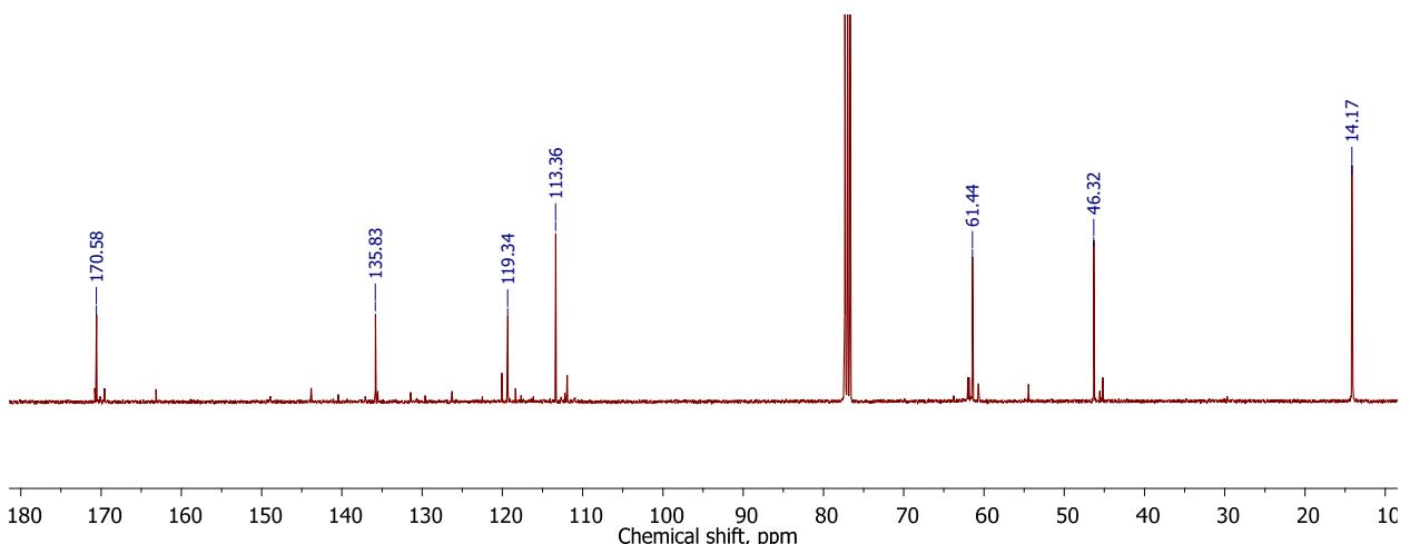
**Figure S111.** <sup>13</sup>C NMR spectrum of diethyl 2,2'-(2,5-dichloro-1,4-phenylene)bis(azanediyl))diacetate 6ss.
