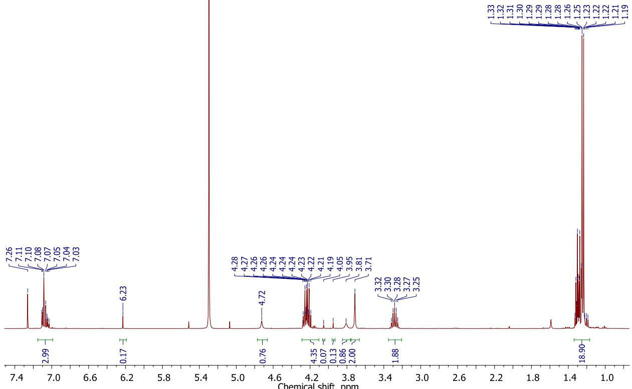
**Figure S65.** <sup>1</sup>H NMR spectrum of the reaction mixture after reaction of EDA with 2,6-diisopropylaniline **2h** in the presence of 0.15 mol. % **1a**.
