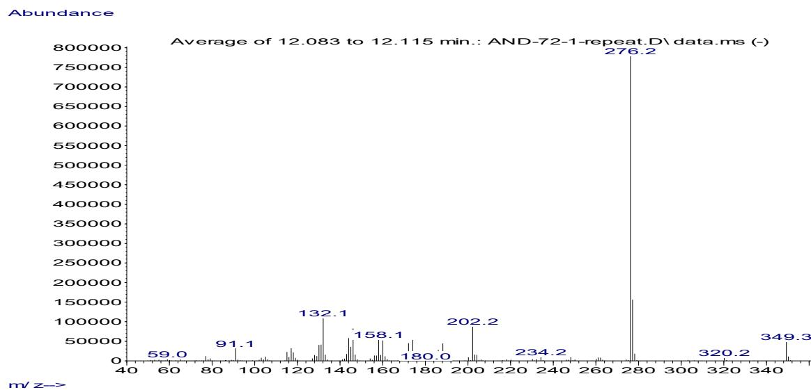
**Figure S73.** Mass spectrum (EI) of diethyl 2,2'-(2,6-diisopropylphenyl)azanediyl)diacetate **4h**.
