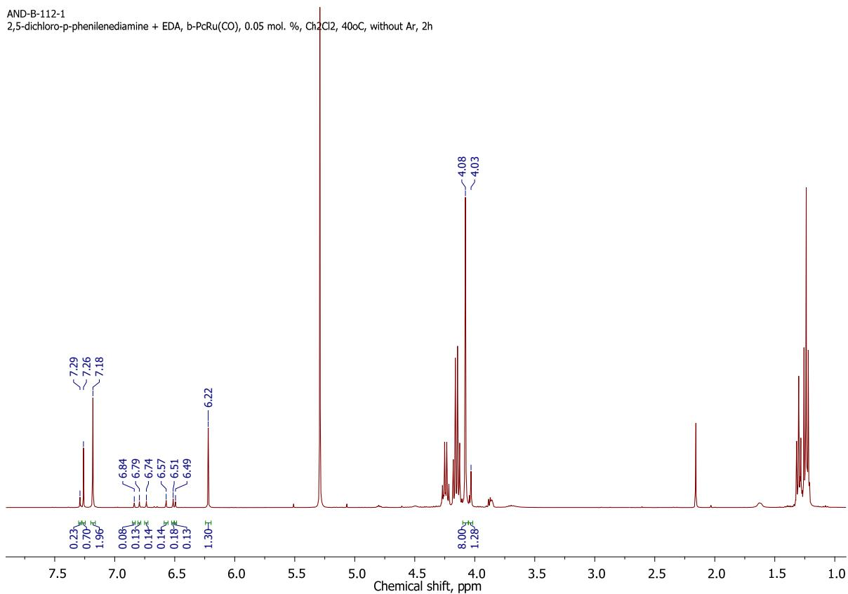
**Figure S109.**  $^1\text{H}$  NMR spectrum of the reaction mixture after reaction of 2,5-dichlorobenzene-1,4-diamine **6** with EDA in the presence of 0.05 mol. % **1 $\beta$** . Reaction time: 3 h.
