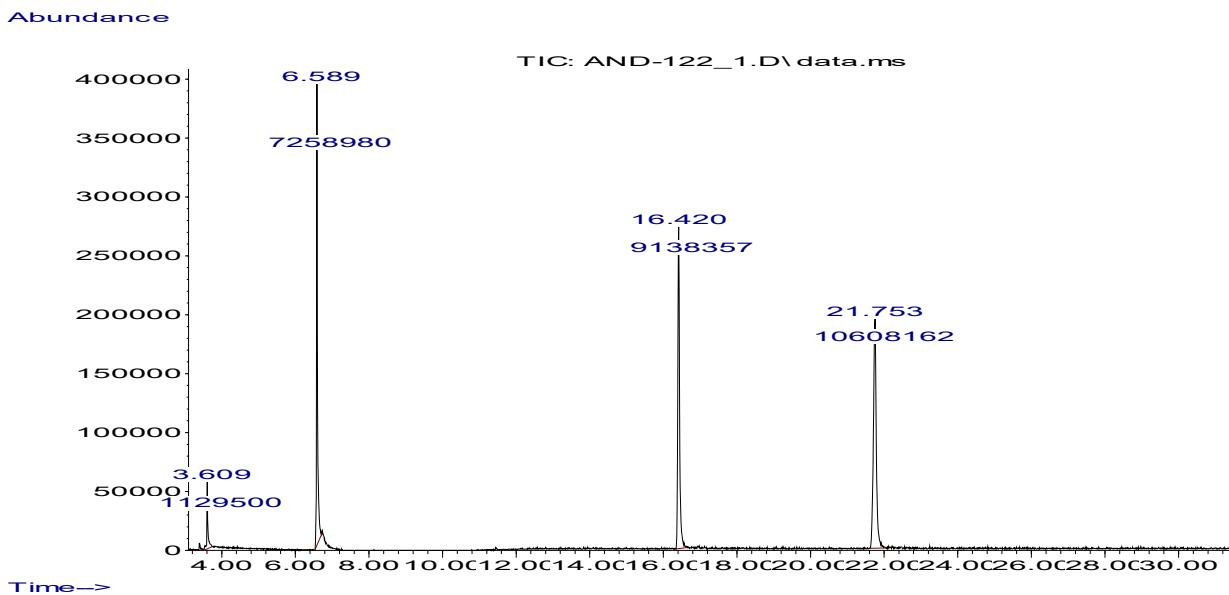
**Figure S105.** Chromatogram of the reaction mixture after reaction of 2,5-dichlorobenzene-1,4-diamine **6** with EDA in the presence of 0.15 mol. % **1a**. Reaction time: 2 h.
