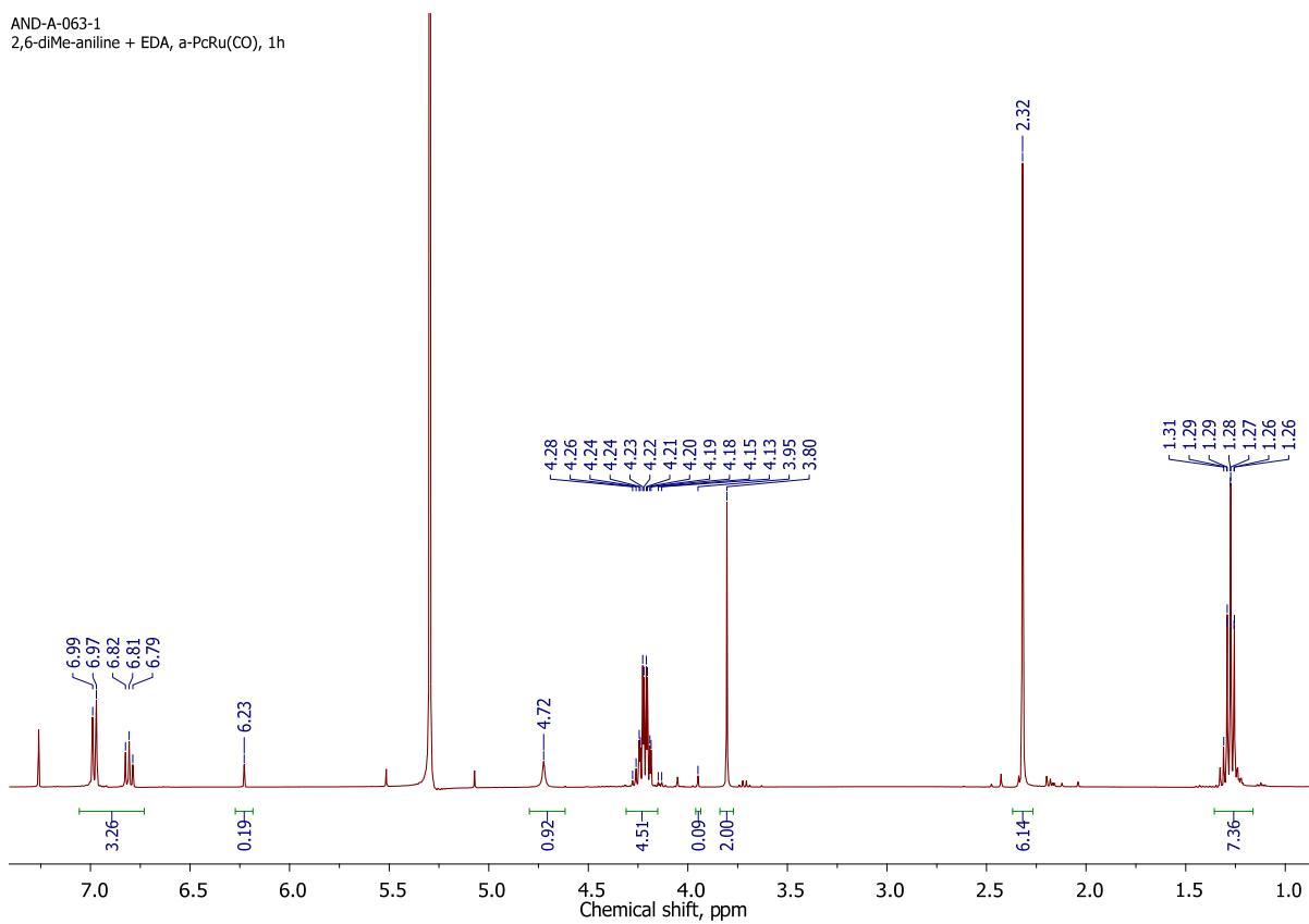
**Figure S57.**  $^1\text{H}$  NMR spectrum of the reaction mixture after reaction of EDA with 2,6-dimethylaniline **2g** in the presence of 0.15 mol. % **1a**.
