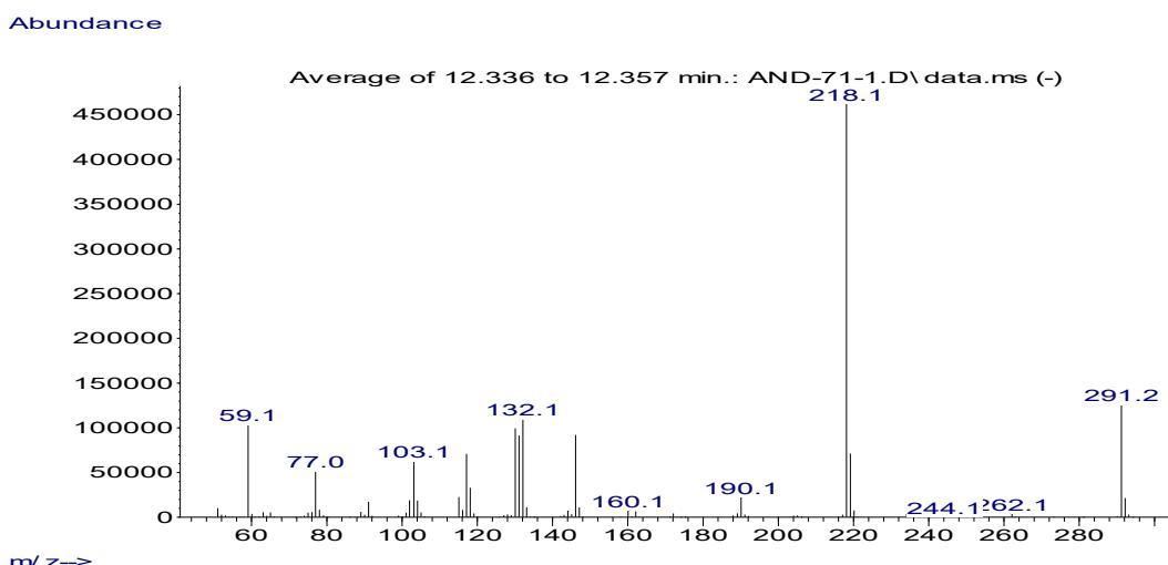
**Figure S87.** Mass spectrum (EI) of diethyl 2,2'-(4-vinylphenyl)azanediyl diacetate **4j**.
