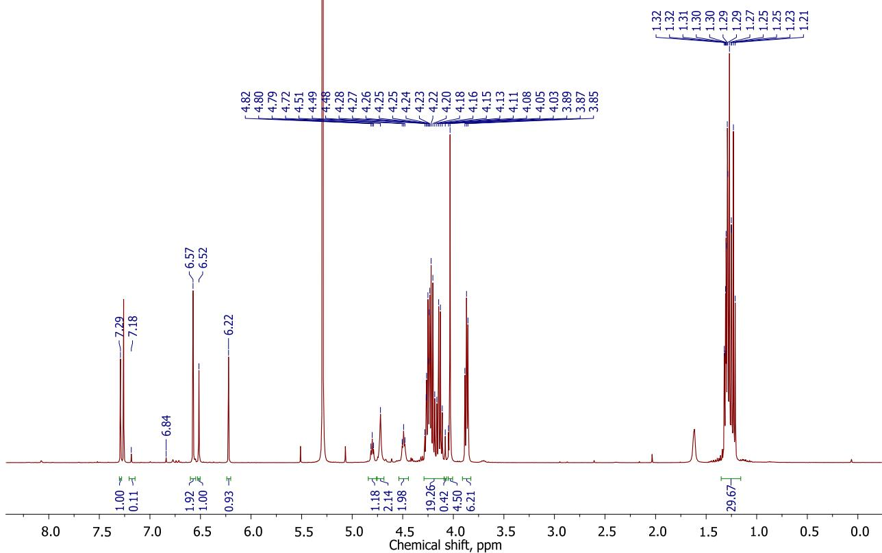
**Figure S104.** <sup>1</sup>H NMR spectrum of the reaction mixture after reaction of 2,5-dichlorobenzene-1,4-diamine **6** with EDA in the presence of 0.15 mol. % **1a** for 2h.
