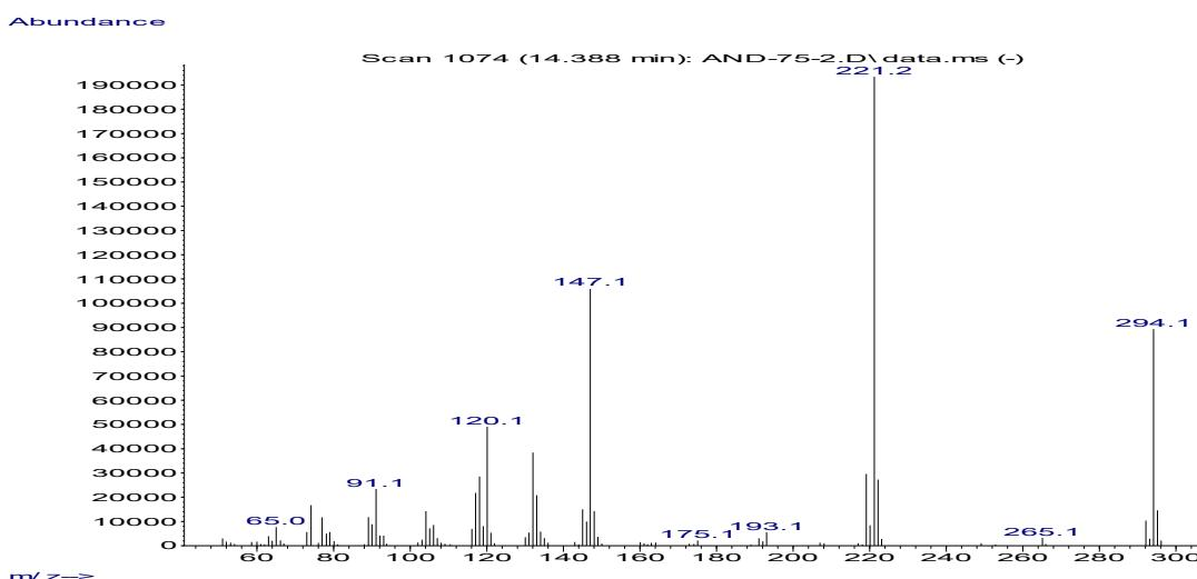
**Figure S119.** Mass spectrum (EI) of diethyl 2,2'-(2-methyl-1,3-phenylene)bis(azanediyl)diacetate 7ss.
