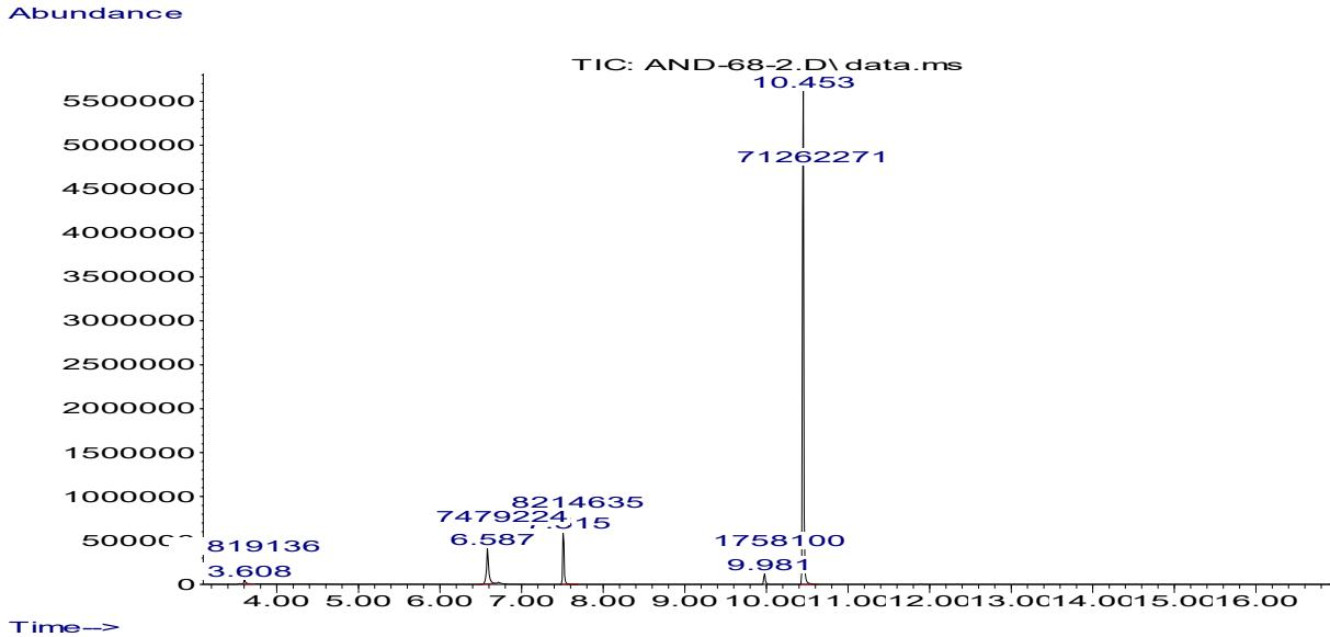
**Figure S75.** Chromatogram of the reaction mixture after reaction of EDA with 2-(*tert*-butyl)aniline **2i** in the presence of 0.15 mol. % **1a**.
