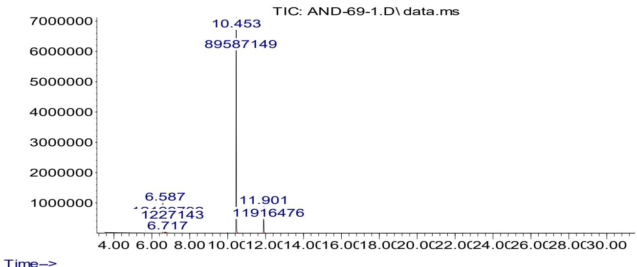
**Figure S79.** Chromatogram of the reaction mixture after reaction of EDA with 2-(*tert*-butyl)aniline **2i** in the presence of 0.05 mol. % **1β**.
