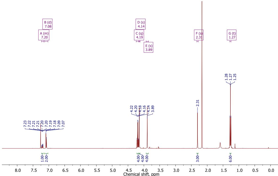
**Figure S139.**  $^1\text{H NMR}$  spectrum of diethyl 2,2'-(2-methyl-1,3-phenylene)bis((cyanomethyl)azanediyil))diacetate **11**.
