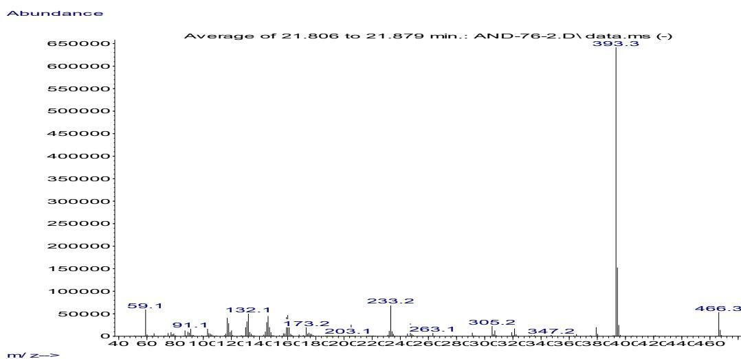
**Figure S126.** Mass spectrum (EI) of tetraethyl 2,2',2'',2'''-((2-methyl-1,3-phenylene)bis(azanetriyl))tetraacetate **7dd**.
