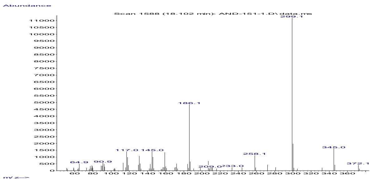
**Figure S142.** Mass spectrum (EI) of diethyl 2,2'-(2-methyl-1,3-phenylene)bis((cyanomethyl)azanediyl))diacetate **11**.
