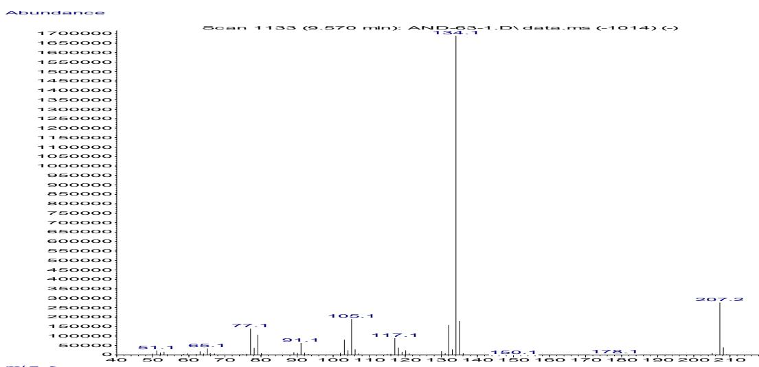
**Figure S60.** Mass spectrum (EI) of ethyl (2,6-dimethylphenyl)glycinate **3g**.
