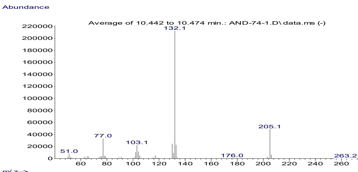
**Figure S83.** Mass spectrum (EI) of ethyl (4-vinylphenyl)glycinate **3j**.
