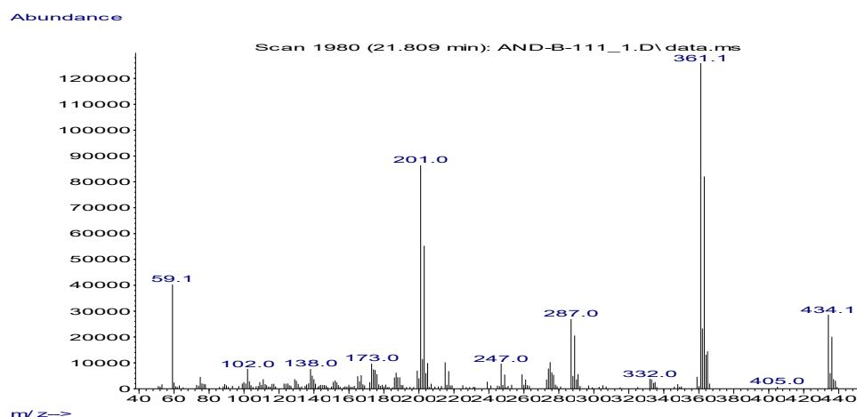
**Figure S108.** Mass spectrum (EI) of diethyl 2,2'-(2,5-dichloro-4-((2-ethoxy-2-oxoethyl)amino)phenyl)azanediyl)diacetate **6sd**.
