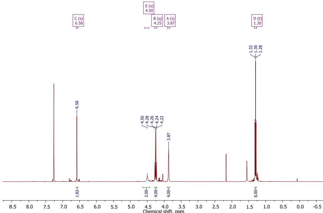
**Figure S110.** <sup>1</sup>H NMR spectrum of diethyl 2,2'-(2,5-dichloro-1,4-phenylene)bis(azanediyl))diacetate, 6ss.
