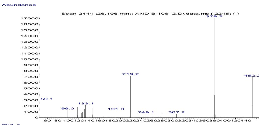
**Figure S101.** Mass spectrum (EI) of tetraethyl 2,2',2'',2'''-(1,4-phenylenebis(azanetriyl))tetraacetate 5dd.
