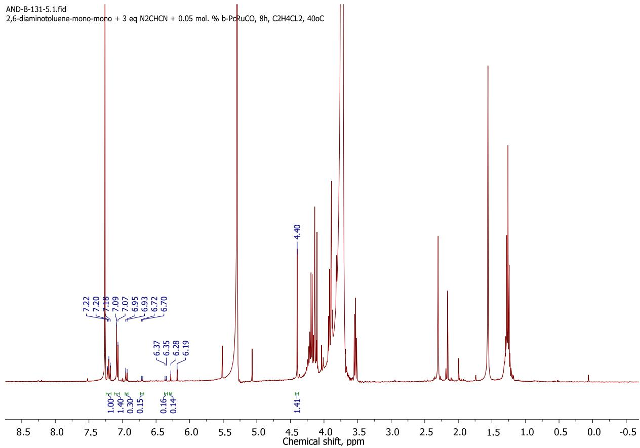
**Figure S137.** <sup>1</sup>H NMR spectrum of the reaction mixture after reaction of diethyl 2,2'-(2-methyl-1,3-phenylene)bis(azanediyl)diacetate **7ss** with 2.1 eq. diazoacetonitrile in C<sub>2</sub>H<sub>4</sub>Cl<sub>2</sub> (0.57 M) in the presence of 0.20 mol. % **1β**.
