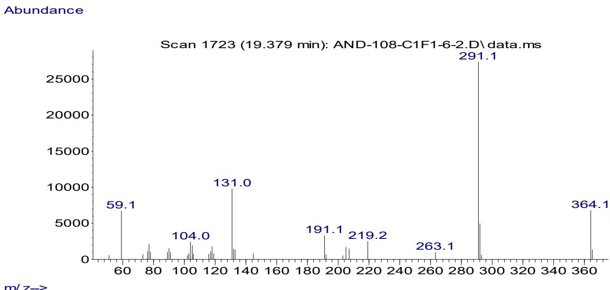
**Figure S103.** Mass spectrum (EI) of diethyl 2,2'-(4-((2-ethoxy-2-oxoethylidene)amino)phenyl)azanediyl)-diacetate **5s'd**.
