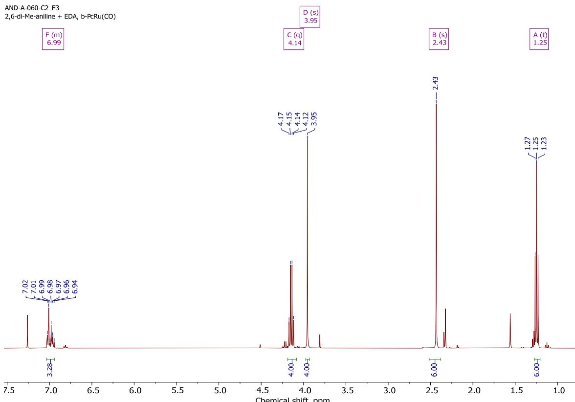
**Figure S63.** <sup>1</sup>H NMR spectrum of diethyl 2,2'-(2,6-dimethylphenyl)azanediyldiacetate **4g**.
