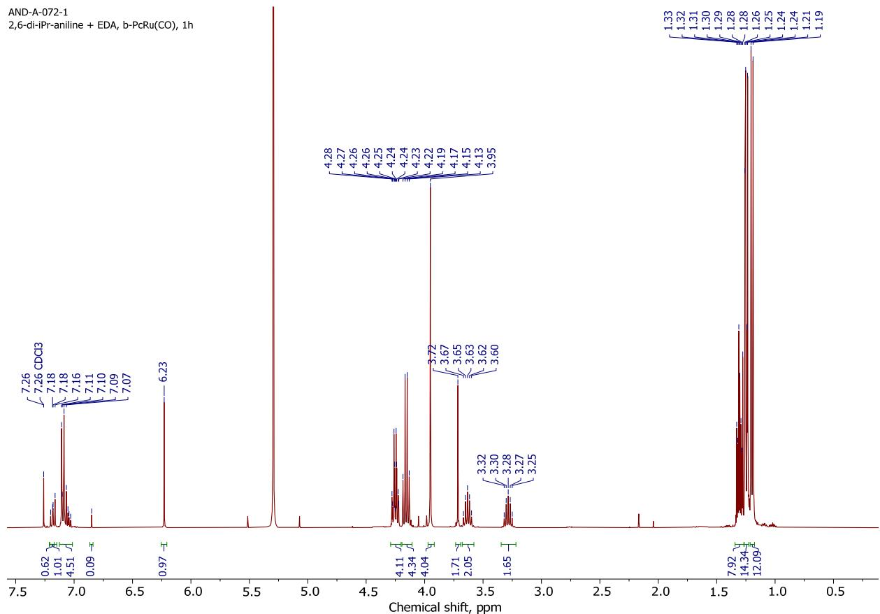
**Figure S69.**  $^1\text{H}$  NMR spectrum of the reaction mixture after reaction of EDA with 2,6-diisopropylaniline **2h** in the presence of 0.05 mol. % **1\beta**.
