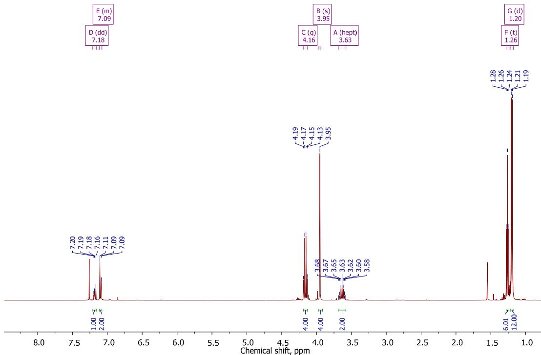
**Figure S71.** <sup>1</sup>H NMR spectrum of diethyl 2,2'-(2,6-diisopropylphenyl)azanediyl diacetate **4h**.
