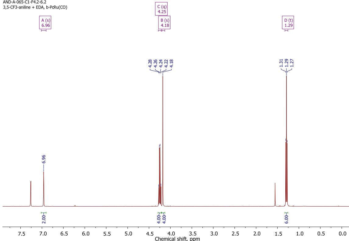
**Figure S53.** <sup>1</sup>H NMR spectrum of diethyl 2,2'-(*(3,5-bis(trifluoromethyl)phenyl)azanediyl*)diacetate **4f**.
