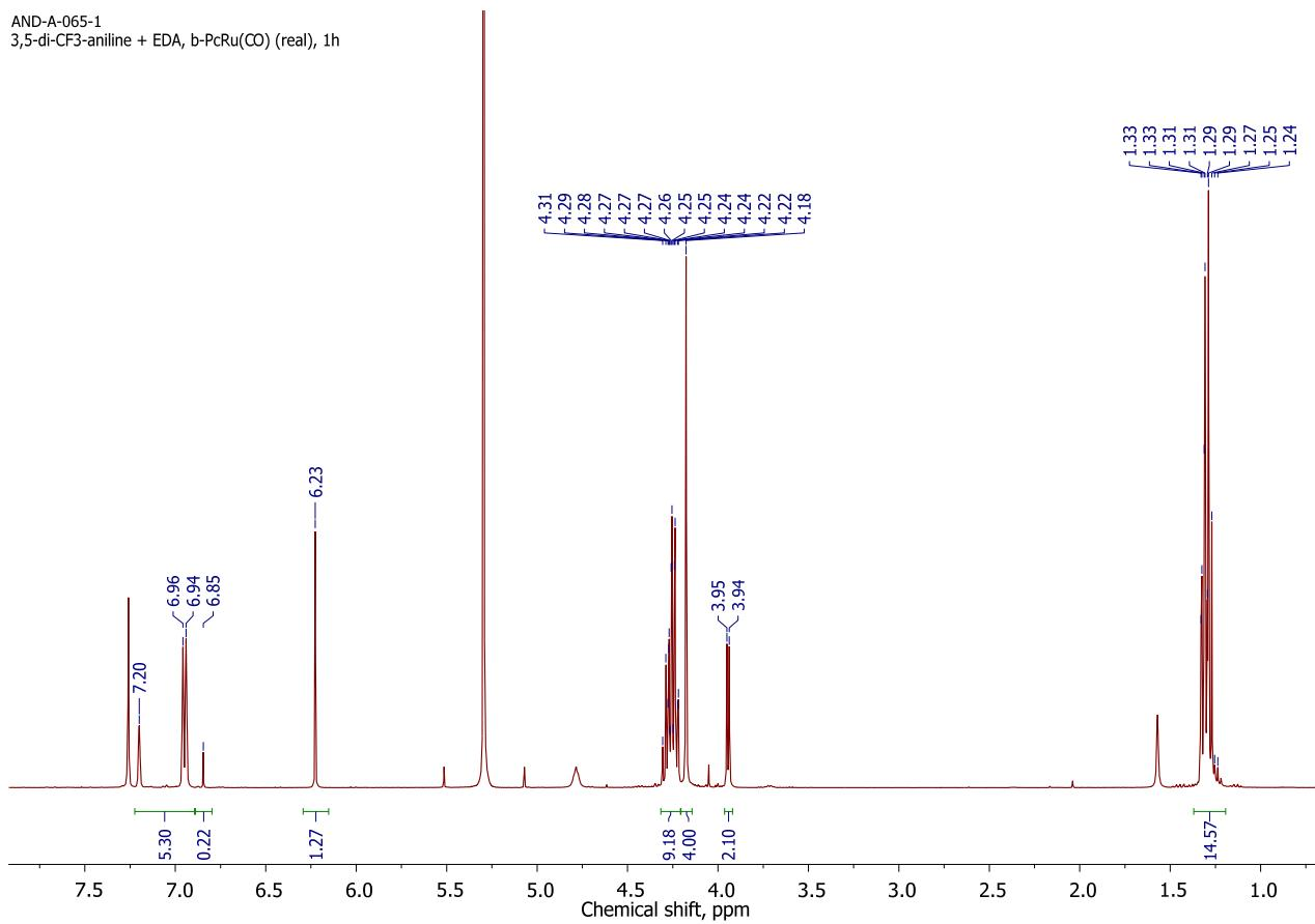
**Figure S51.**  $^1\text{H}$  NMR spectrum of the reaction mixture after reaction of EDA with 3,5-bis(trifluoromethyl)aniline **2f** in the presence of 0.05 mol. % **1 $\beta$** .
