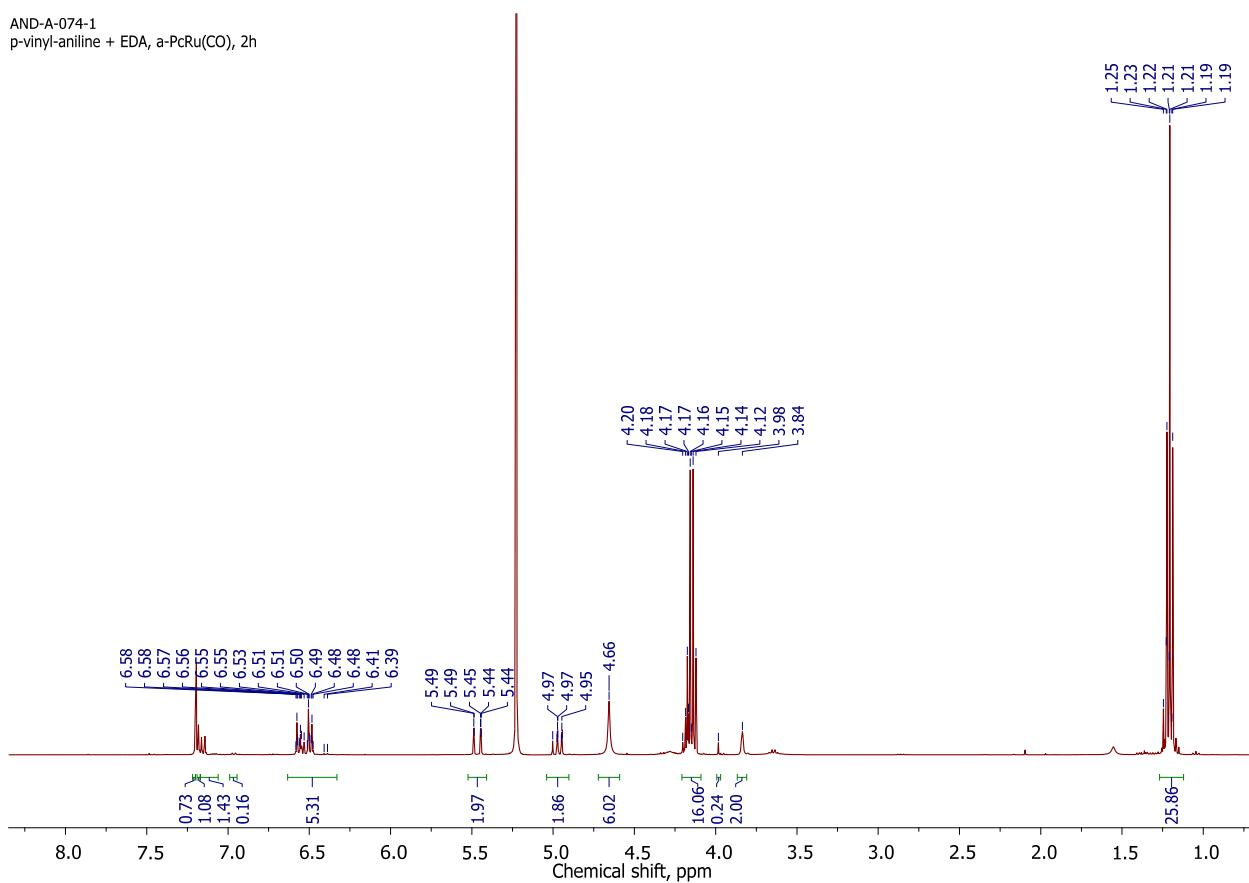
**Figure S80.**  $^1\text{H}$  NMR spectrum of the reaction mixture after reaction of EDA with 4-vinylaniline **2j** in the presence of 0.15 mol. % **1\alpha**.
