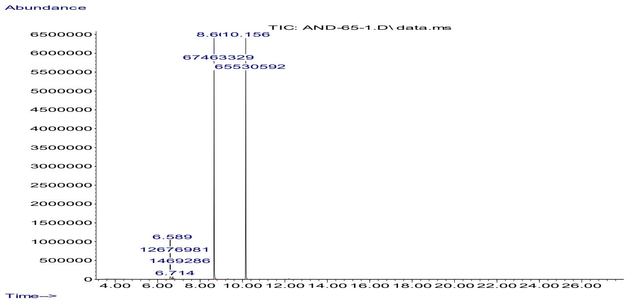
**Figure S52.** Chromatogram of the reaction mixture after reaction of 3,5-bis(trifluoromethyl)aniline **2f** with EDA in the presence of 0.05 mol. % **1 $\beta$** .
