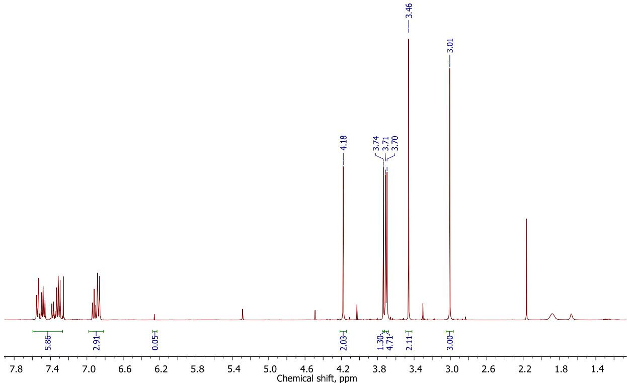
**Figure S127.** <sup>1</sup>H NMR spectrum of the organic phase after extraction of the reaction mixture from the reaction of N-methylaniline **8** with diazoacetonitrile (generated in situ) in the presence of 0.1 mol. % **1β** in CH<sub>2</sub>Cl<sub>2</sub>/H<sub>2</sub>O emulsion.
