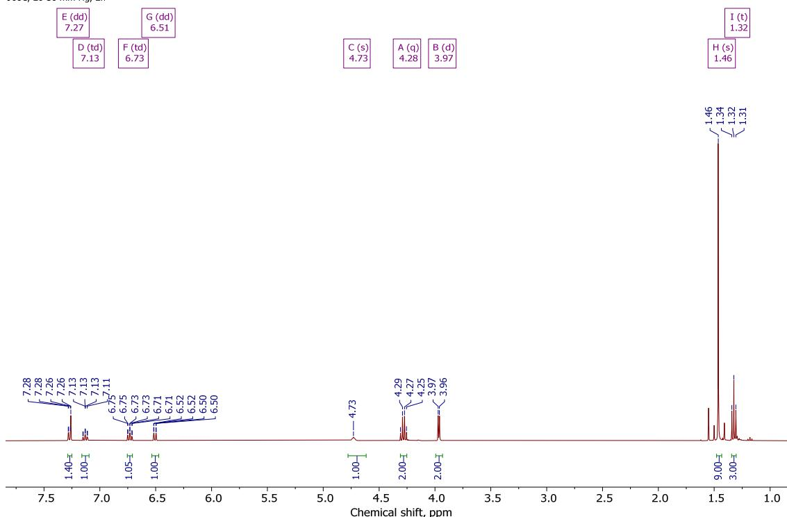
**Figure S76.** <sup>1</sup>H NMR spectrum of ethyl (2-(*tert*-butyl)phenyl)glycinate **3i**.
