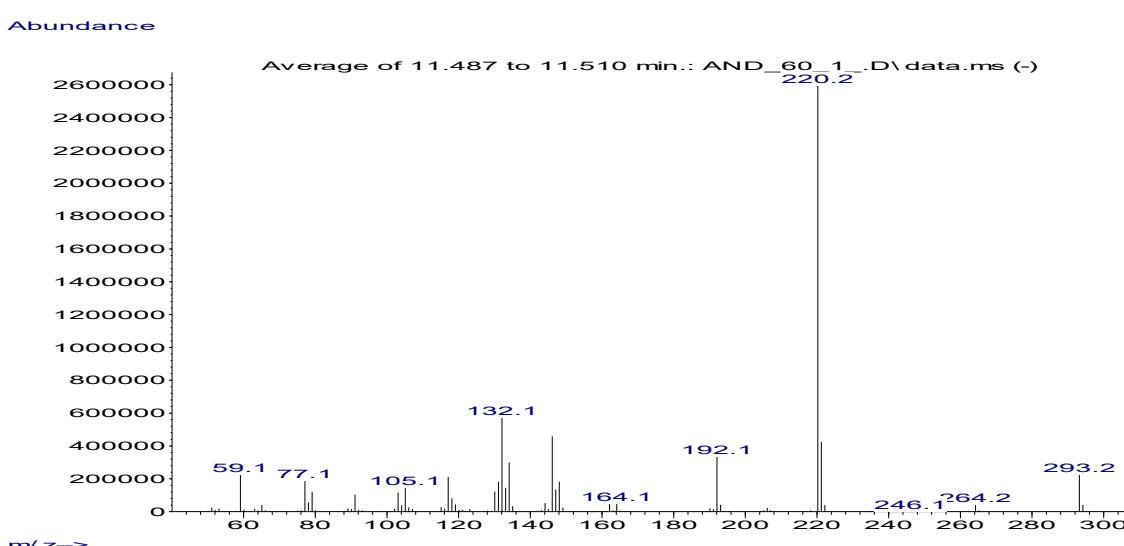
**Figure S64.** Mass spectrum (EI) of diethyl 2,2'-(2,6-dimethylphenyl)azanediyldiacetate **4g**.
