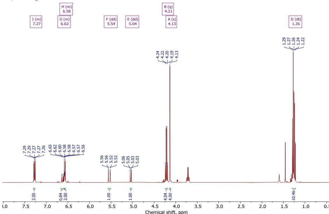
**Figure S86.** <sup>1</sup>H NMR spectrum of diethyl 2,2'-(4-vinylphenyl)azanediyl diacetate **4j**.
