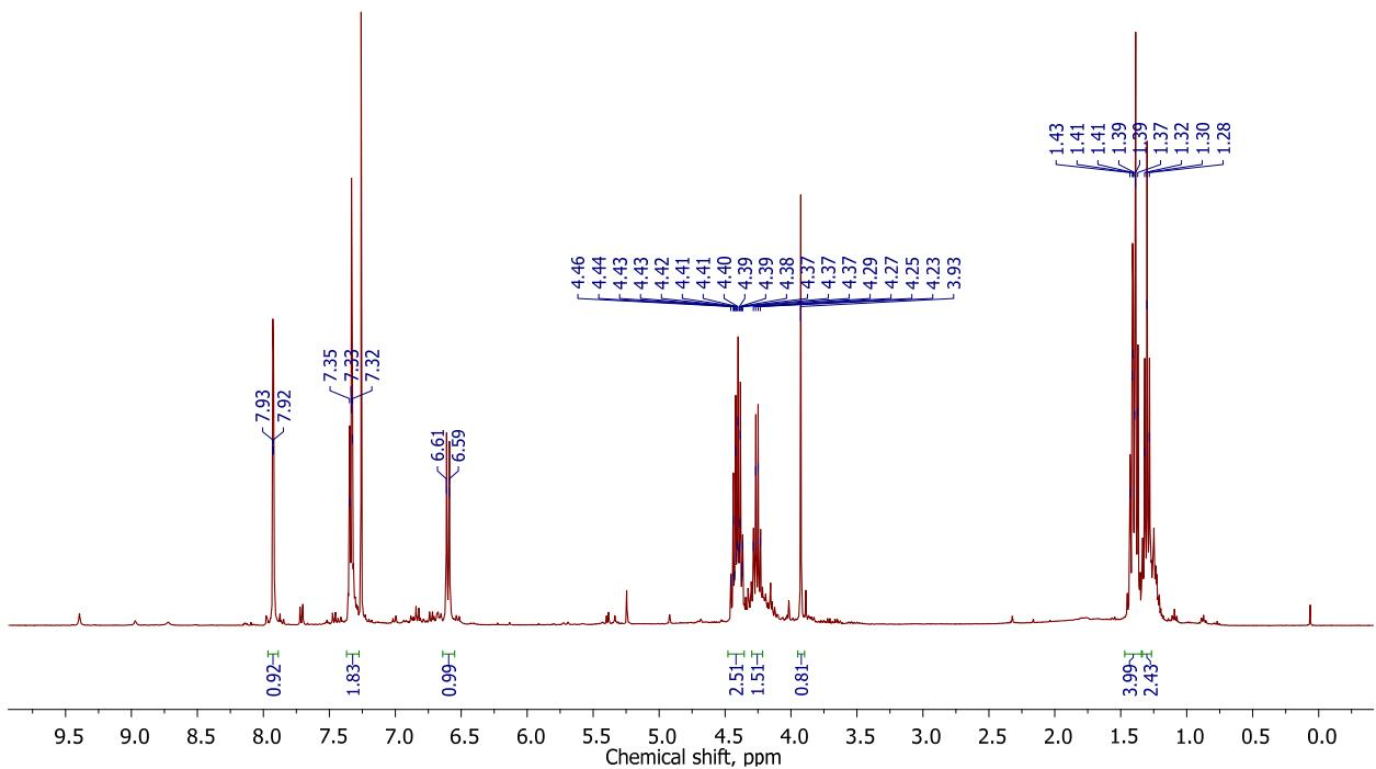
**Figure S97.**  $^1\text{H}$  NMR spectrum of mixture of the target SS-insertion product (diethyl 2,2'-(1,4-phenylenebis(azanediyl))diacetate) **5ss** and ethyl 2-((4-((2-ethoxy-2-oxoethyl)amino)phenyl)imino)acetate **5s's**, isolated by chromatography on Al<sub>2</sub>O<sub>3</sub> column after reaction of 1,4-diaminobenzene with EDA in the presence of 0.30 mol. % **1 $\alpha$** .
