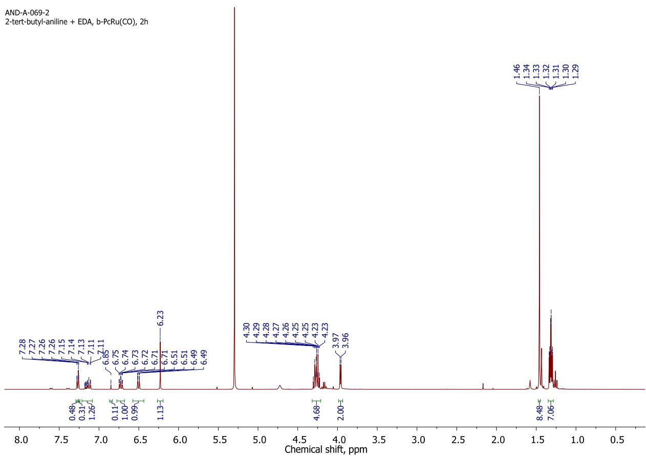
**Figure S78.** <sup>1</sup>H NMR spectrum of the reaction mixture after reaction of EDA with 2-(*tert*-butyl)aniline **2i** in the presence of 0.05 mol. % **1β**.
