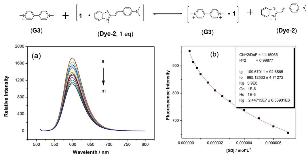
**Figure S22.** (a) Competitive fluorescence titration spectra of **Dye-2c1** upon sequential addition of **G5** ( $[I] = 0.001$  mM,  $[Dye-2] = 0.001$  mM,  $[G3] = 0 - 0.007$  mM); (b) nonlinear curve-fitting of fluorescence changes at 630 nm.
