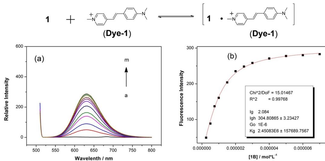
**Figure S19.** (a) Fluorescence titration spectra for **Dye-1** upon sequential addition of **1** ( $[\text{Dye-1}] = 0.001$  mM,  $[\text{1}] = 0 - 0.007$  mM); (b) nonlinear curve-fitting of fluorescence changes at 630 nm.
