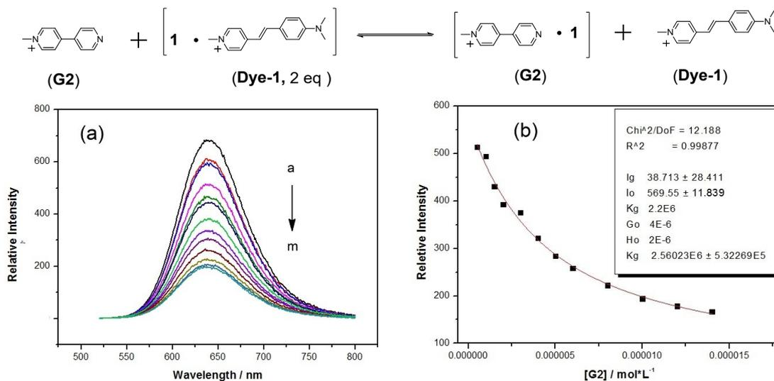
**Figure S21.** (a) Competitive fluorescence titration spectra for **Dye-1**–**1** upon sequential addition of **G2** ([**1**] = 0.002 mM, [**Dye-1**] = 0.004 mM, [**G2**] = 0 – 0.014 mM); (b) nonlinear curve-fitting of fluorescence changes at 630 nm.
