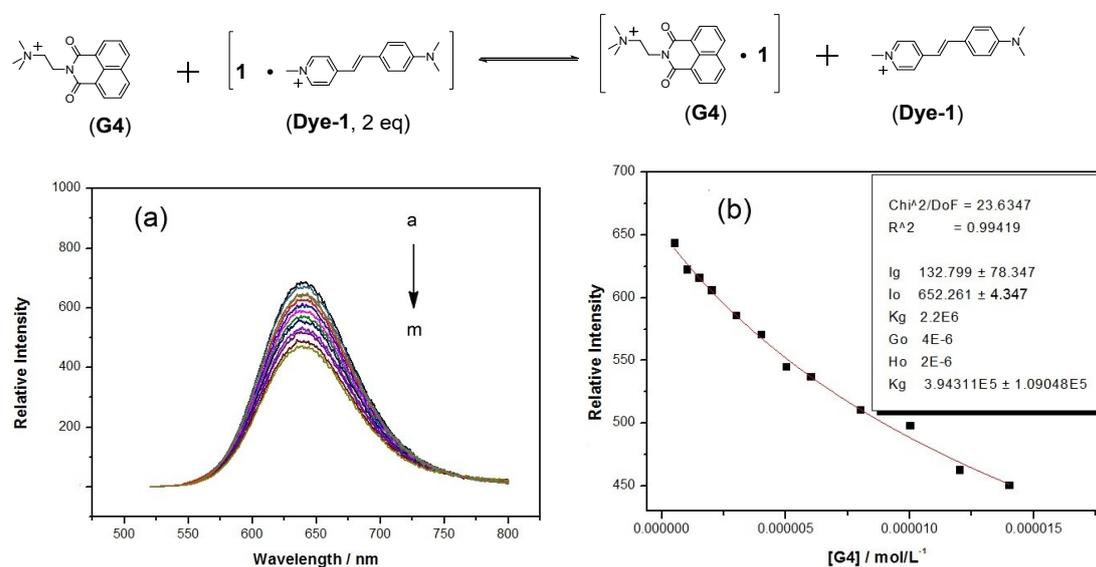
**Figure S23.** (a) Competitive fluorescence titration spectra of **Dye-1c1** upon sequential addition of **G4** ( $[I] = 0.002$  mM,  $[Dye-1] = 0.004$  mM,  $[G4] = 0 - 0.014$  mM); (b) nonlinear curve-fitting of fluorescence changes at 630 nm.
