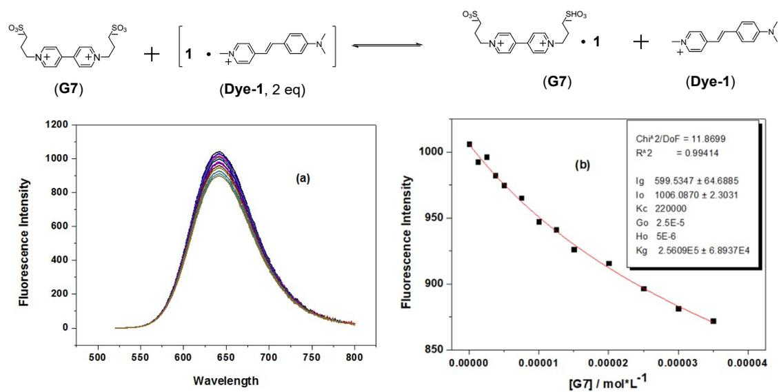
**Figure S26.** Competitive fluorescence titration spectra of (a) **Dye-1** upon sequential addition of **G7** ( $[\text{Dye-1}] = 0.010 \text{ mM}$ ,  $[\mathbf{1}] = 0.005 \text{ mM}$ ,  $[\text{G7}] = 0 - 0.07 \text{ mM}$ ) and (b) nonlinear curve-fitting of fluorescence changes at 650 nm.
