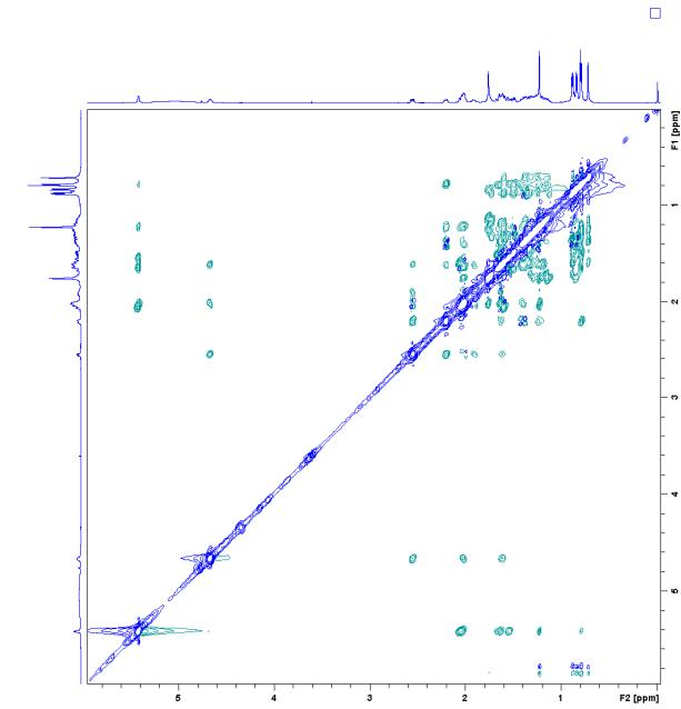
**Figure S36** ROESY spectrum of **8** in pyridine-*d*<sub>5</sub> at 600 MHz
