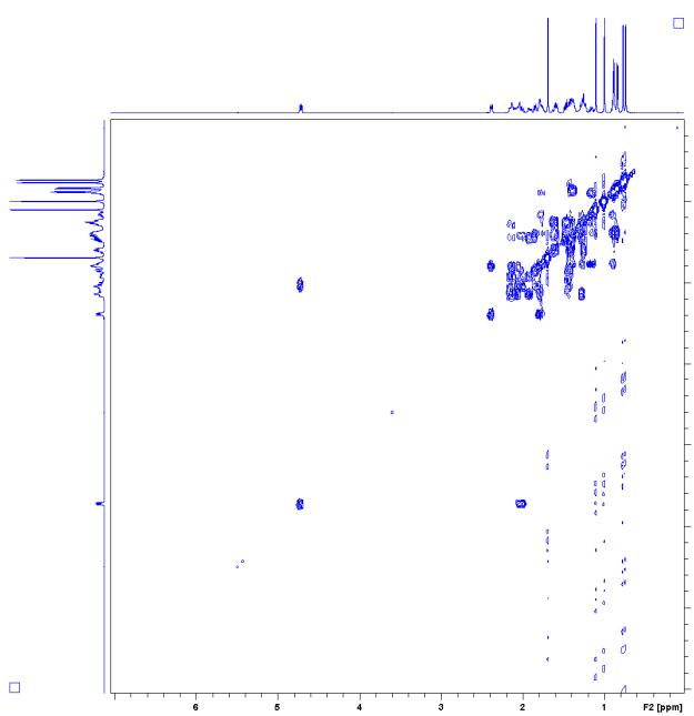
**Figure S58**  $^1\text{H}$ - $^1\text{H}$  COSY spectrum of **12** in pyridine- $d_5$  at 600 MHz
