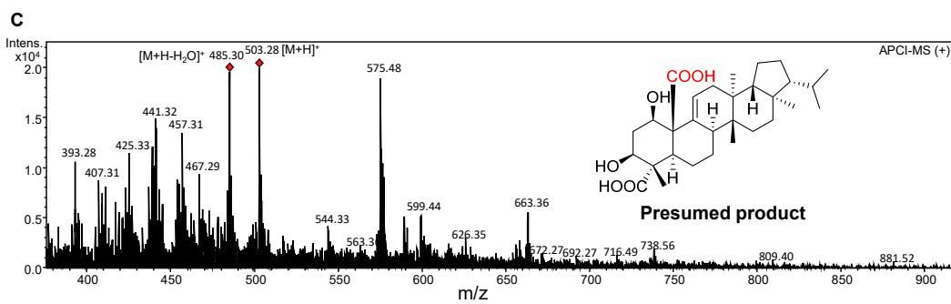
**Figure S49** MS analysis of *A. oryzae* NSAR1 transformants co-expressing *efuA<sub>TC</sub>* and *polC/E*
