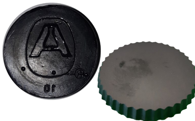
Figure S3 Moulded object made of poly(S-Dipentene-DAS).
