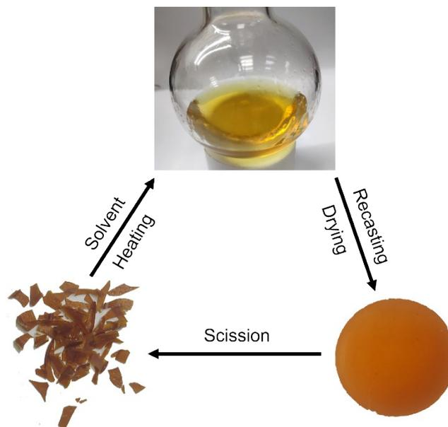
**Figure S17.** Reprocessing procedure of **PU-H<sub>5</sub>** samples: small pieces of polyurethane network were immersed in DMF and heated to 80 °C for 5 h to form a homogenous solution. Subsequently, the solution was poured into Teflon mold for recasting and a new polyurethane film was afforded after drying in vacuo.
