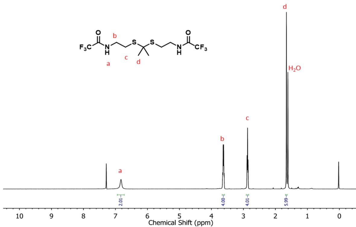
Fig. S5. <sup>1</sup>H NMR characterization of B2.
