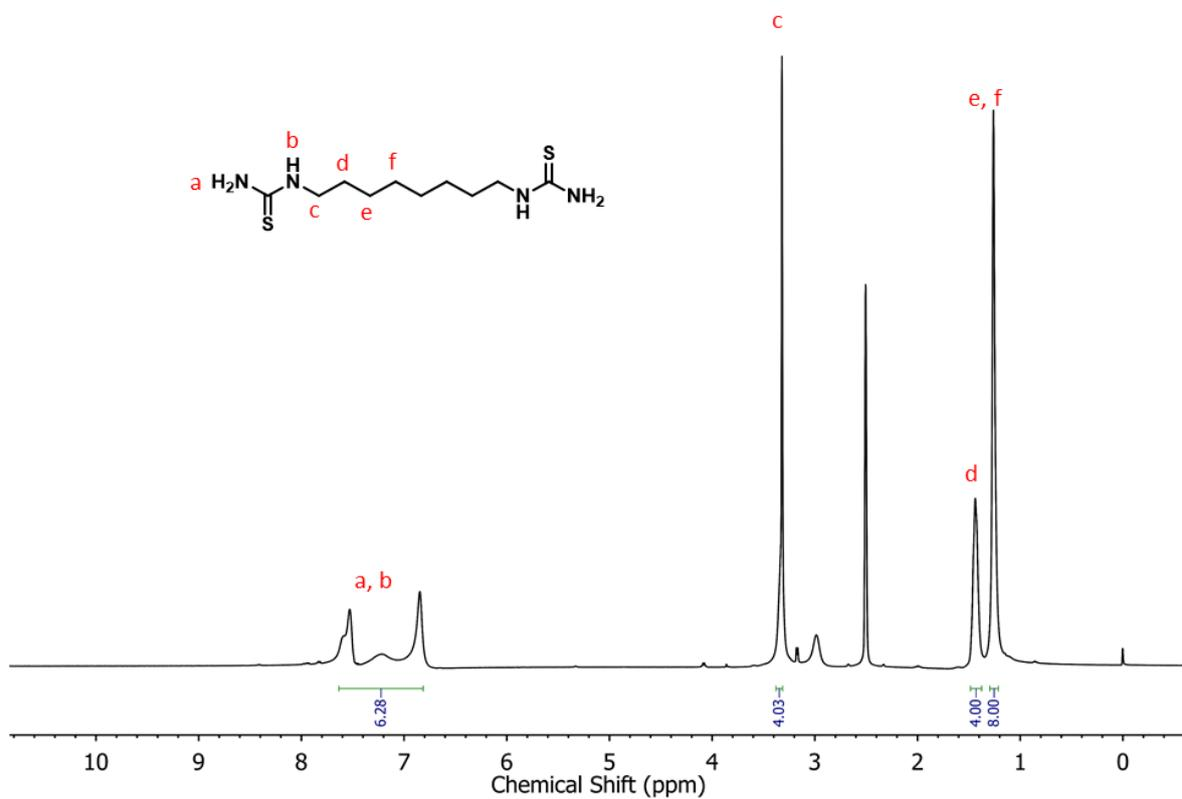
Fig. S21. <sup>1</sup>H NMR characterization of M3-2.
