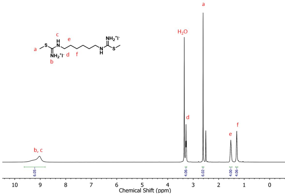
Fig. S17. <sup>1</sup>H NMR characterization of M2-3.
