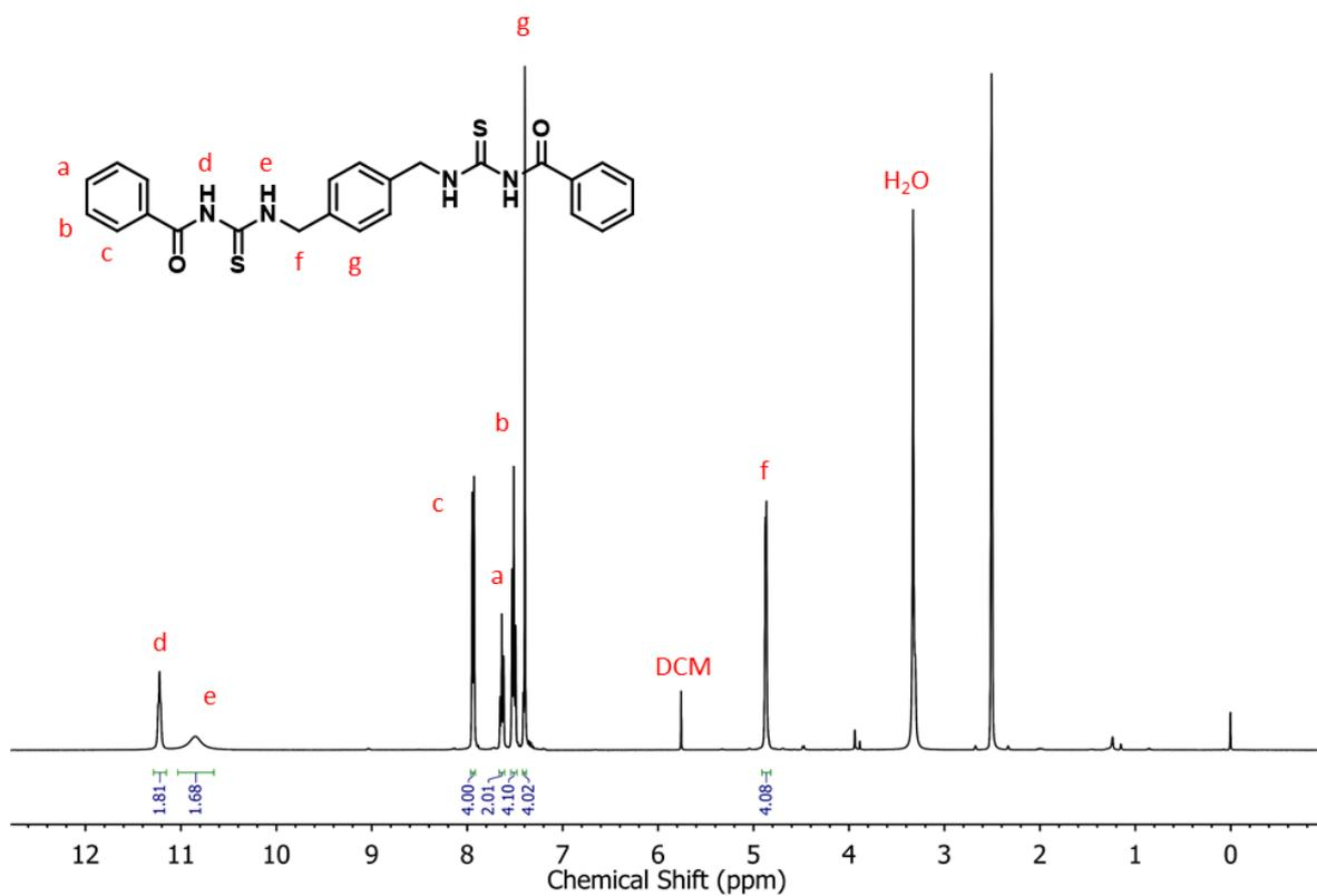
Fig. S31.  $^1\text{H}$  NMR characterization of M5-1.
