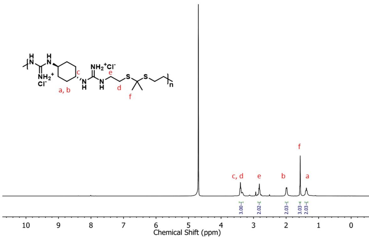
Fig. S44.  $^1\text{H}$  NMR characterization of P4B.
