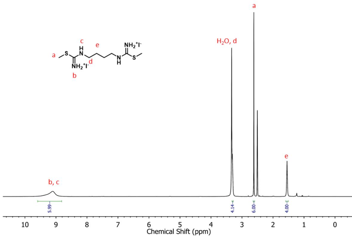
**Fig. S11.**  $^1\text{H}$  NMR characterization of M1-3.
