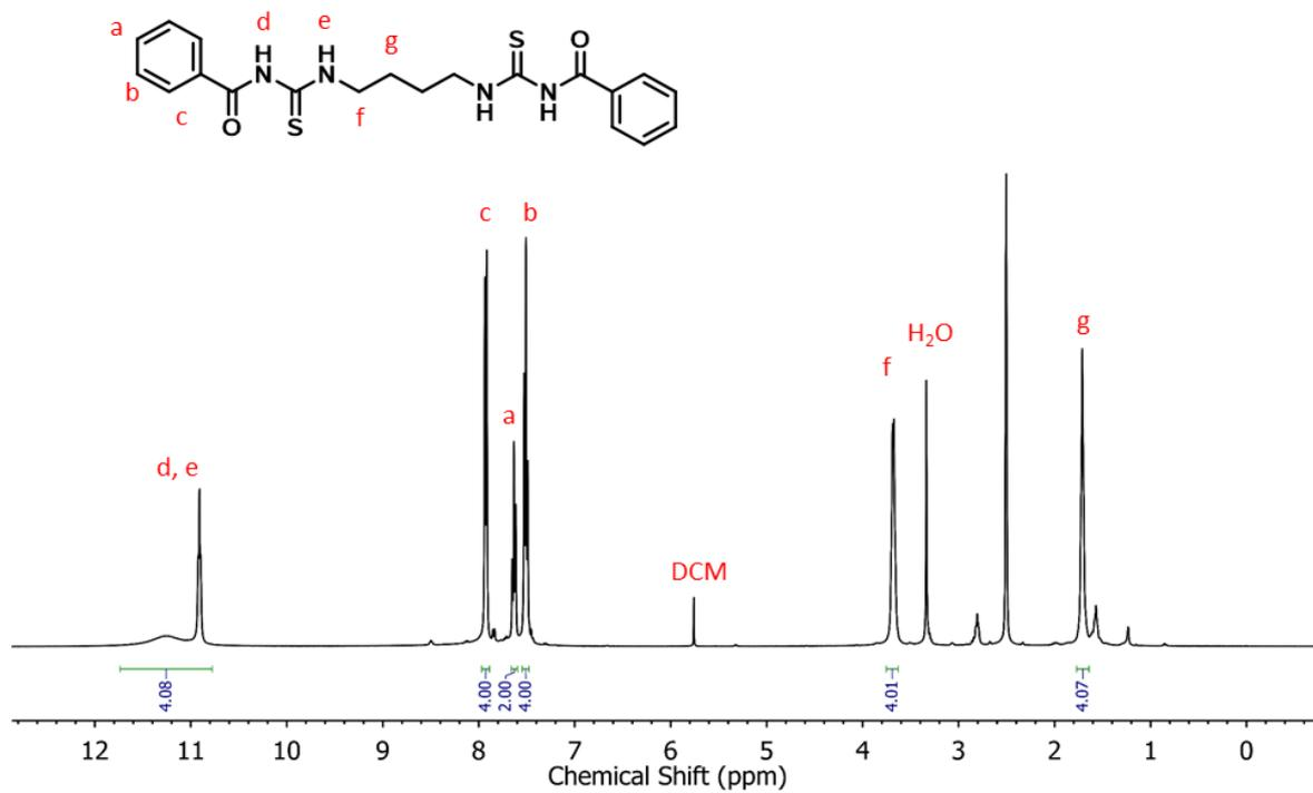
Fig. S7. <sup>1</sup>H NMR characterization of M1-1.
