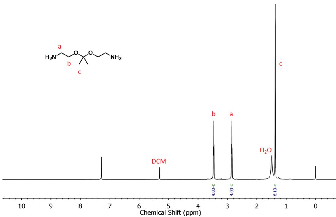
Fig. S3. <sup>1</sup>H NMR characterization of A3.
