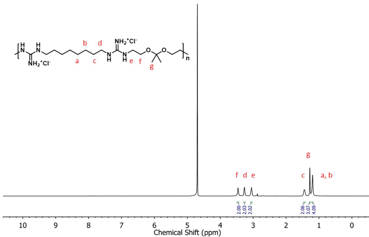
Fig. S41. <sup>1</sup>H NMR characterization of P3A.
