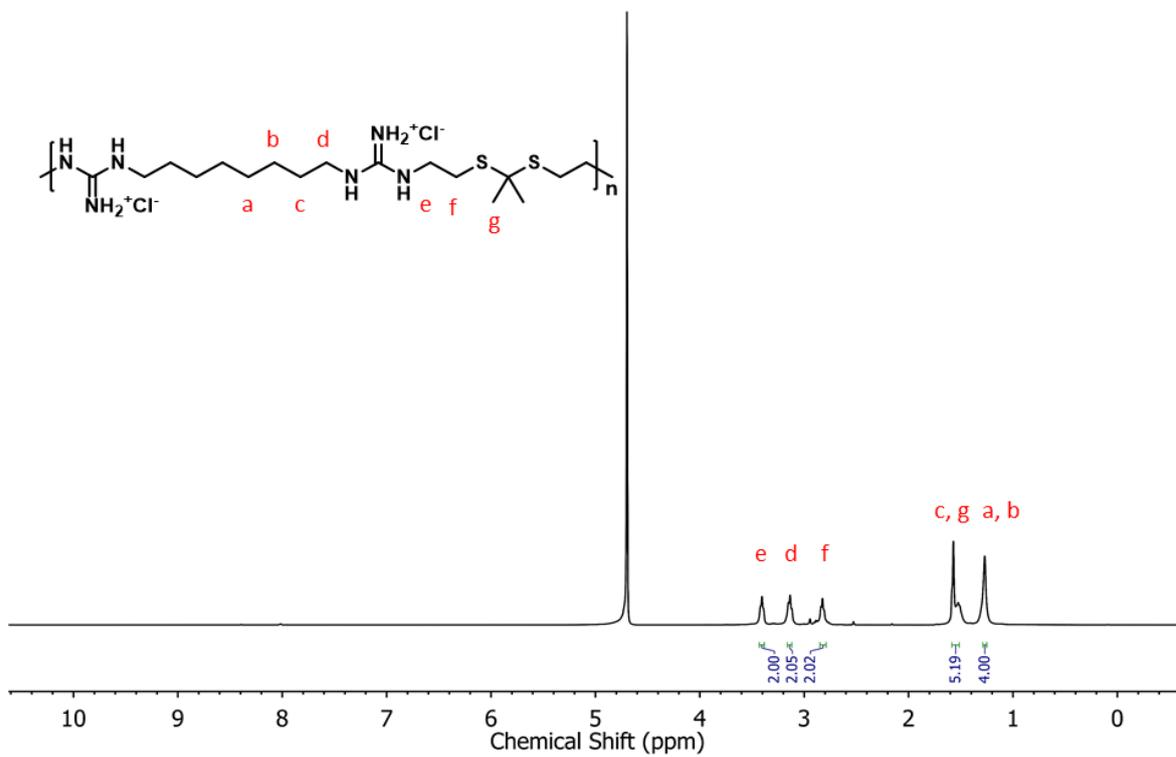
Fig. S42. <sup>1</sup>H NMR characterization of P3B.
