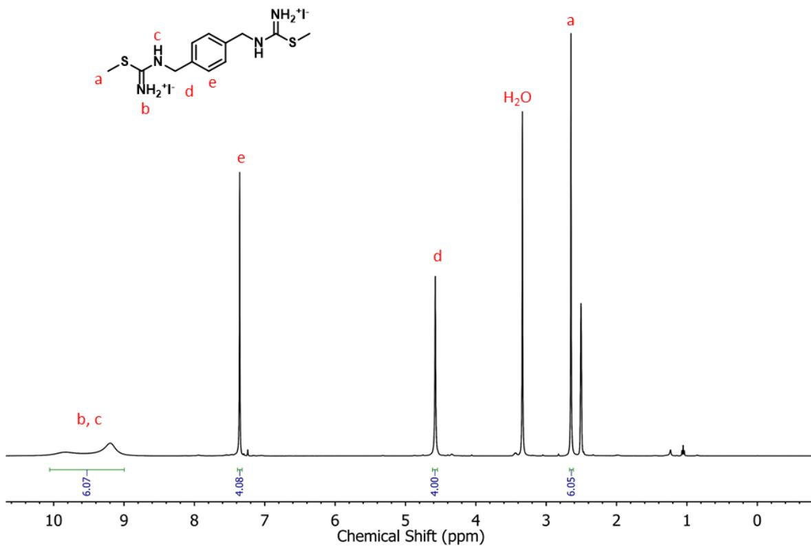
Fig. S35. <sup>1</sup>H NMR characterization of M5-3.
