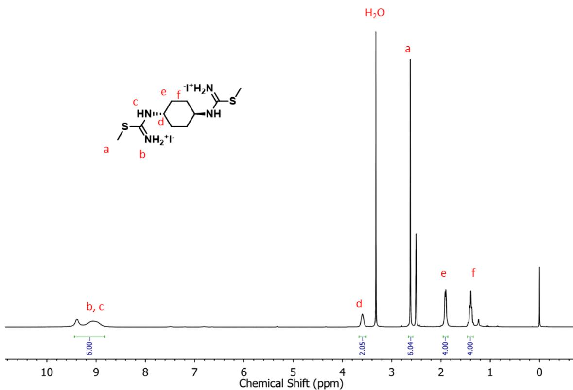
Fig. S29.  $^1\text{H}$  NMR characterization of M4-3.
