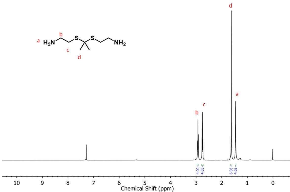
Fig. S6. <sup>1</sup>H NMR characterization of B3.
