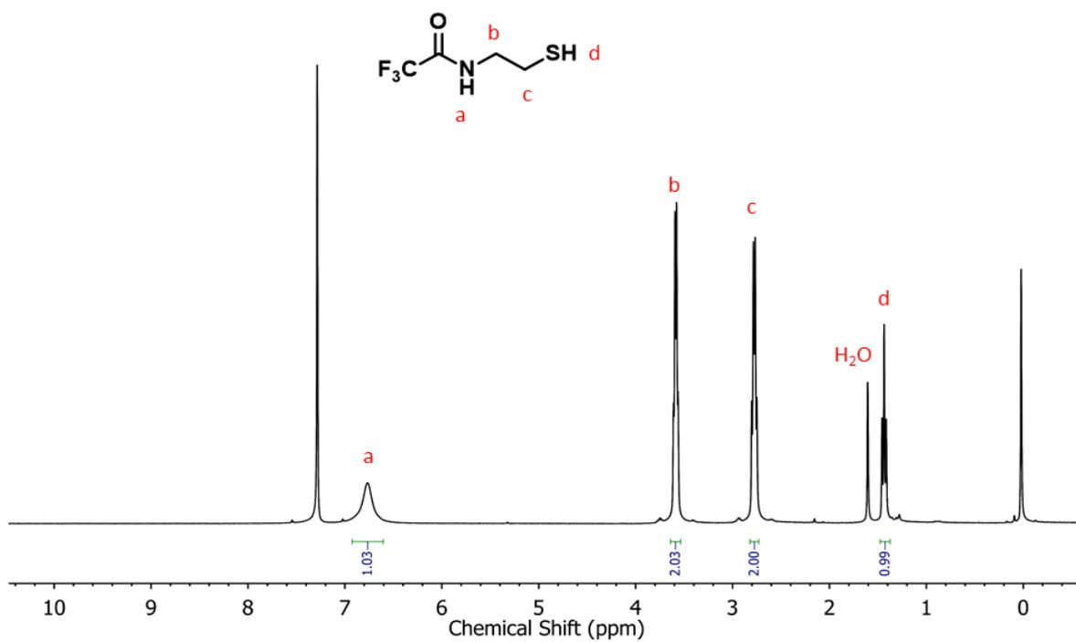
Fig. S4. <sup>1</sup>H NMR characterization of B1.
