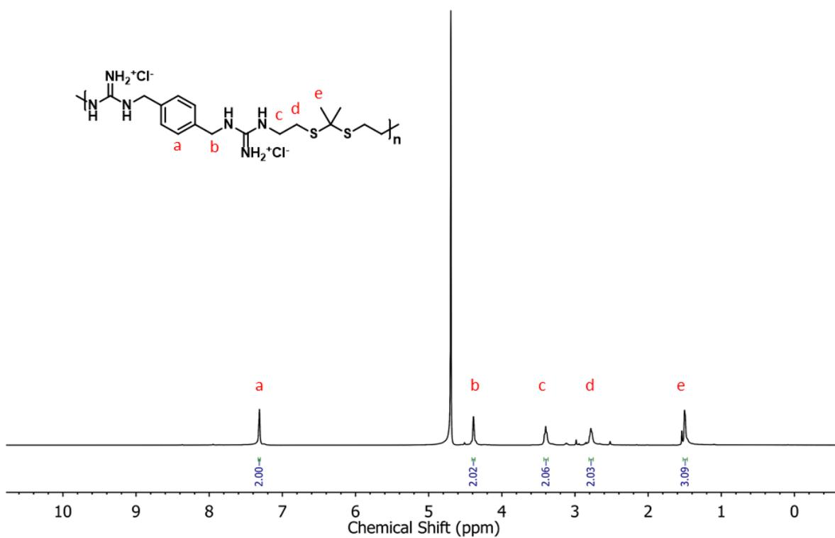
Fig. S46. <sup>1</sup>H NMR characterization of P5B.
