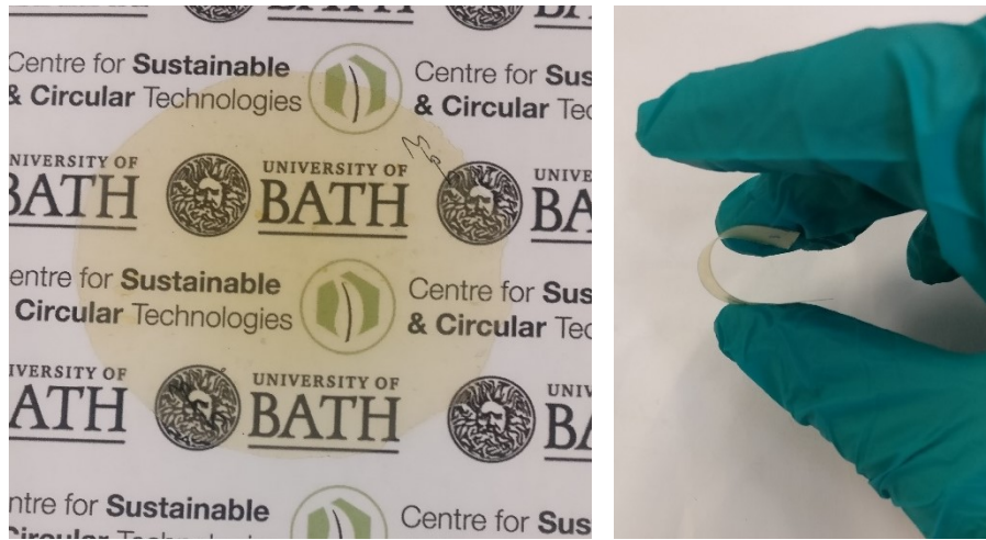
Figure S15. Compression moulded films of PA6F.
