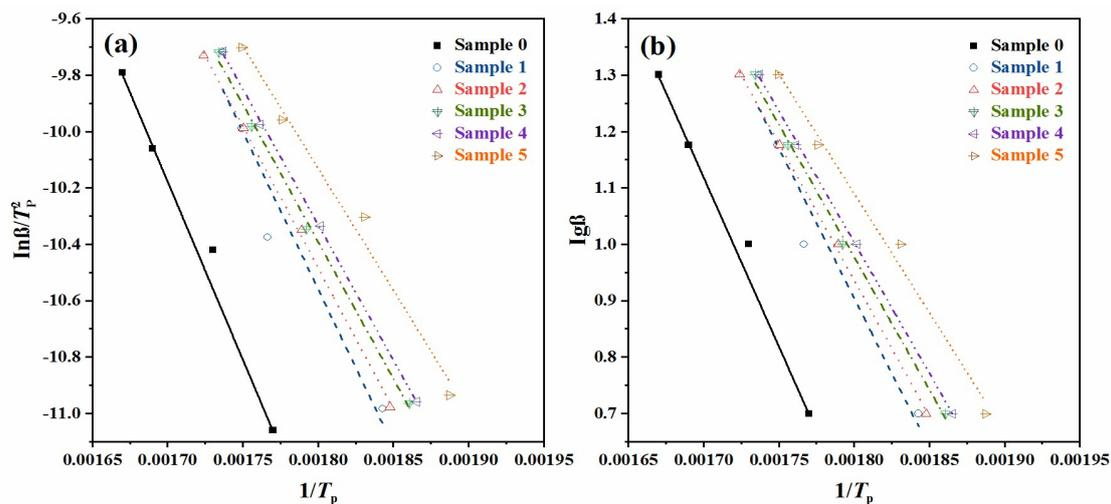
**Figure S2.** Kinetic curves of the curing reaction for unmodified BADCy and *m*-BADCy resin calculated by Kissinger (a) and Ozawa (b) method
