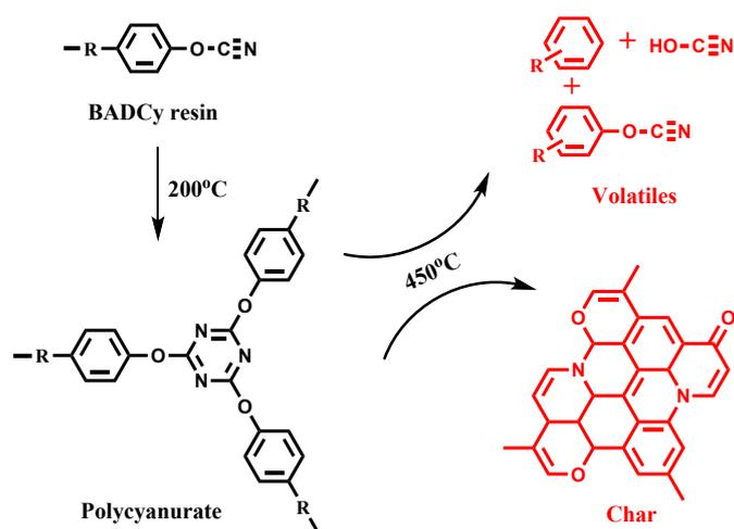
**Scheme S1.** Schematic diagram of polymerization and thermal degradation of BADCy resin
