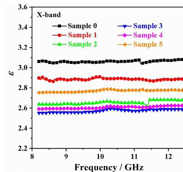
**Figure S3.** The dielectric constant ( $\epsilon$ ) of unmodified BADCy (Sample 0) and *m*-BADCy (Sample 1-5) resins in X-band frequency range (8.2~12.4 GHz).
