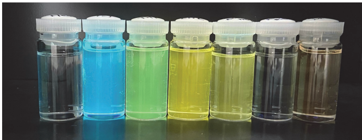
Figure S7. Photograph of TPPhG2B solution under UV irradiation. From left: hexane, toluene, THF, chloroform, acetone, and DMSO.
