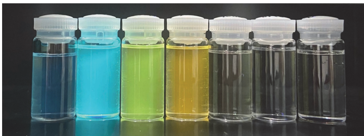
Figure S6. Photograph of AdG2B solution under UV irradiation. From left: hexane, toluene, THF, chloroform, acetone, and DMSO.
