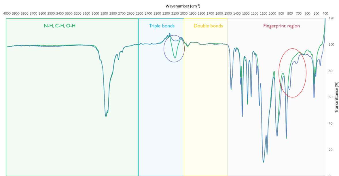
Figure S17. FT-IR spectra of MeO-PEG-OMs (blue, 4 ) vs MeO-PEG-N 3 (green, 5 ). Characteristic stretching of sulphur bonds (with oxygen and carbon in 4 ) and azide (in 5 ) are circled in red and purple, respectively.
