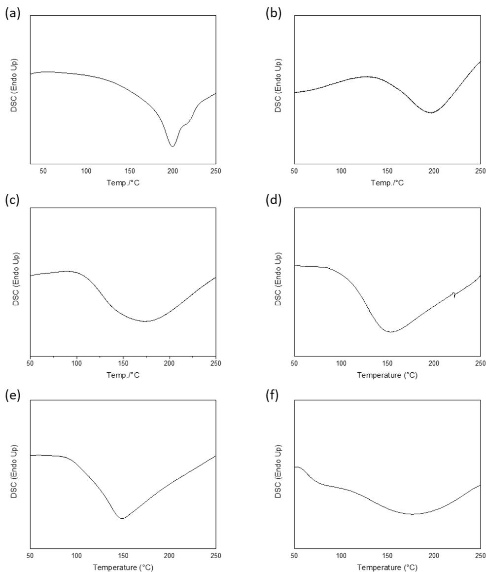
Figure S19 DSC curves of (a) Poly EDY-A; (b) Poly EDY-A<sup>1</sup>; (c) Poly EDY-A<sup>2</sup>; (d) Poly EDY-B; (e) Poly EDY-C; (f) Poly EDY-D under heating rate as 5 K/min
