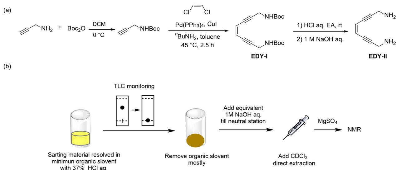
**Figure S1** (a) Synthetic route of di-*tert*-butyl octa-4-en-2,6-diyne-1,8-diyl(*Z*)-dicarbamate **EDY-I** and (*Z*)-octa-4-en-2,6-diyne-1,8-diamine **EDY-II**. (b) Designed procedure of handle with **EDY-II** solution
