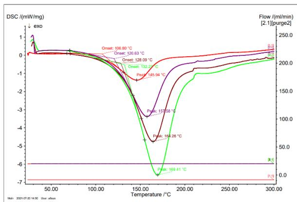
Figure S18 DSC curves of EDY-III under heating rate as 5/10/15/20 K/min
