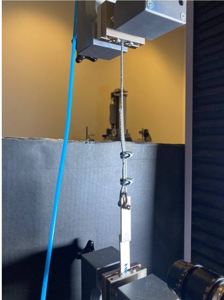
Figure S123 – Homemade setup for the lap-shear tests on prepared specimens.
