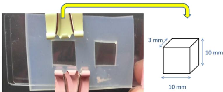
**Figure S3.** Photograph of the mold for gel preparation.
