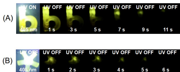
Figure S16. Photographs of (A) spiroBF 2 -PAA-0.125% and (B) fluoreneBF 2 -PAA-0.125% under 405 nm lamp and after removal of lamp.
