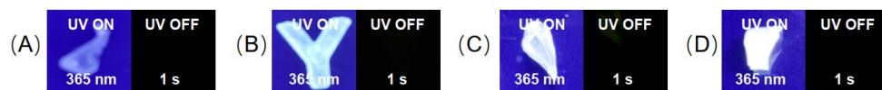
Figure S6. Photographs of PMMA, PAA, PS, PHEMA obtained by photoinitiated bulk polymerization without BF 2 bdk addition under 365 nm UV lamp and after removal of UV lamp.
