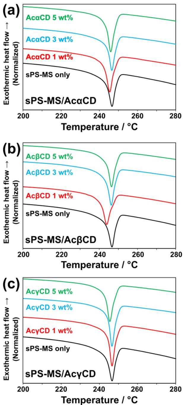
**Fig. S7.** DSC thermograms of the sPS-MS composites under the second scan with (a) Ac $\alpha$ CD, (b) Ac $\beta$ CD, and (c) Ac $\gamma$ CD.
