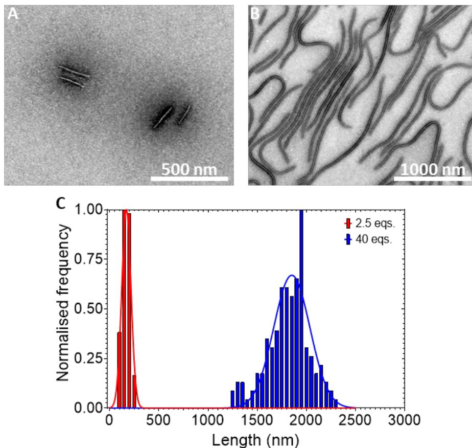
**Figure S11.** TEM micrographs of nanofibers prepared through seeded-growth after 12 months of the addition of unimer in THF to nanofiber seed solutions ( $L_n = 46$  nm,  $D = 1.17$ ,  $\sigma = 19$  nm, in THF:MeOH 15:85 v/v) at: A) 2.5:1  $m_{unimer}/m_{seed}$  ratio ( $L_n = 167$  nm,  $D = 1.05$ ,  $\sigma = 37$  nm), and B) 40:1  $m_{unimer}/m_{seed}$  ratio ( $L_n = 1798$  nm,  $D = 1.02$ ,  $\sigma = 267$  nm). C) Contour length histograms of the nanofibers in A (red) and B (blue).
