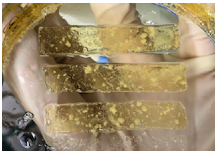
Fig. S7 Appearance of a gel containing 0.50 g/L of C-dots. Preparation condition: [DMAAm unit of \mathbf{D}_{300} ] = 1000 mM, [NIPAAm] = 1000 mM, [BIS] = 20 mM in C-dots dispersion in water (0.50 g/L) at 60 °C for 18 h.
