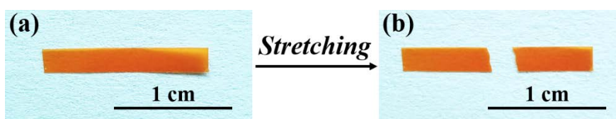
Fig. S10 The photo images of an unstretched PEA-2b film (a) and the resulting broken PEA-2b film upon stretching (b).
