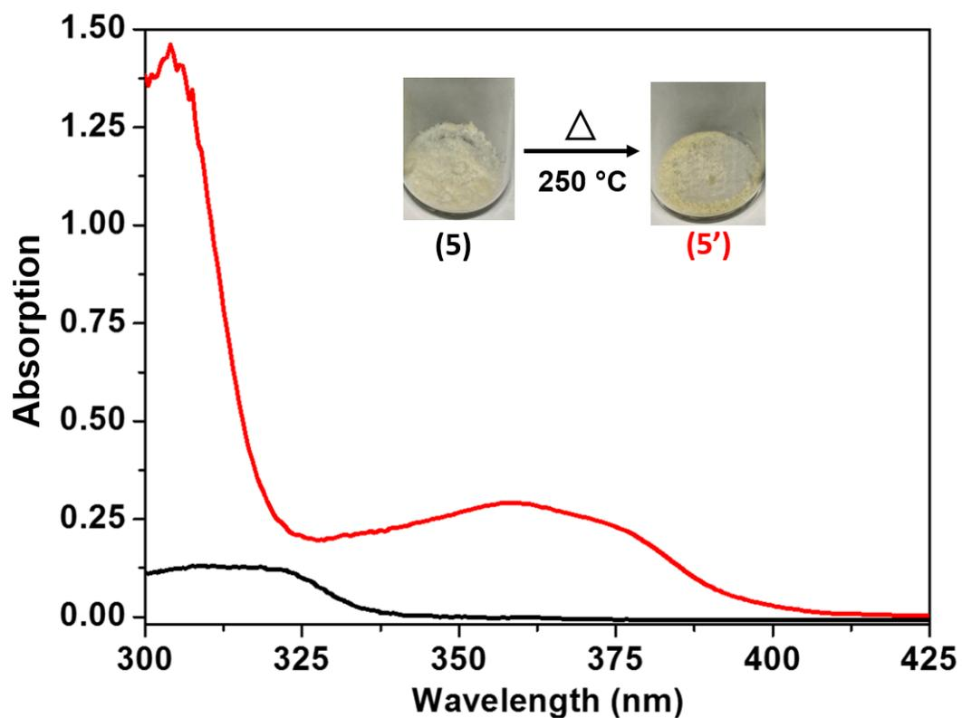
**Fig. S23** UV-Vis absorbance spectra of CO-mechanophore before (5) and after (5') thermal activation.
