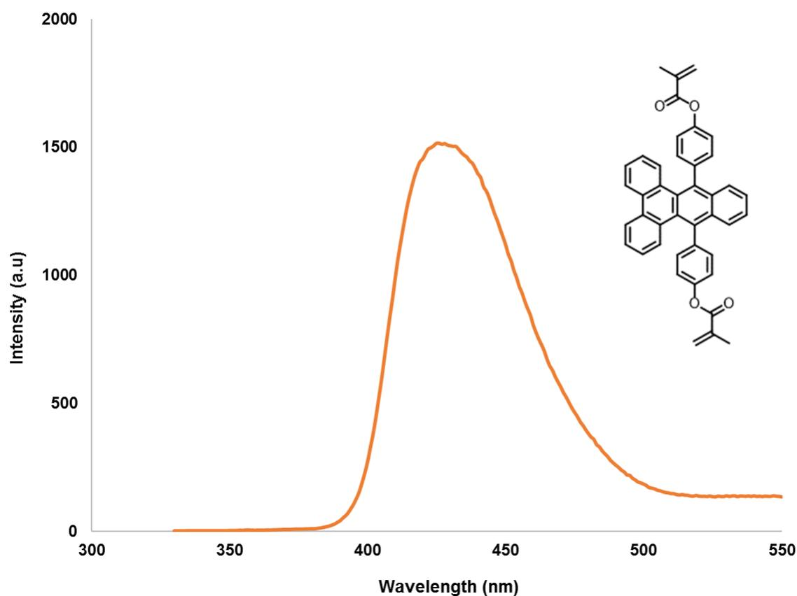
Fig. S24 Fluorescence emission of CO-mechanophore after thermal activation (5') at 330 nm excitation wavelength.
