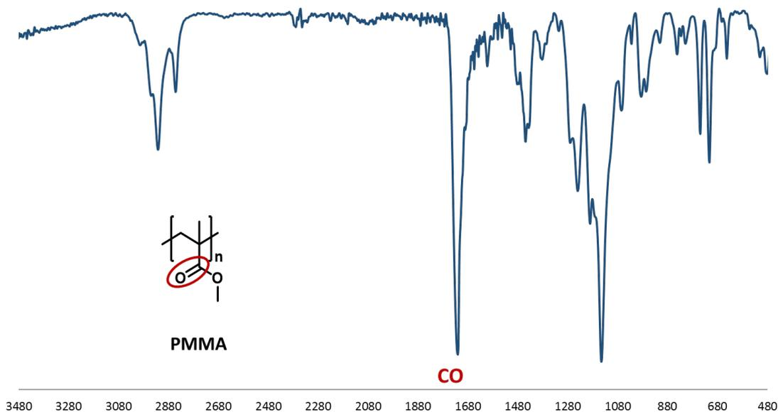
**Fig. S21** IR spectrum of cross-linked PMMA network free of CO-mechanophore molecule.
