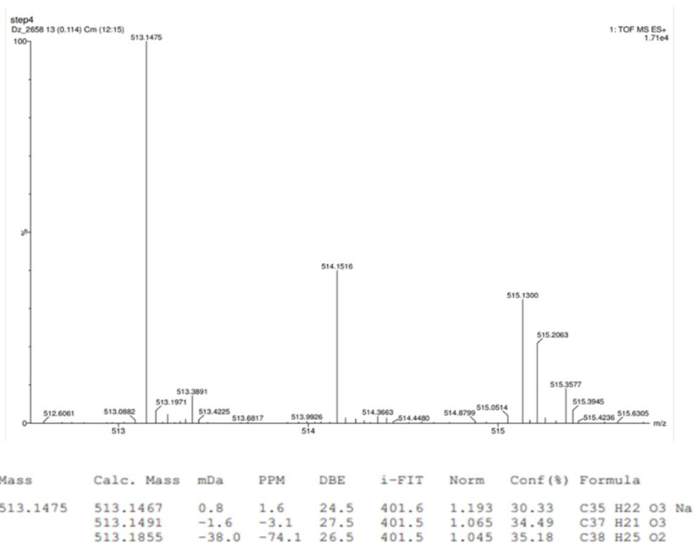
Fig. S18 High-Resolution Mass spectroscopy of diol CO-mechanophore 4.
