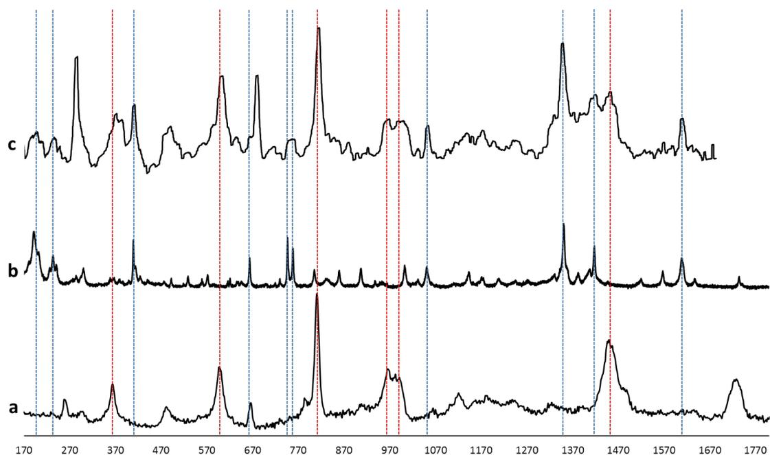
**Fig. S22** Raman spectra of a) pure PMMA b) dimethacrylate CO-mechanophore (5) and c) active network before cryomilling composed of both PMMA peaks (red) and CO-mechanophore peaks (blue).
