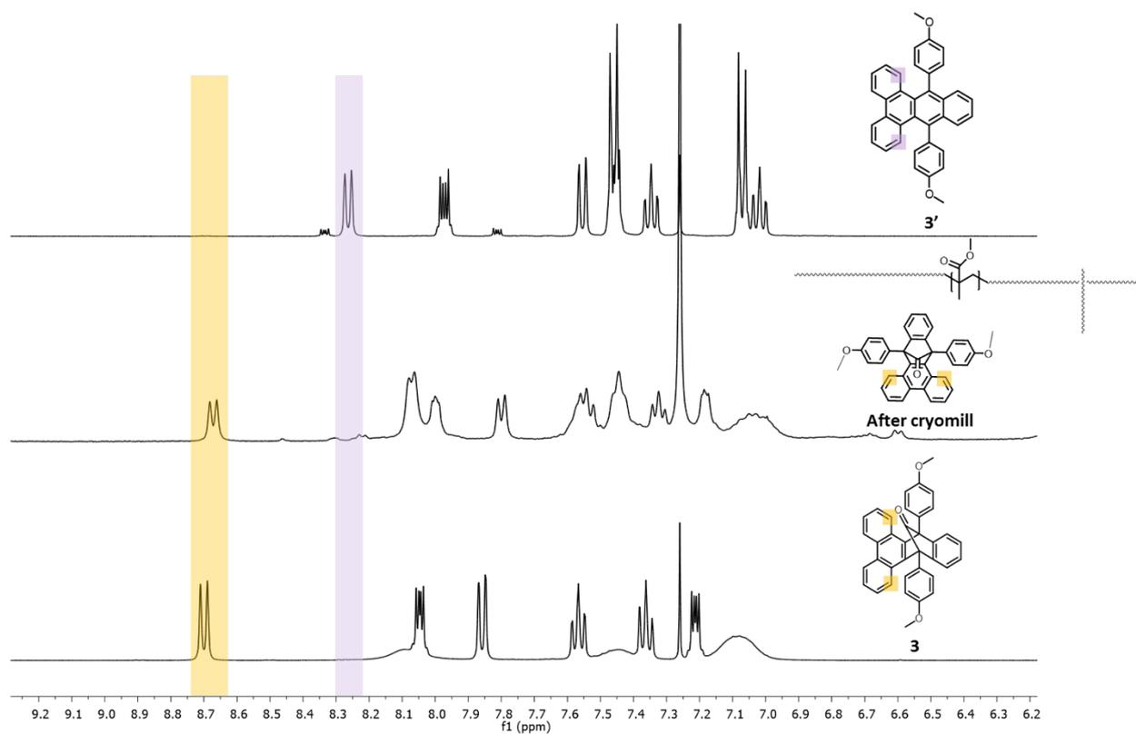
**Fig. S17** <sup>1</sup>H NMR (400 MHz) of control PMMA network (**6**) after cryomilling compared to compounds **3** and **3'**.
