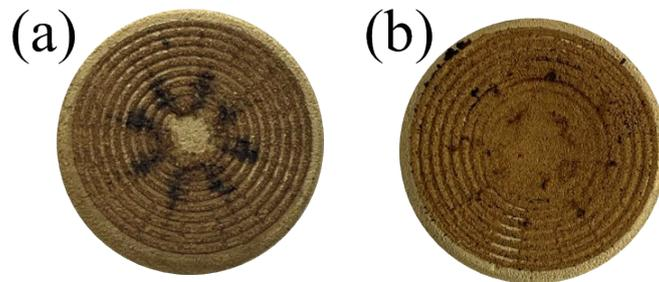
Figure S2. The digital images of CMPs@6 and CMPs@7 after PM filtration for 48 h.
