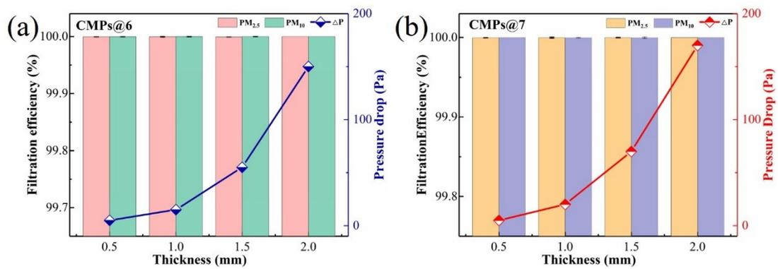
Figure S6. Filtration efficiency and pressure drop for CMPs@6(a) and CMPs@7(b) with different thickness.
