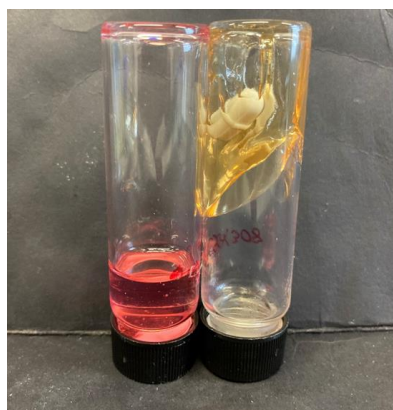
Figure S7. Digital photograph recorded for the original free-flowing 20% w/w dispersion of P(LMA 50 - stat -GlyMA 9 )-PMMA 67 nanoparticles (left-hand vial) and the viscous gel that is obtained after heating the same dispersion to 110 °C for 40 h (right-hand vial).
