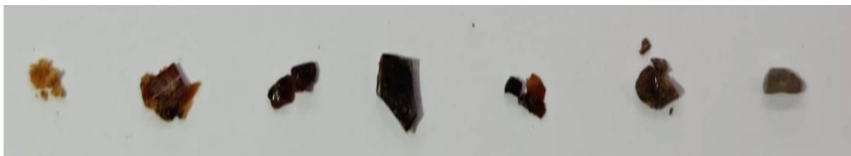
Figure S1: Photo of X-poly(S- r -TVTSi) series ( X = \text{wt\% S} ). From left to right: X = 20, 30, 40, 50, 60, 70 and 80 .
