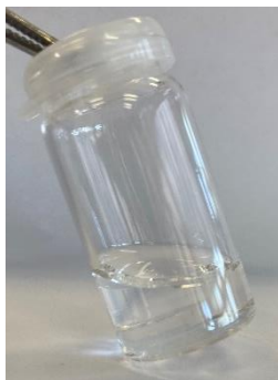
Figure S50: A small PU-disk was cut out and placed in a vial containing 1 mL THF to remove the molecular tag.
