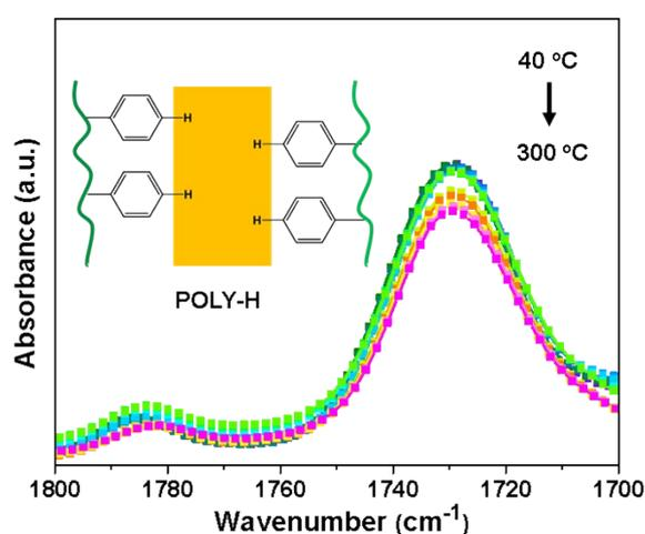
**Figure S2.** Temperature-dependent FTIR spectra of POLY-H upon heating from 40 to 300 °C
