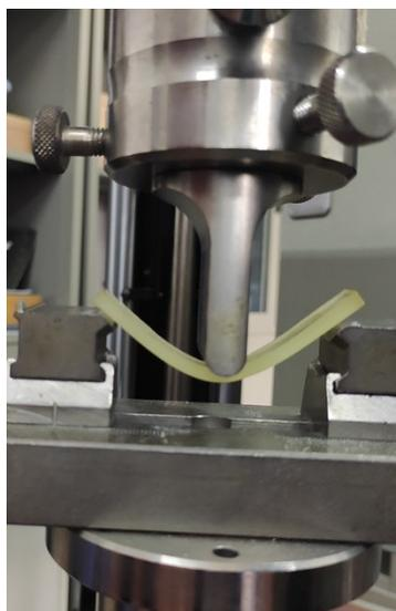
Figure S5. Optical image of the EG-1.2MQ-20% specimen during the flexural test.
