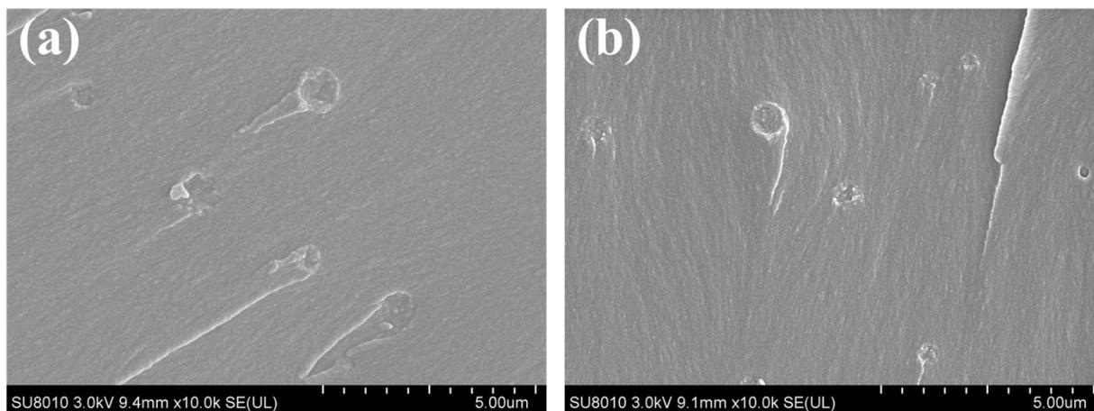
Figure S6. High Resolution SEM images of (a) EG-0.8MQ-20% and (b) EG-1.0MQ-20%.
