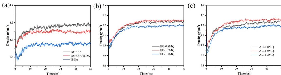
**Figure S3.** Molecular density (a) DGEBA, IPDA and their mixture (b) EG-MQ (c) AG-MQ.
