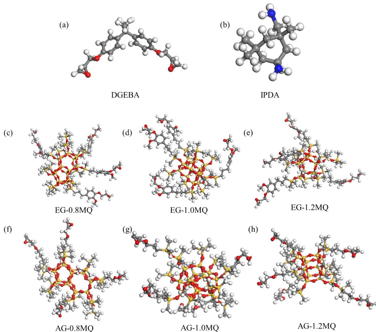
**Figure S2.** Molecular structure of DGEBA, IPDA, and epoxy MQ silicone resins.
