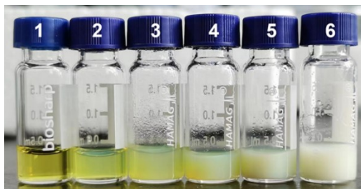
Figure S2 Digital images of the withdrawn samples from the RAFT dispersion polymerization of St mediated by (mPEG750) 3 -CDPA. Polymerization conditions: [St] 0 : [CTA]: [AIBN] = 1200:3:1, 15 wt% solids, MeOH/H 2 O = 4/1 (w/w), 70 °C. 1-6 correspond to 4.25, 8.25, 11.25, 14.25, 16.75, and 19.75 h.
