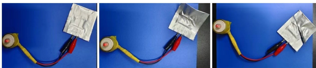
Figure S14. Photographs of the lamps lightened by the flat, folded and cut Li|PUSS 1 PEG 3 |LFP pouch cell.
