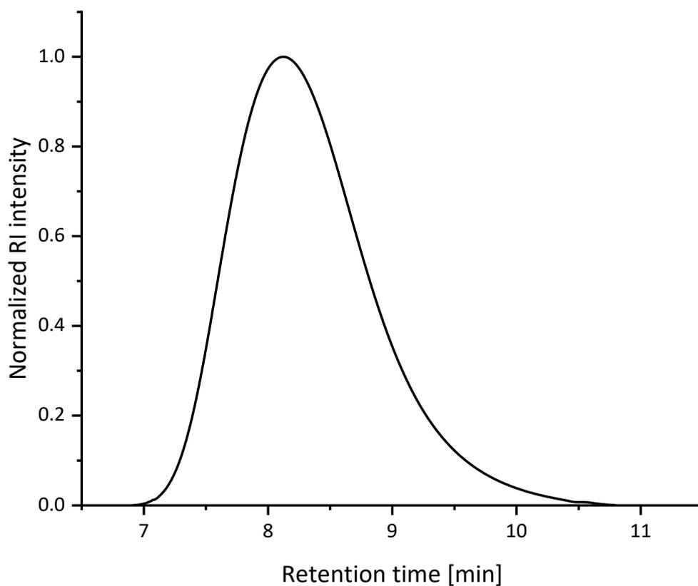
**Figure S9:** SEC-elugram of polymer **P3** (chloroform/isopropanol/triethylamine [94/2/4], PMMA-standard).
