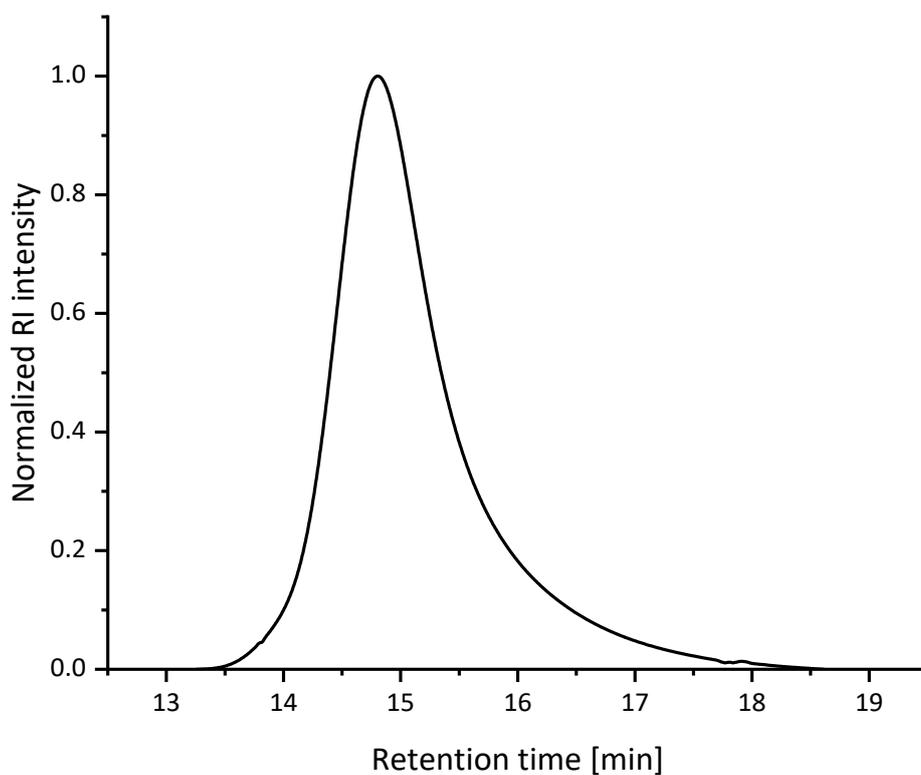
**Figure S8:** SEC-elugram of polymer **P2** (chloroform/isopropanol/triethylamine [94/2/4], PMMA-standard).
