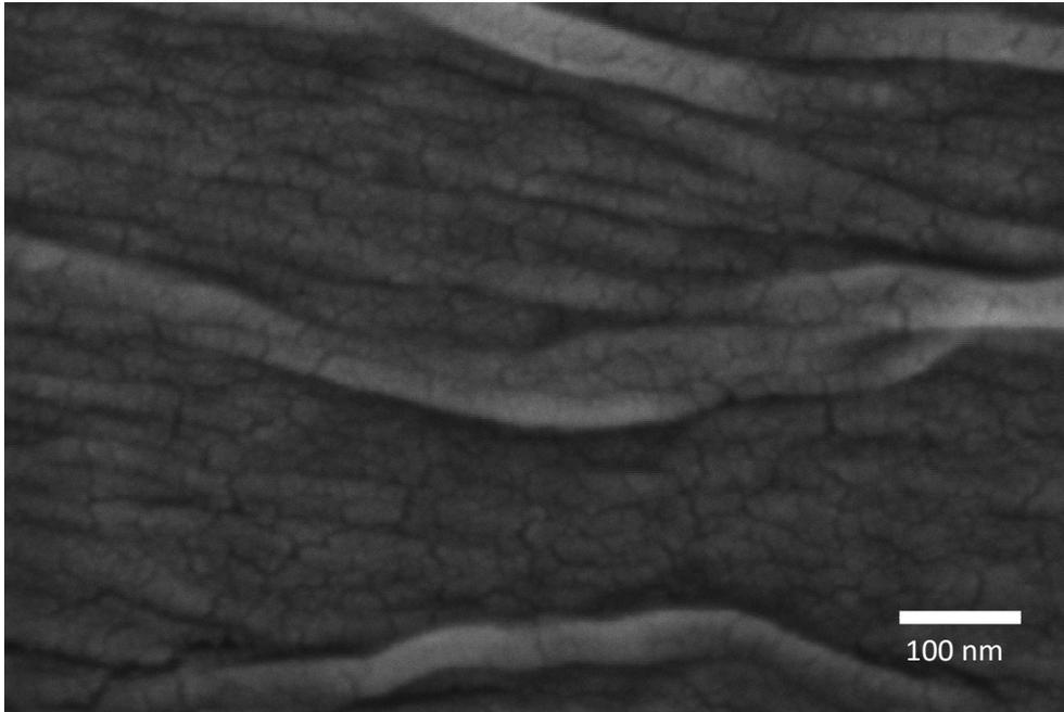
**Figure S3:** SEM-image of a dialysis tubing with a cut-off of 1 kDa freeze dried from water.
