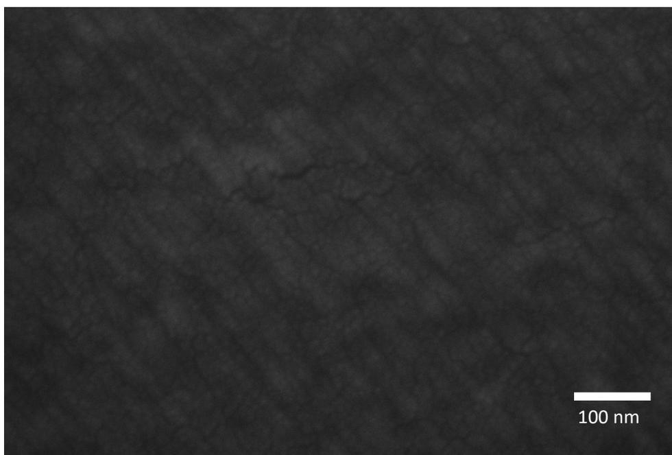
**Figure S6:** SEM-image of a dialysis tubing with a cut-off of 8 kDa freeze dried from chloroform.
