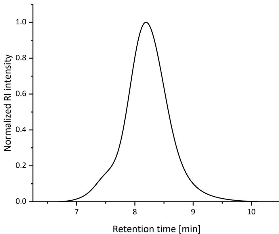
**Figure S11:** SEC-elugram of polymer P5 (chloroform/isopropanol/triethylamine [94/2/4], PMMA-standard).
