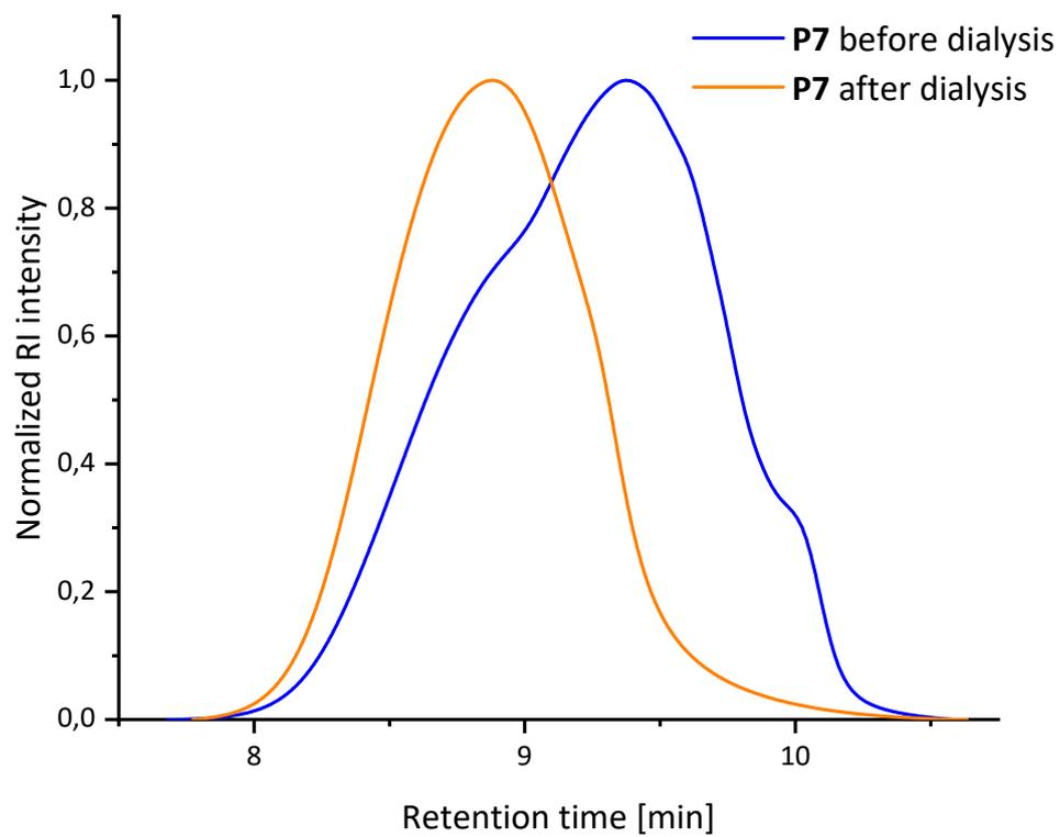
**Figure S13:** SEC-elugrams of Polymer **P7** before (blue) and after (orange) dialysis (chloroform/isopropanol/triethylamine [94/2/4], PMMA-standard).
