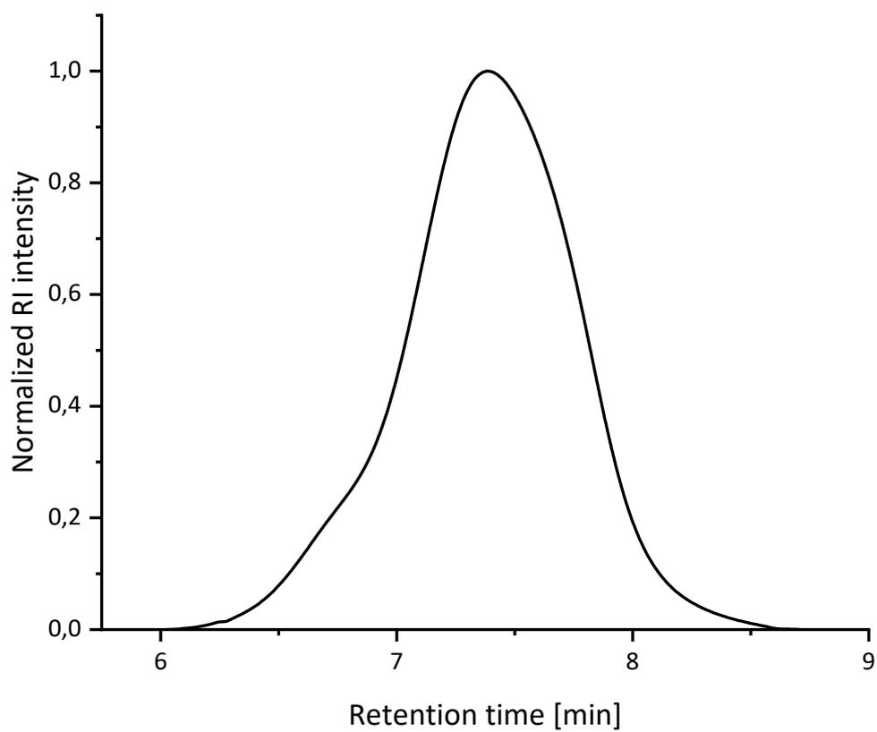
**Figure S12:** SEC-elugram of polymer P6 (chloroform/isopropanol/triethylamine [94/2/4], PMMA-standard).
