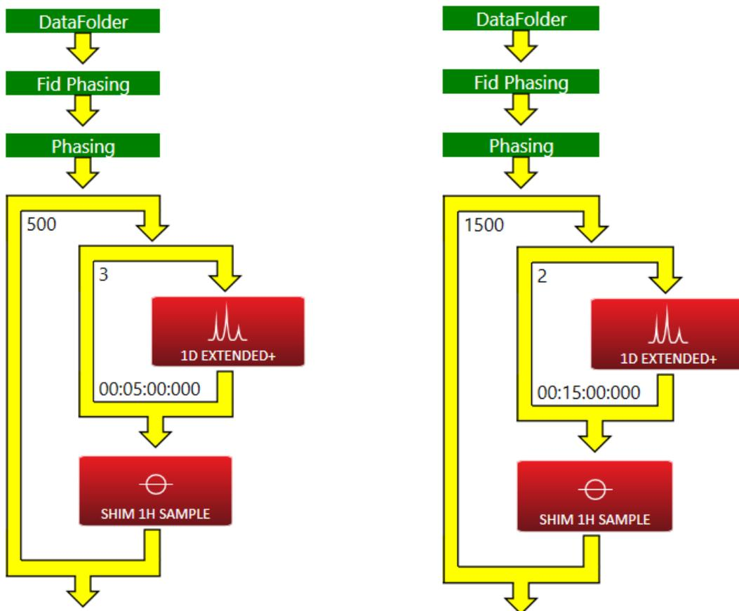
**Figure S1:** Schematic representation of the NMR-measurement-script shown in the Spinsolve software. Left: THF and toluene experiments. Right: Chloroform measurements.
