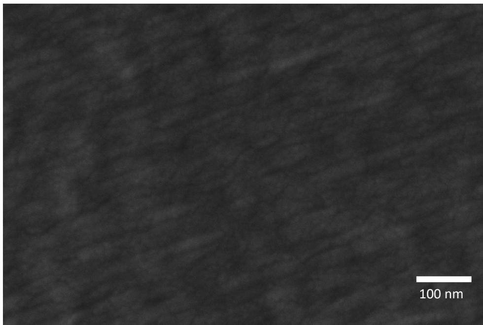
**Figure S5:** SEM-image of a dialysis tubing with a cut-off of 1 kDa freeze dried from chloroform.
