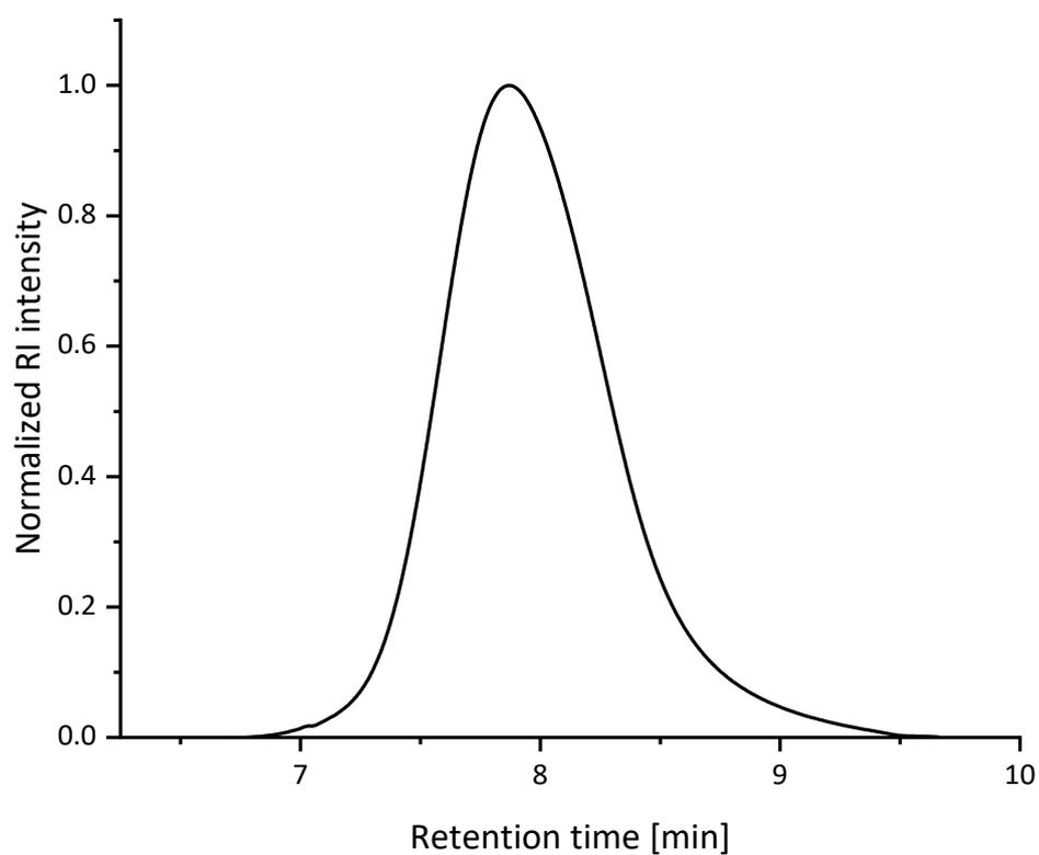
**Figure S7:** SEC-elugram of polymer **P1** (chloroform/isopropanol/triethylamine [94/2/4], PMMA-standard).
