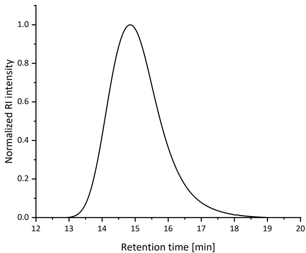
**Figure S10:** SEC-elugram of polymer **P4** (chloroform/isopropanol/triethylamine [94/2/4], PMMA-standard).
