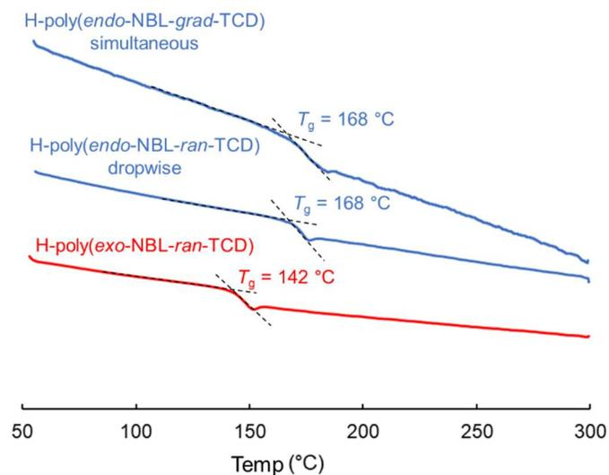
**Figure S8.** DSC curves and  $T_g$  values of H-poly(*endo*-NBL-*grad*-TCD) (entry 1 in Table S2), H-poly(*endo*-NBL-*ran*-TCD) (entry 2 in Table S2), and H-poly(*exo*-NBL-*ran*-TCD) (entry 4 in Table S2).
