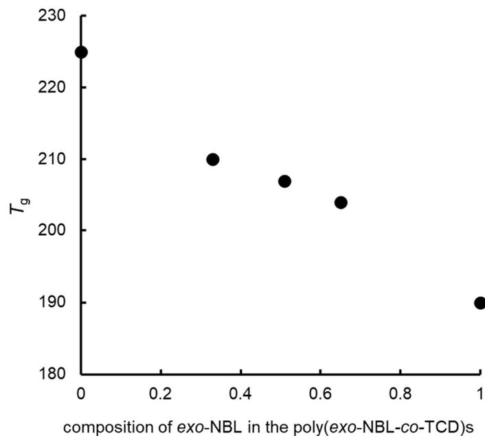
Figure S4.  $T_g$  values of poly(*exo*-NBL-*co*-TCD)s at various compositions of *exo*-NBL unit.
