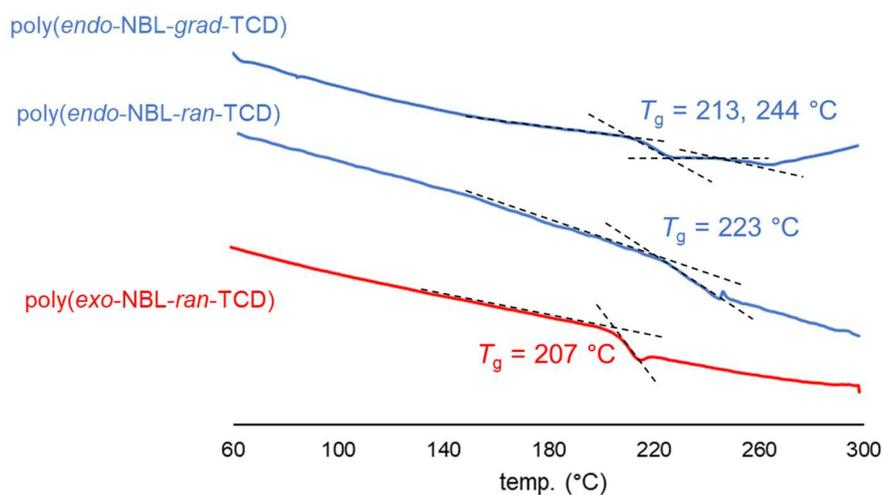
**Figure S7.** DSC curves and  $T_g$  values of poly(*endo*-NBL-*grad*-TCD) (entry 1 in Table 2), poly(*endo*-NBL-*ran*-TCD) (entry 2 in Table 2) and poly(*exo*-NBL-*ran*-TCD) (entry 4 in Table 2).
