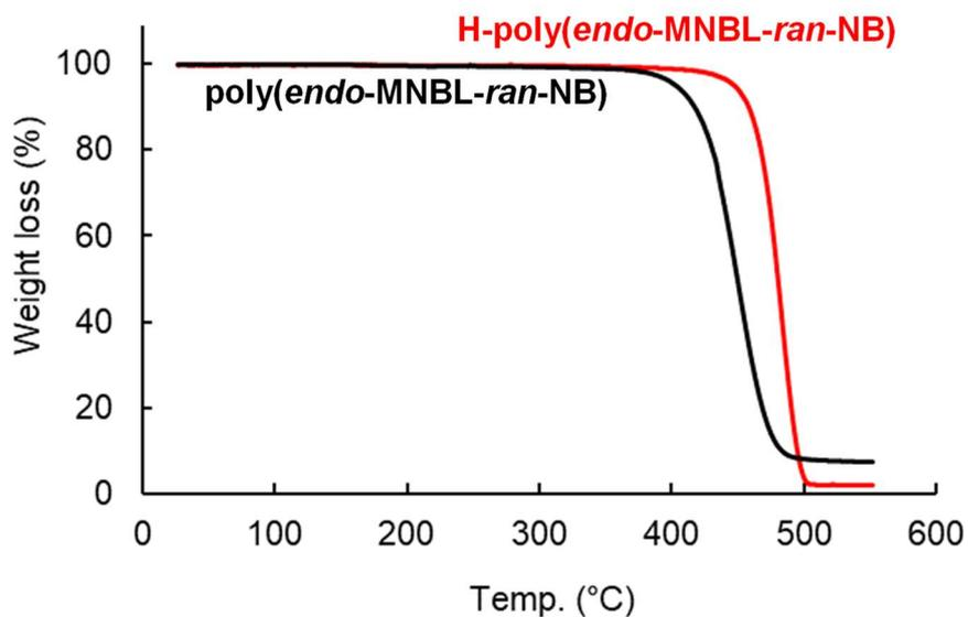
Figure S15. TGA curves of poly(*endo*-MNBL-*ran*-NB) and H-poly(*endo*-MNBL-*ran*-NB) (*endo*-MNBL /NB = 52/48)
