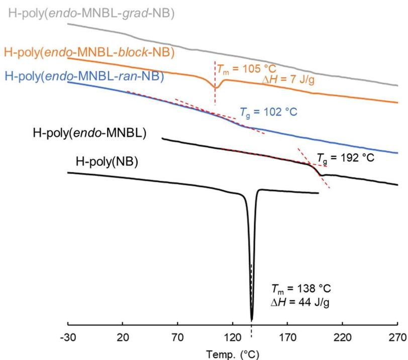
Figure S11. DSC curves and  $T_g$  values of H-poly(*endo*-MNBL-*co*-NB)s compared with the corresponding homopolymers.
