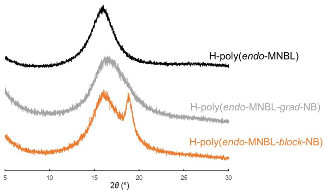
Figure S19. XRD patterns of H-poly(*endo*-MNBL) and H-poly(MNBL-*co*-NB)s with heat hysteresis (annealed at 200 °C for 30 min).
