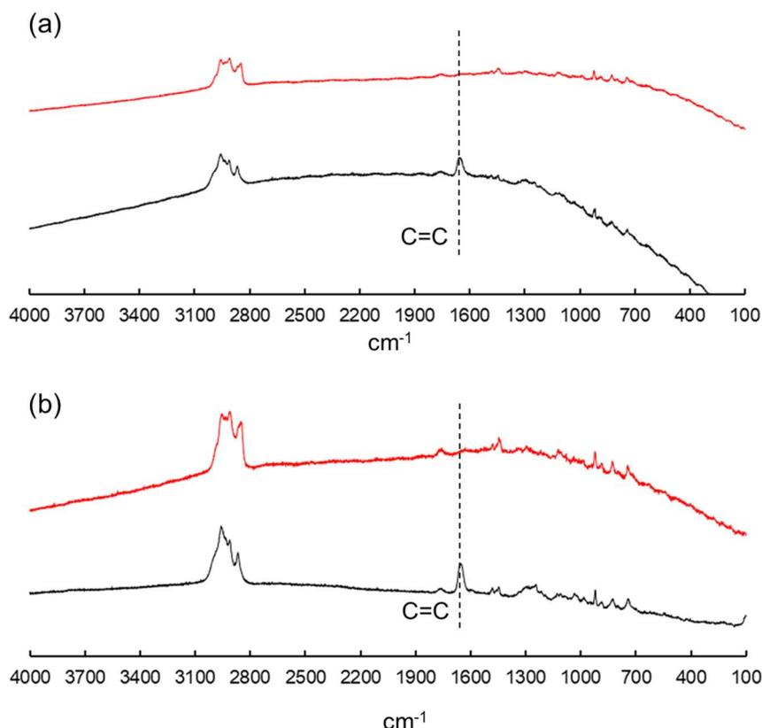
**Figure S3.** Raman spectra of before (black) and after (red) the hydrogenation of (a) poly(*endo*-NBL-grad-TCD) (entry 1, Table 2) and (b) poly(*endo*-NBL-ran-TCD) (entry 2, Table 2).
