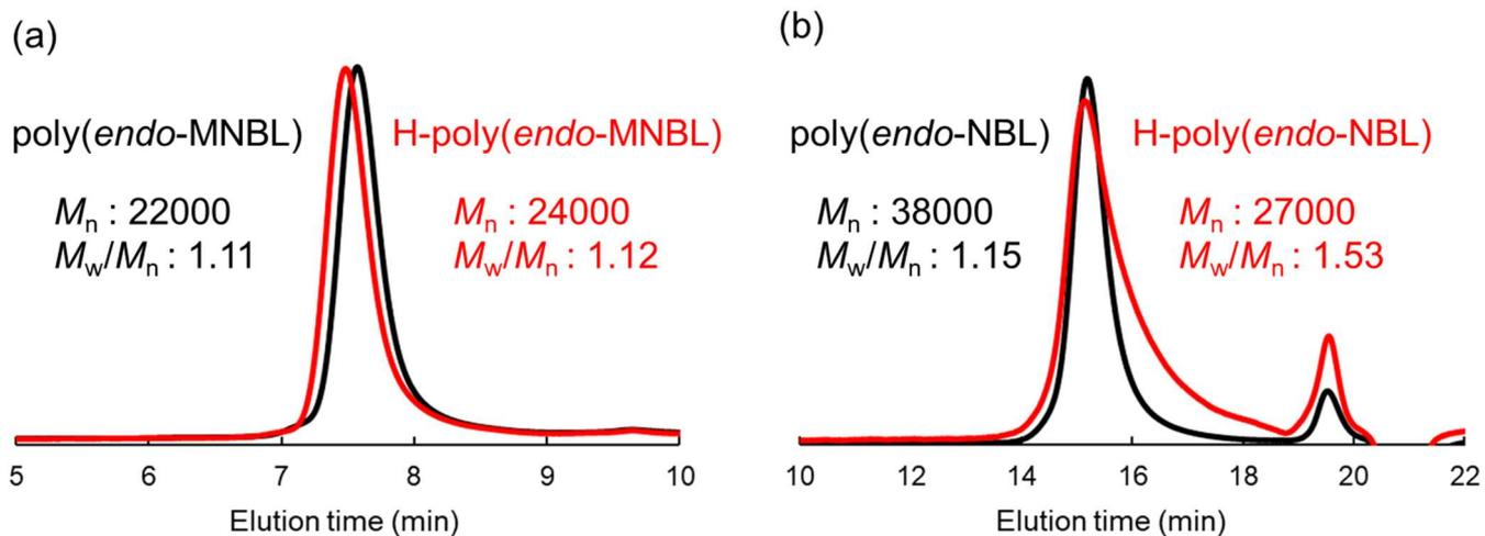
**Figure S2.** SEC profiles of before and after the hydrogenation of (a) poly(*endo*-MNBL) ( $\text{CHCl}_3$  as the eluent) and (b) poly(*endo*-NBL) (DMF as the eluent).
