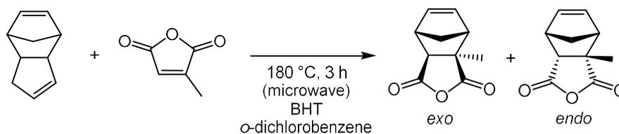
Dicyclopentadiene (2.96 g, 22.4 mmol), citraconic anhydride (5.24 g, 46.8 mmol) and a trace amount of 3,5-di-*tert*-butyl-4-hydroxytoluene (BHT) were dissolved in *o*-dichlorobenzene (5.0 mL). The solution was stirred under microwave irradiation at 180 °C for 3 h. After the volatiles were evaporated under vacuum and subsequent sublimation, the mixture of *endo/exo*-2-methyl-5-norbornene-2,3-
