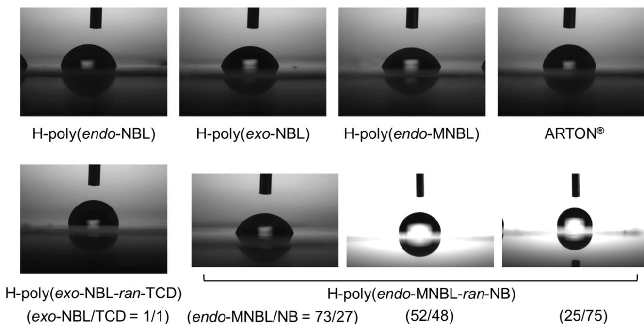
**Figure S21. Pictures of water contact angle measurement.**
