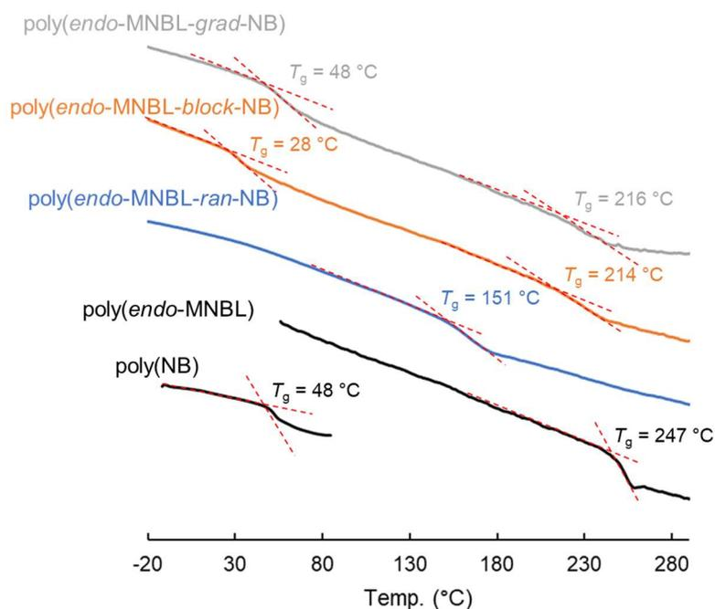
**Figure S9.** DSC curves and  $T_g$  values of poly(*endo*-MNBL-*co*-NB)s compared with the corresponding homopolymers.
