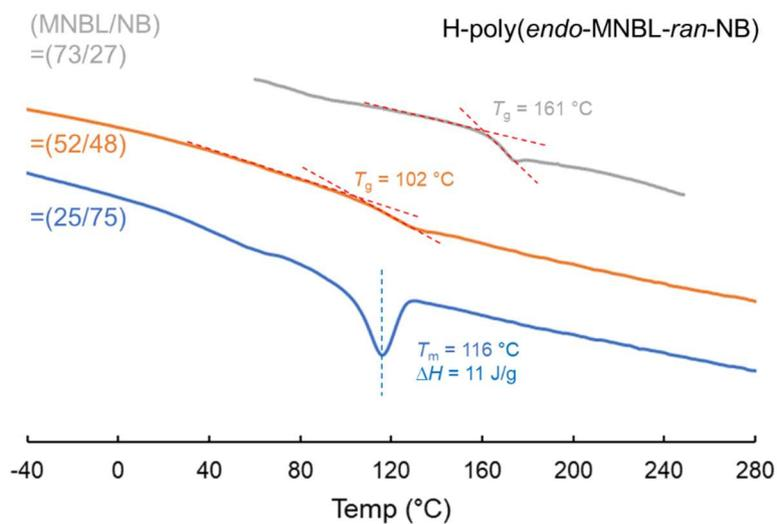
Figure S12. DSC curves and  $T_g$  values of H-poly(*endo*-MNBL-*ran*-NB)s with various compositions.
