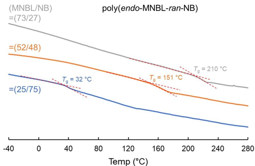
Figure S10. DSC curves and  $T_g$  values of poly(*endo*-MNBL-*ran*-NB)s with various compositions.
