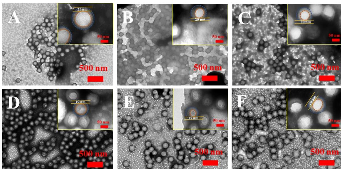
**Fig. S13** TEM images of nanoparticles. (A) – (C): BA/MMA=1/3, 1/1, 3/1, macro-initisurf =40%, reaction temperature=90 °C, solid content=40%; (D) – (F): BA/MMA=1/3, 1/1, 3/1, macro-initisurf =40%, reaction temperature=90 °C, solid content=50%.
