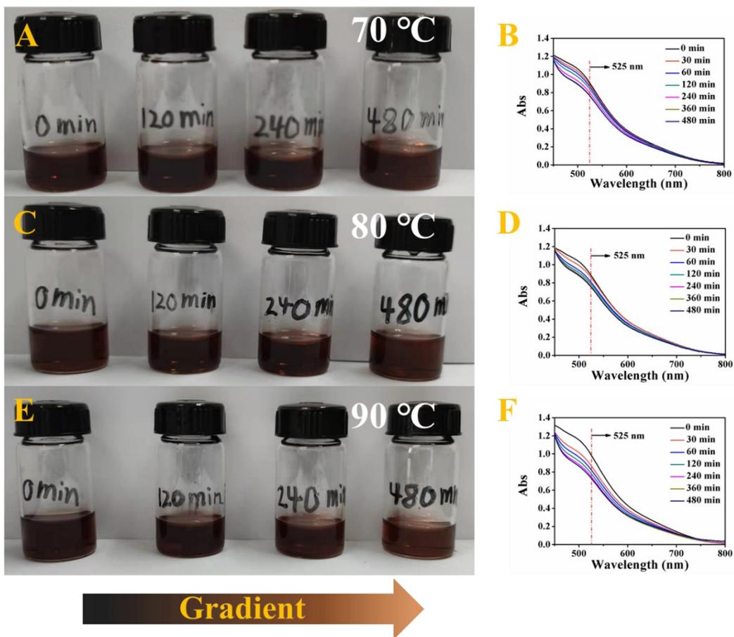
**Fig. S5** The photos of mixture of MAA-*alt*-AMS and DPPH in DMSO at different temperatures, (A) 70 °C, (C) 80 °C and (E) 90 °C , and their corresponding UV-vis absorption spectra, (B) 70 °C, (D) 80 °C and (F) 90 °C.
