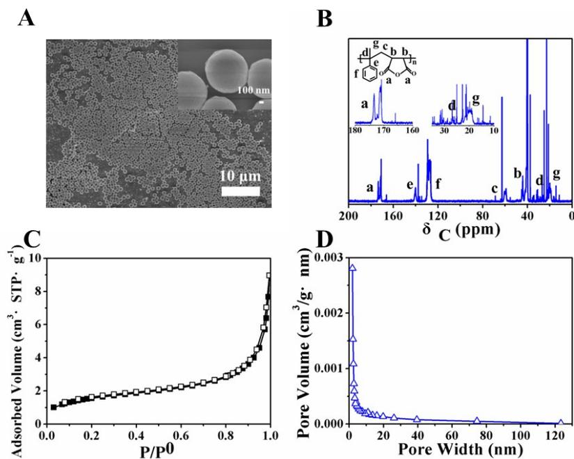
**Fig. S1** (A) SEM images of MAH-*alt*-AMS microspheres, (B)  $^{13}\text{C}$  NMR spectra of MAH-*alt*-AMS microspheres, (C)  $\text{N}_2$  adsorption isotherms and (D) the pore size distribution of MAH-*alt*-AMS microspheres.
