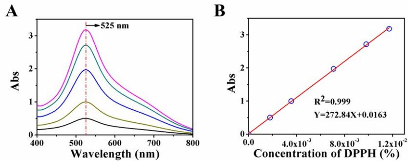
**Fig. S4** (A) UV-vis absorption spectrum of DPPH-DMSO, and (B) the relation curve that absorbance at 525 nm varies with DPPH concentration.
