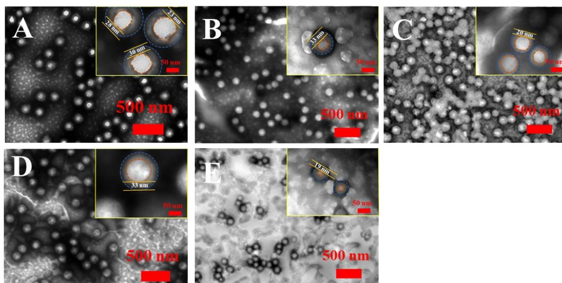
**Fig. S12** TEM images of nanoparticles. (A) – (C): BA/MMA=1/3, 1/1, 3/1, macro-initisurf=40%, reaction temperature=80 °C; (D) – (E): BA/MMA=1/3, 1/1, macro-initisurf=40%, reaction temperature=70 °C.
