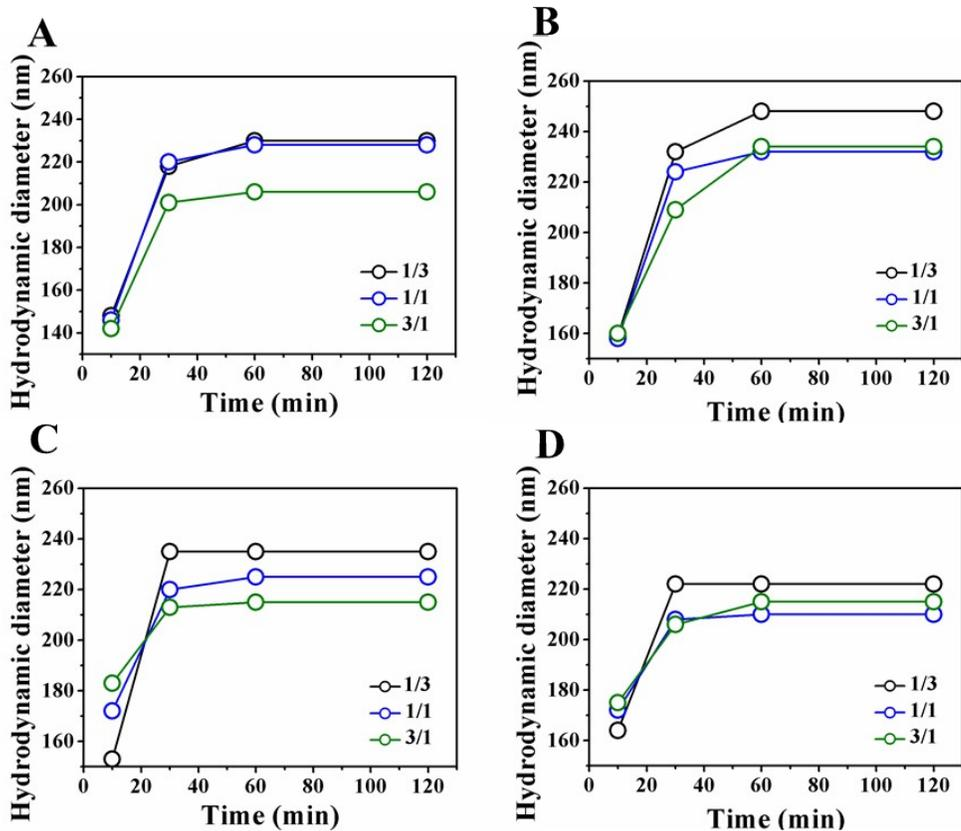
**Fig. S8** Evolution of nanoparticles size during emulsion PISA initiated by different amount of macro-initisurf. Macro-initisurf / monomers = 10%, w/w. (A), 20% (B), 30% (C) and 40% (D).
