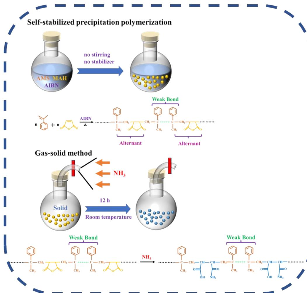
**Scheme S1.** Schematic illustration of the macro-initisurf prepared by AMS, MAH and  $\text{NH}_3$ .
