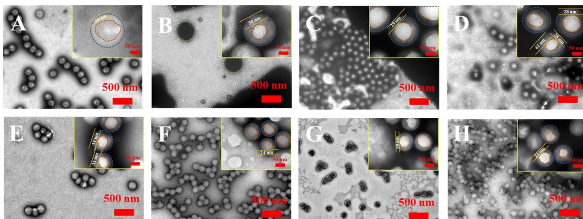
**Fig. S11** TEM images of nanoparticles, reaction temperature=90 °C. (A), (B): BA/MMA=1/2, 2/1, macro-initisurf content=10%; (C), (D): BA/MMA=1/2, 2/1, macro-initisurf content=20%; (E), (F): BA/MMA=1/2, 2/1, macro-initisurf content=30%; (G), (H): BA/MMA=1/2, 2/1, macro-initisurf content=40%
