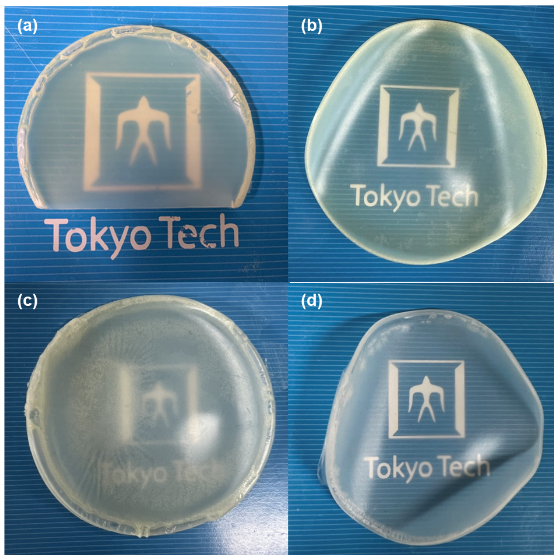
Fig. S6 PU films formed by solvent casting: (a) PDCPU20; (b) PDCPU30; (c) PDCPU50; (d) EGPU20.
