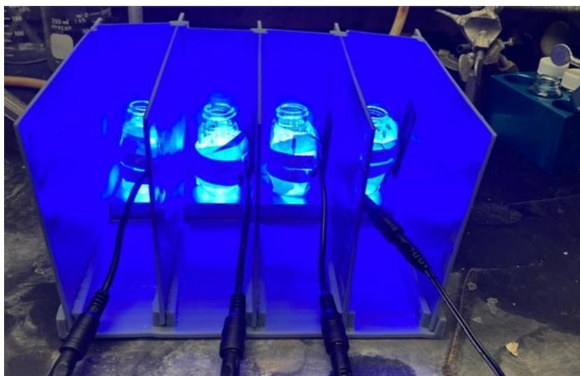
**Figure S1:** Photograph of the photoreactor used for the kinetic studies (without the reaction vials).
