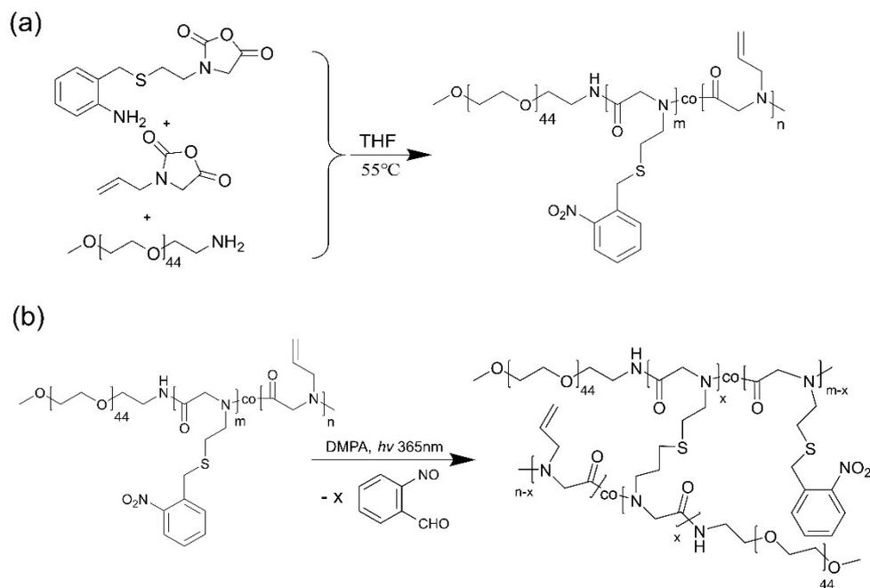
**Scheme S3.** Synthetic pathway of the self-crosslinking nanogels from photoresponsive polypeptoid copolymers.
