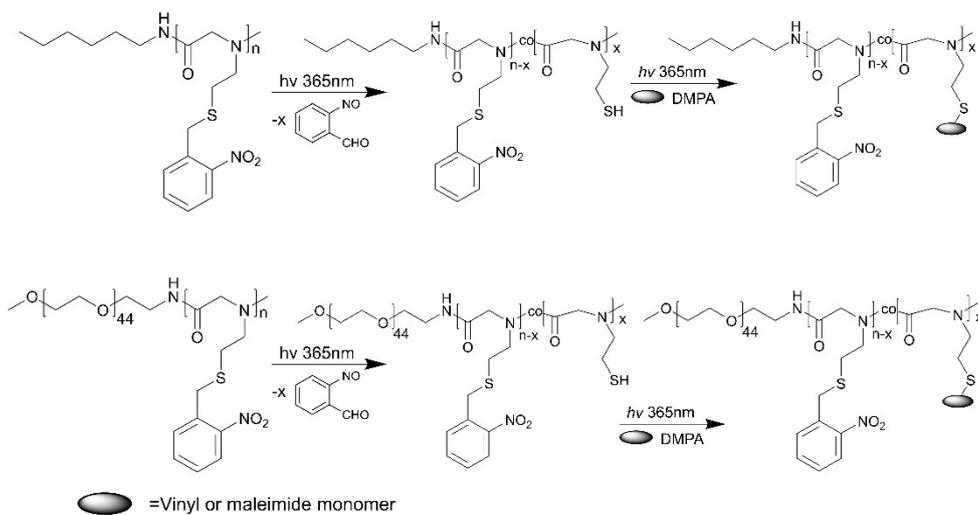
**Scheme S4.** Synthetic route of the side chain modification of photoresponsive polypeptoid copolymers.
