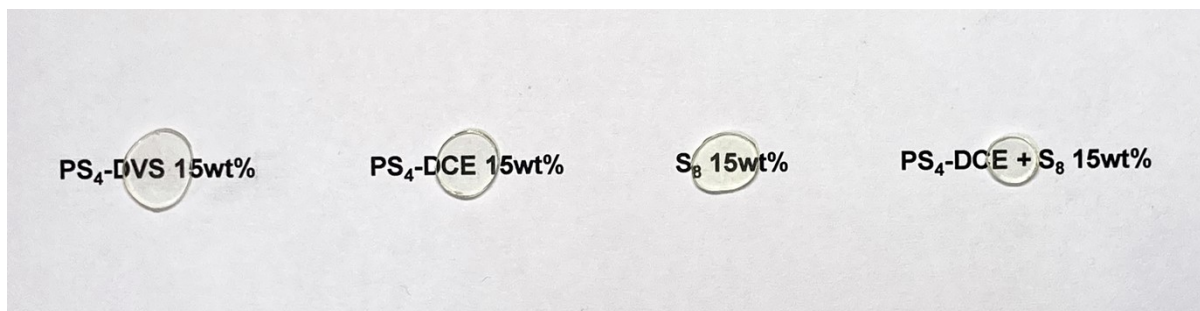
Figure S4. Digital image of films (thickness = 1 mm) of p(PS-BEPS) and p(S-BEPS) obtained from polysulfide polymers, elemental sulfur, and a combination of PS 4 -DCE and elemental sulfur.
