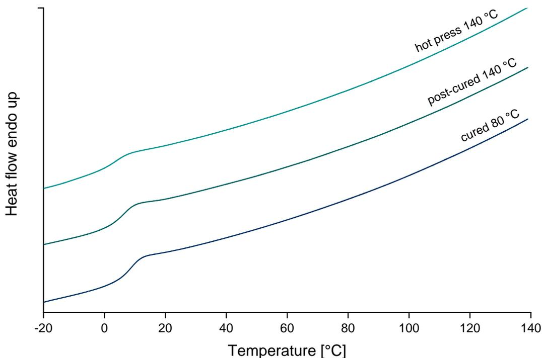
**Figure S43.** DSC curves of 3<sup>rd</sup> heat run (heating rate of 40 °C/min) of **poly4** after curing at 80 °C, post-curing at 140 °C and hot press experiment at 140 °C
