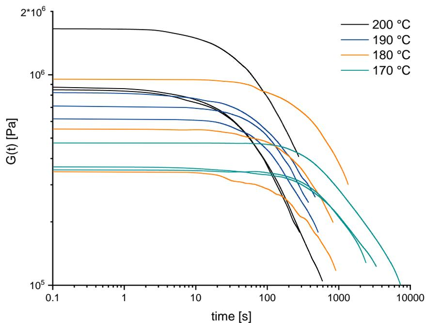
**Figure S46.** Non-normalized stress relaxation experiment at 170, 180, 190, and 200 °C in triple determination; parallel plate setup  $\phi = 8$  mm; preset  $F_n = 1$  N; strain = 1%.
