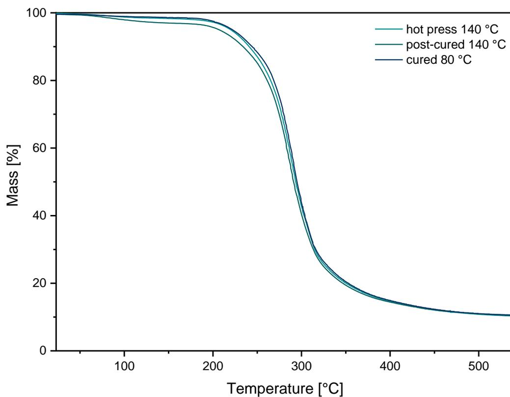
**Figure S42.** Thermogravimetric analysis of **poly4** after curing at 80 °C, post-curing at 140 °C and hot press experiment at 140 °C.
