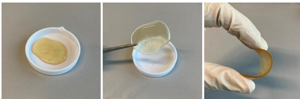
**Figure S37.** Pictures of **poly4** after curing at 80 °C.
