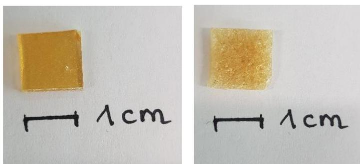
**Figure S39.** Pictures of **poly4** before and after immersion in methylene chloride for 22 h.
