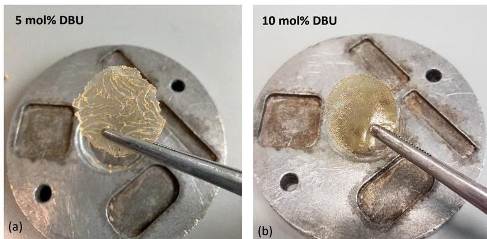
**Figure S44.** Pictures of **poly4** prepared with (a) 5 mol% DBU vs (b) 10 mol% DBU after hot press (1 h, 140 °C, 50 bar).
