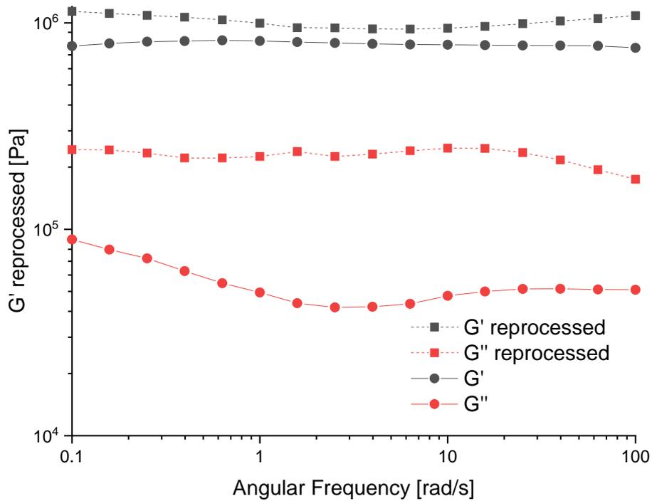
**Figure S48.** Frequency sweep at 180 °C showing storage ( $G'$ ) and loss modulus ( $G''$ ) of the sample before and after reprocessing at 180 °C in a range of 0.1-100 rad/s.
