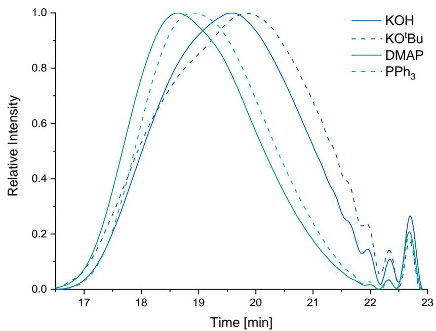
**Figure S24:** SEC of **poly1** including bases (KOH or KO<sup>t</sup>Bu) or nucleophiles (PPh<sub>3</sub> or DMAP) after 1 month.
