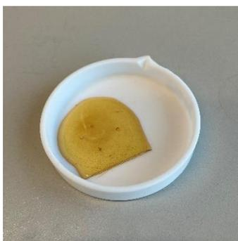
**Figure S38.** Pictures of **poly4** after curing at 140 °C.
