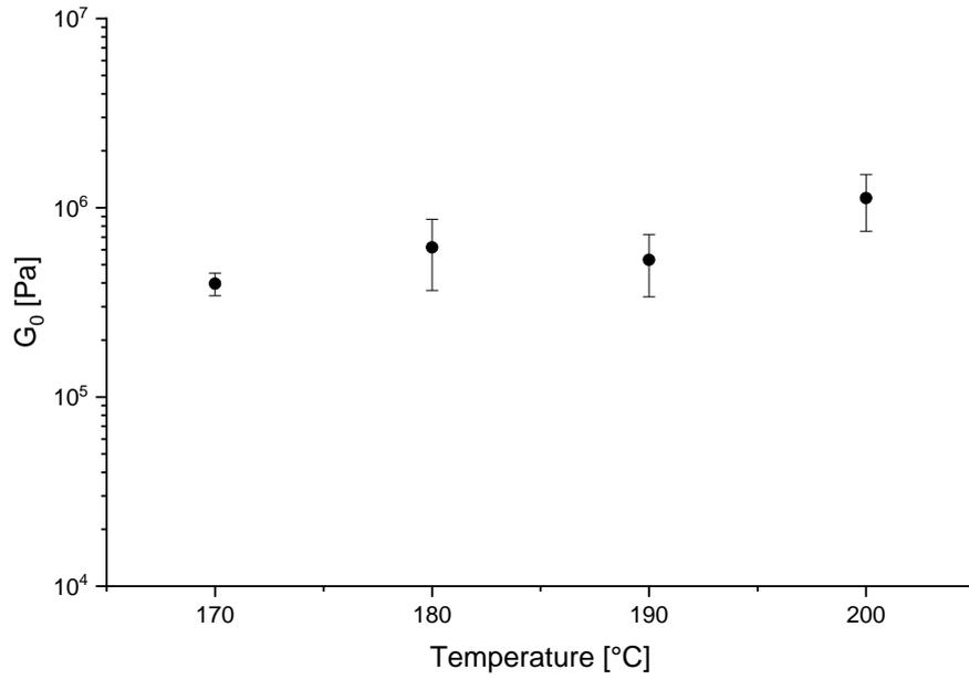
**Figure S47.** Temperature dependence of initial stress relaxation modulus  $G_0$  at  $t = 0.1$  s; parallel plate setup  $\phi = 8$  mm; preset  $F_n = 1$  N; strain = 1%.
